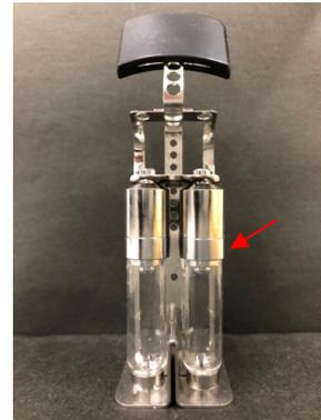
**Fig. S1a.** Pictures of Mettler-Toledo DP 70 Drop Point system for  $T_{\text{drop}}$  measurements. (a1) System overview. (a2) A sample cup, where a hole is made in the bottom. Left: side view, right: top view. (a3) An adapter to hold the sample cup. The red arrow indicates the position where the cup is placed.
