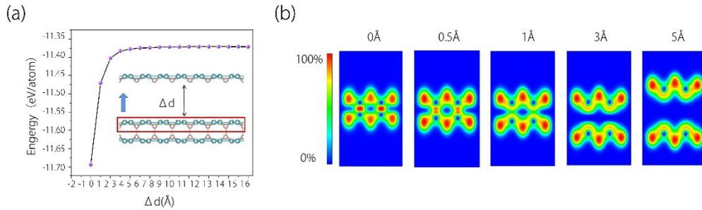
Fig.S2 (a) Curve of interlayer interaction as a function of  $\Delta d$ . (b) 2D slice of local charge density of (-110) plane at different interlayer distances.
