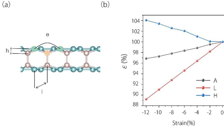
Fig.S3 (a) Side views of BL- $\alpha$  borophene.  $\theta$ ,  $l$  and  $h$  are respectively B<sub>2</sub>-B<sub>1</sub>-B<sub>2</sub> bond angle, B<sub>1</sub>-B<sub>2</sub> bond length and buckling height. (b) Change trend of L, H and A with strain.  $\theta_0$  and  $l_0$ ,  $h_0$  are the bond angle, bond length and buckling height under no strain, respectively.  $A = \theta / \theta_0$ ,  $L = l / l_0$ ,  $H = h / h_0$ .
