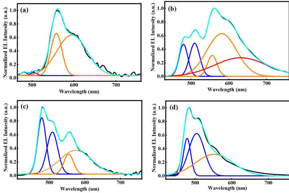
**Figure S4.** The EL spectra and fitting of peaks of the pristine device tested at (a) 4 V and (b) 12 V when annealed temperature was 60 °C. The EL spectra and fitting of peaks of the optimized device tested at (c) 4 V and (d) 12 V when annealed temperature was 60 °C.
