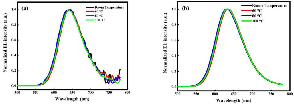
**Figure S2.** The EL spectra of Rubrene at (a) 4 V and (b) 12 V when annealed at different temperatures.
