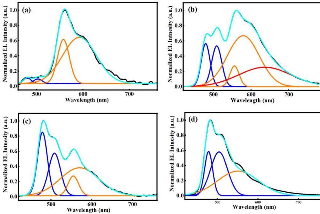
**Figure S5.** The EL spectra and fitting of peaks of the pristine device tested at (a) 4 V and (b) 12 V when annealed temperature was 100 °C. The EL spectra and fitting of peaks of the optimized device tested at (c) 4 V and (d) 12 V when annealed temperature was 100 °C.
