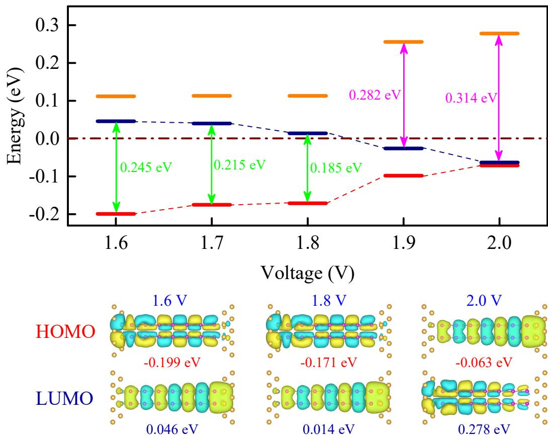
**Fig. S17** The energy of molecular states close to the  $E_f$  as a function of bias near the NDR in  $(\text{SiC})_{13}^{D2-3}$ . The value of HLG is labeled. The spatial distributions of HOMO and LUMO are shown below.
