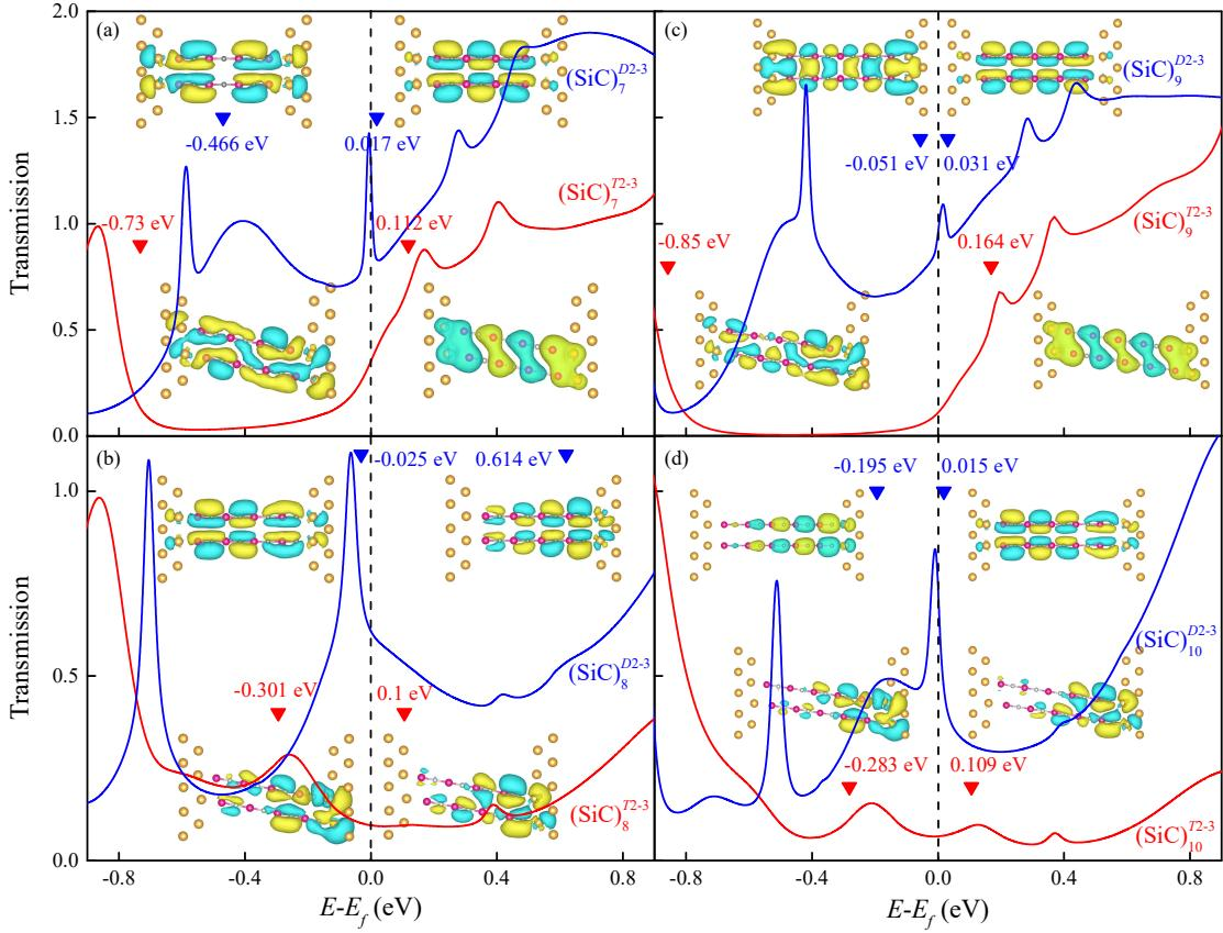
**Fig. S4** The transmission spectra  $T(E,V)$  of  $(\text{SiC})_n^{T2-3}$  and  $(\text{SiC})_n^{D2-3}$  ( $n=7-10$ ) as a function of the electron energy at zero bias. The triangles denote eigenvalues of the MPSH states of HOMO and LUMO. Their spatial distributions are displayed nearby. The isovalue is set to be 0.03.
