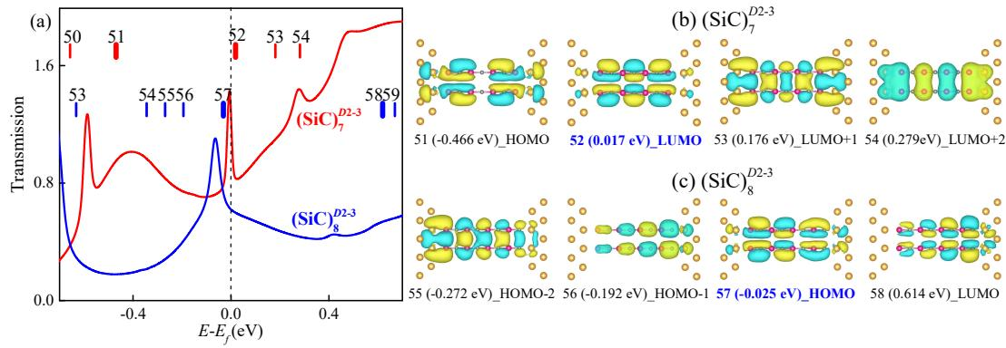
**Fig. S11** (a) The transmission spectra  $T(E,V)$  of  $(\text{SiC})_n^{D2-3}$  ( $n=7, 8$ ) as a function of electron energy at zero bias. The short lines denote eigenvalues of the MPSH states, where the thick ones stand for HOMO and LUMO, respectively. (b-c) The spatial distribution of four MPSH states of  $(\text{SiC})_n^{D2-3}$  ( $n=7, 8$ ) close to the  $E_f$ . The molecular orbital lies closest to the  $E_f$  is highlighted in blue. The isovalue is set to be 0.03.
