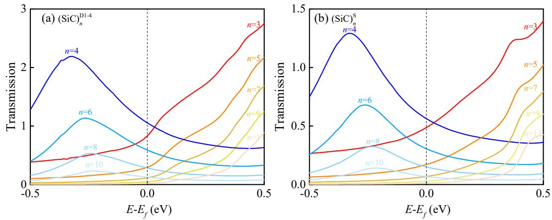
**Fig. S12** (a-b) The transmission spectra  $T(E, V)$  of  $(\text{SiC})_n^{D1-4}$  and  $(\text{SiC})_n^S$  ( $n=3-11$ ) as a function of electron energy at zero bias, respectively.
