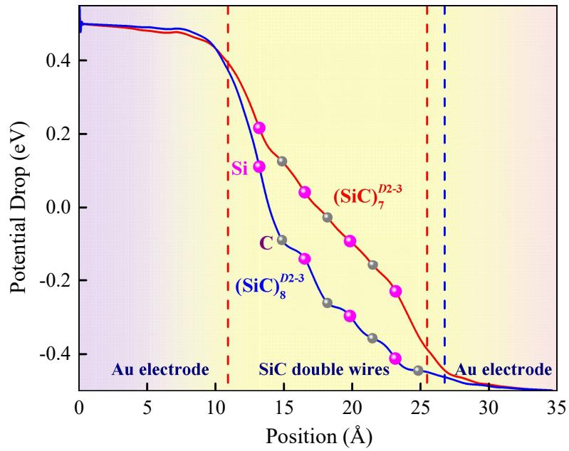
**Fig. S16** The potential drop along the length of  $(\text{SiC})_n^{D2-3}$  ( $n=7,8$ ) at 1.0 V. The red and blue dashed lines indicate the positions of the tip Au atoms in  $(\text{SiC})_n^{D2-3}$  ( $n=7,8$ ), respectively. The small circles represent the positions of the atoms in the chains, and the atomic symbols are given nearby.
