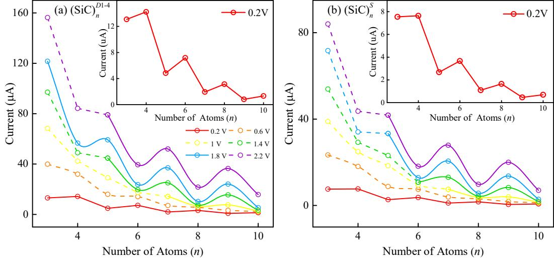
**Fig. S14** The current of  $(\text{SiC})_n^{D1-4}$  and  $(\text{SiC})_n^S$  ( $n=3-10$ ) as a function of number of atoms  $n$ . The partial disturbance of the current oscillation is given by dashed lines. The insets are the occasional current oscillation at 0.2 V.
