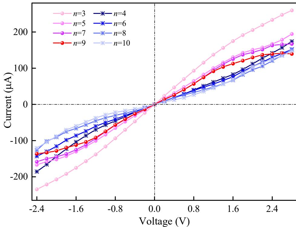
**Fig. S13** The current of  $(\text{SiC})_n^{D2-3}$  ( $n=3-10$ ) as a function of bias in the range of -2.4 to 2.8 V.
