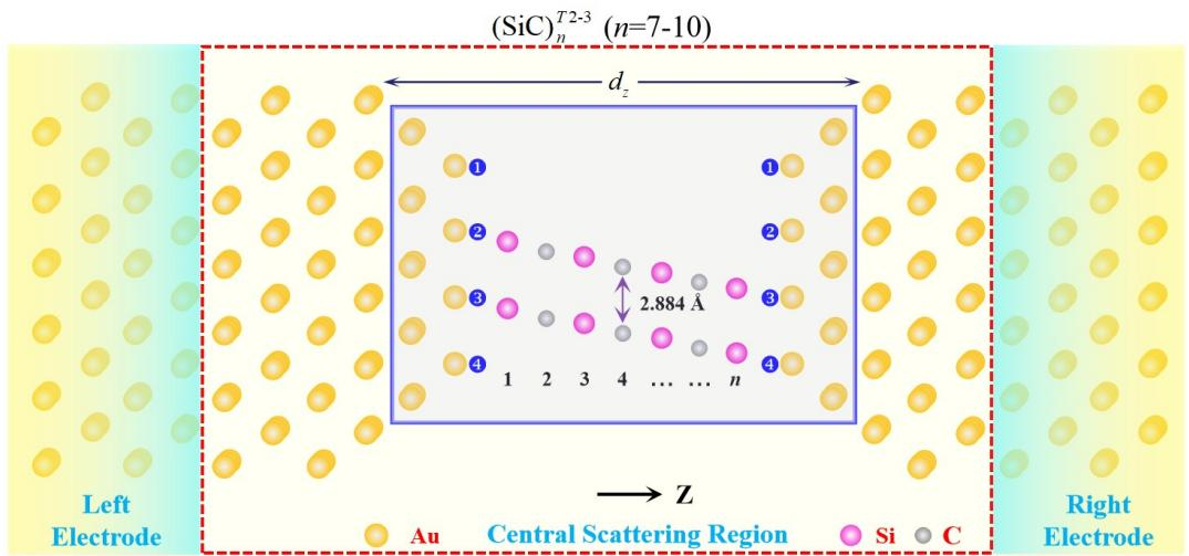
**Fig. S1.** The structure of  $(\text{SiC})_n^{T2-3}$  ( $n=7-10$ ) with double inclined SiC chains, which take sites 2 and 3 on the left electrode, 3 and 4 on the right electrode, to bridge the two semi-infinite Au (100)-3×6 electrodes.
