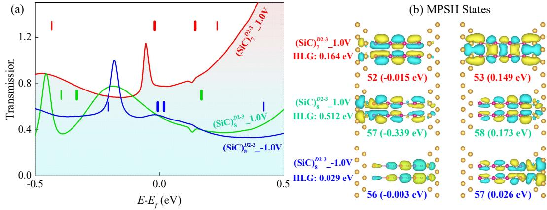
**Fig. S15** (a) The transmission spectra  $T(E,V)$  of  $(\text{SiC})_n^{D2-3}$  ( $n=7, 8$ ) under the typical biases of  $\pm 1.0$  V. The shaded area stands for the transmission integral within the bias window. The short lines denote eigenvalues of the MPSH states, where the thick ones stand for HOMO and LUMO, respectively. (b) The spatial distribution of HOMO and LUMO of  $(\text{SiC})_n^{D2-3}$  ( $n=7, 8$ ) at  $\pm 1.0$  V. The isovalue is set to be 0.03.
