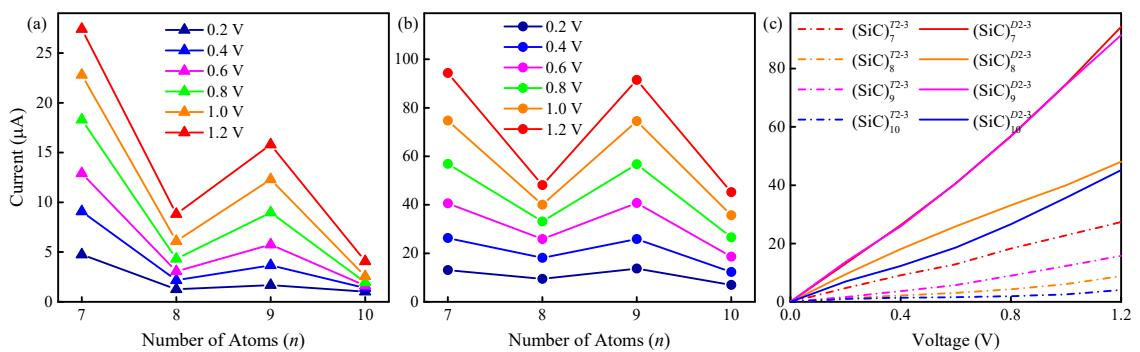
**Fig. S5** The current of (a)  $(\text{SiC})_n^{T2-3}$  and (b)  $(\text{SiC})_n^{D2-3}$  ( $n=7-10$ ) as a function of the number of atoms  $n$ . (c): The current as a function of bias in the range of 0 to 1.2 V.
