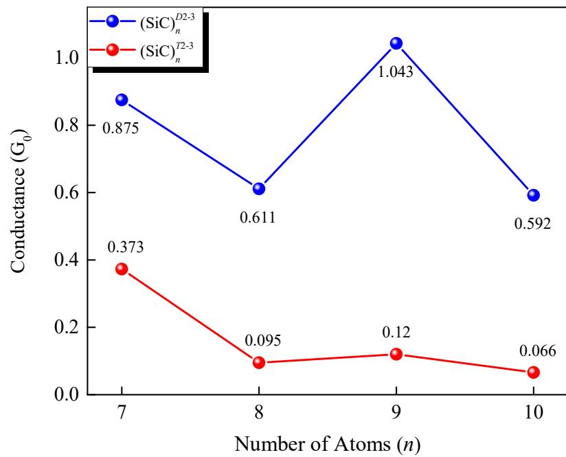
**Fig. S3** The conductance of  $(\text{SiC})_n^{\text{T2-3}}$  and  $(\text{SiC})_n^{\text{D2-3}}$  ( $n=7-10$ ) as a function of the number of atoms  $n$  in the chains.
