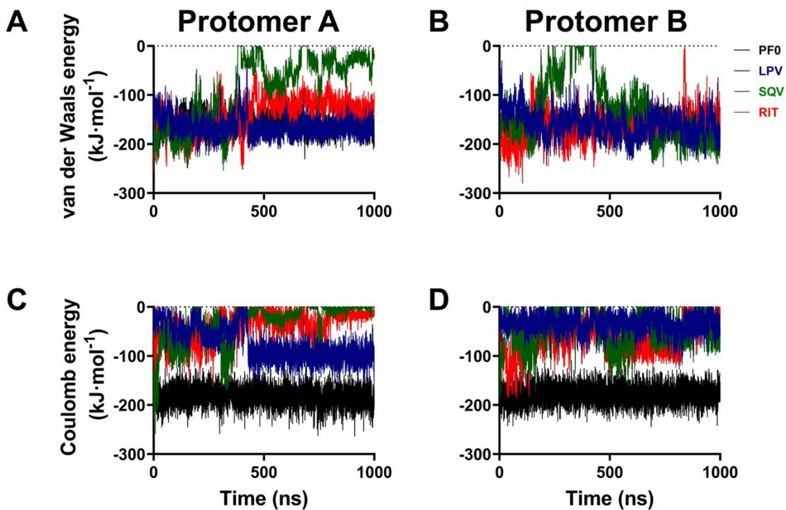
**S3 Fig. The non-bonded interaction energy between the inhibitors and the protomers.** A and B. The van der Waals energy between the four inhibitors and the two protomers, respectively. C and D. The coulomb energy between the four inhibitors and the two protomers, respectively.
