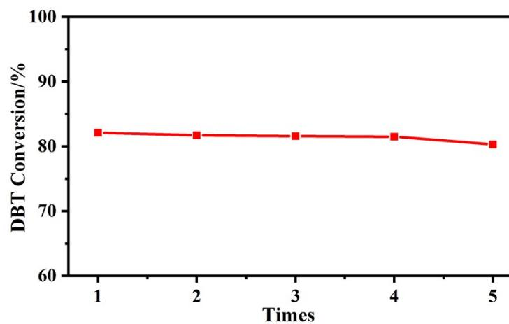
**Fig. S5** Catalytic stability of crystalline Co<sub>4</sub>Mo<sub>12</sub> sulfided at 400 °C.
