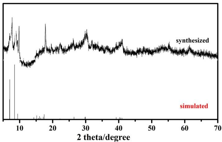
**Fig. S4** The synthesized and simulated powder X-ray diffraction patterns of Co<sub>4</sub>Mo<sub>12</sub>
