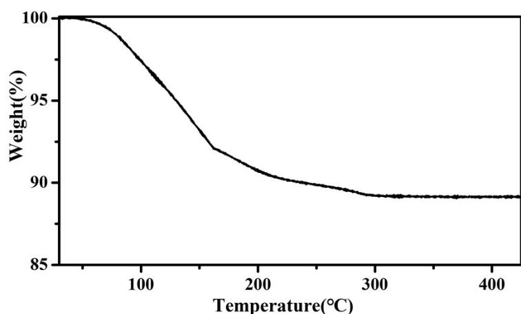
**Fig. S2** TGA of the synthesized Co4Mo12
