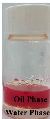
Fig S10. The digital photographs of two-phase systems composed of an aqueous phase and an oil phase containing CdSe 550 /5CdS/2ZnS before reaction (left) and after reaction (right).
