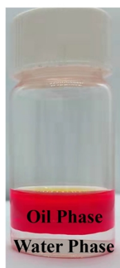
Fig S10. The digital photographs of two-phase systems composed of an aqueous phase and an oil phase containing CdSe 550 /5CdS/2ZnS before reaction (left) and after reaction (right).
