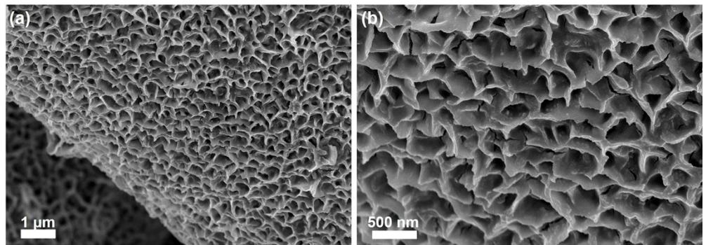
**Fig. S16.** SEM images of NiCo-S electrode after electrolysis.
