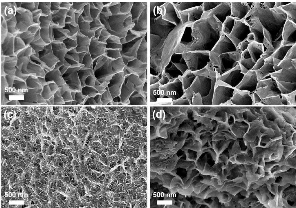
**Fig. S1.** SEM images of (a) NiCo-MOF, (b) NiCo-O, (c) Ni-S, and (d) Co-S samples.
