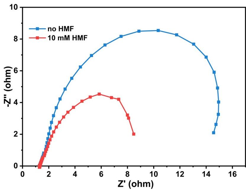
**Fig. S14.** EIS of NiCo-S electrode with or without 10 mM HMF.
