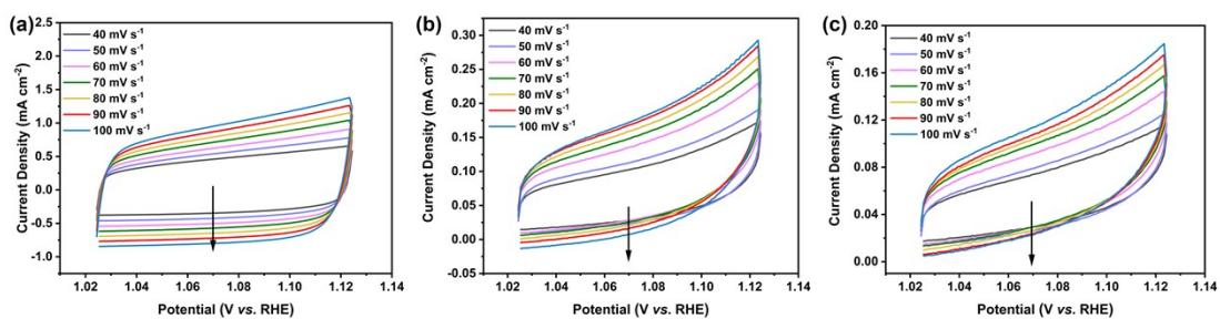
**Fig. S13.** Cyclic voltammetry curves of the (a) NiCo-O, (b) Ni-S and (c) Co-S electrodes from 40 to 100 mV s<sup>-1</sup>.
