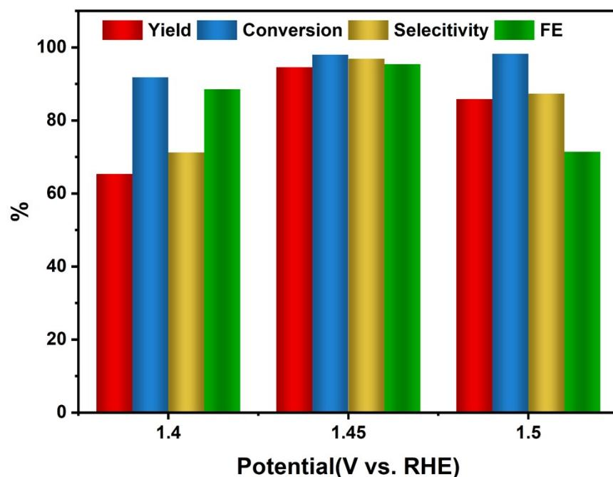
**Fig. S6.** Conversion of HMF and yield/FE/selectivity of FDCA obtained by NiCo-S electrode at different potential in 1 M KOH with 10 mM HMF.
