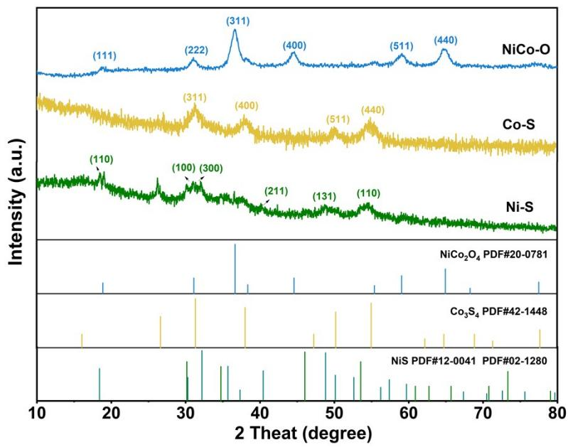
**Fig. S3.** XRD patterns of NiCo-O, Ni-S and Co-S powder sample.
