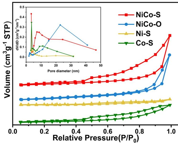
**Fig. S4.** N<sub>2</sub> adsorption-desorption isotherms of the four samples, the inset shows the corresponding pore size distribution.
