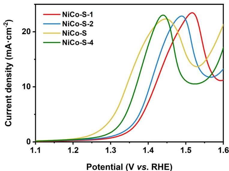
**Fig. S8.** The LSV for bimetallic sulfide catalysts with various Ni to Co ratio measured from 1.1 V to 1.6 V vs. RHE at a scan rate of 10 mV s<sup>-1</sup> in 1 M KOH with 10 mM HMF.
