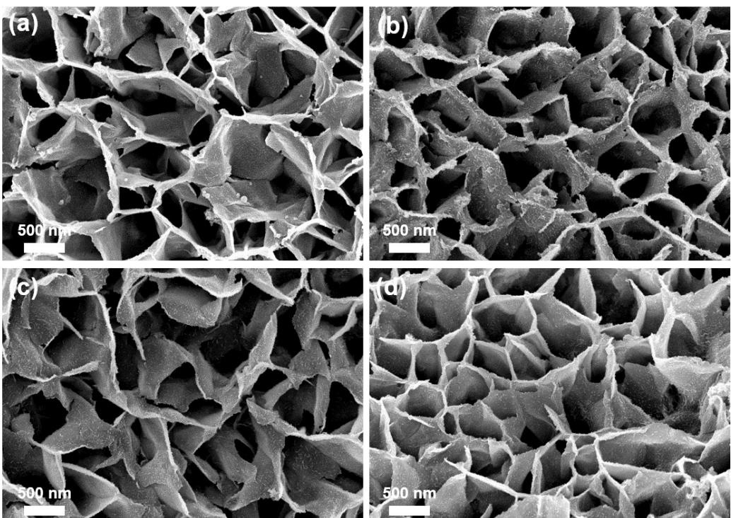
**Fig. S2.** SEM images of NiCo-S samples with various Ni to Co ratio (a) NiCo-S-1, (b) NiCo-S-2, (c) NiCo-S, and (d) NiCo-S-4.
