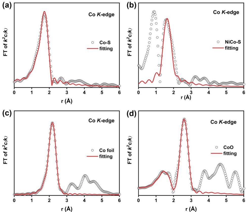
**Fig. S12.** Experimental and best fitted EXAFS spectra in the R space of Co-S (a), and NiCo-S (b) with Co foil (c) and CoO (d) as the references at the Co K-edge.
