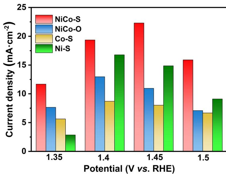
**Fig. S7.** Comparison of HMF oxidation current density at the potential between 1.35 to 1.5 V vs RHE.
