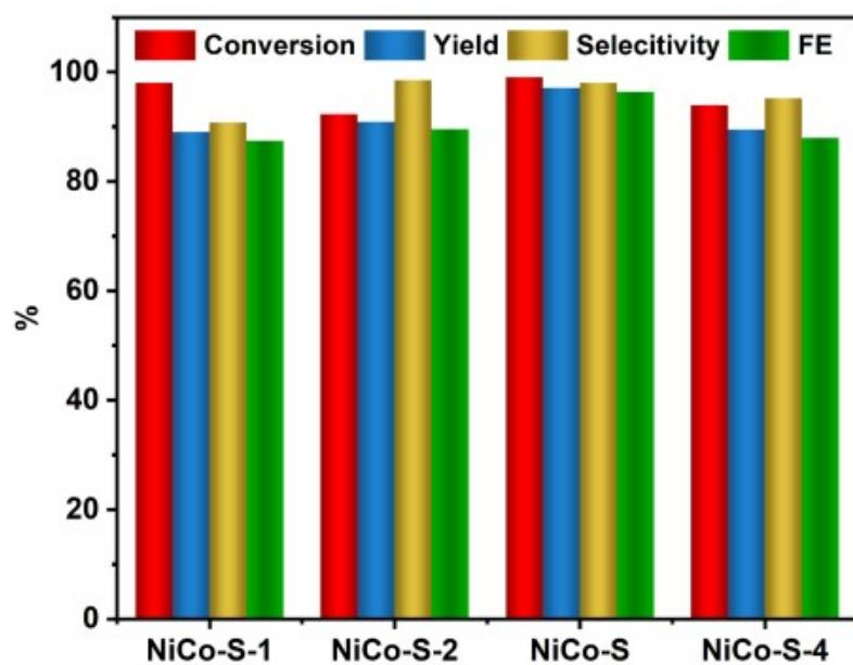
**Fig. S9.** Conversion of HMF and yield/FE/selectivity of FDCA of sulfides with varied Ni/Co ratios. The above tests were examined in 1 M KOH with 10 mM HMF at 1.45 V vs. RHE.
