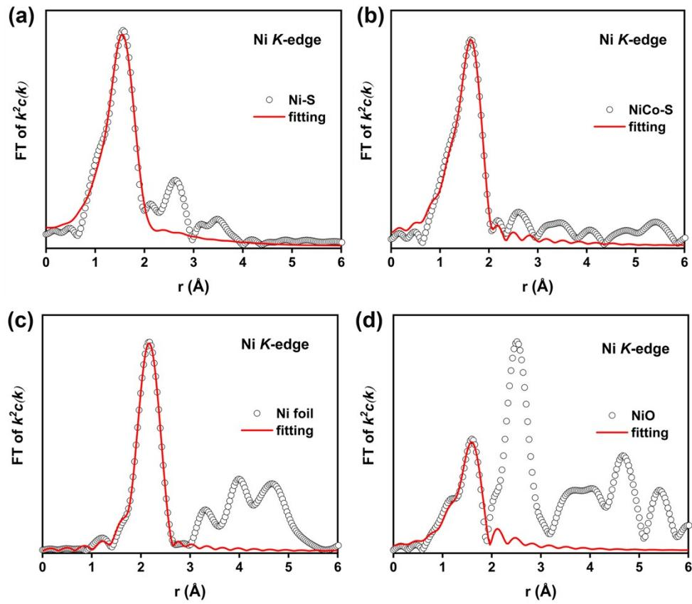
**Fig. S11.** Experimental and best fitted EXAFS spectra in the R space of Ni-S (a), and NiCo-S (b) with Ni foil (c) and NiO (d) as the references at the Ni K-edge.
