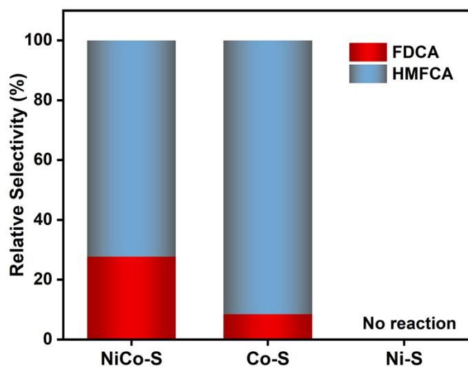
**Fig. S10.** The relative selectivity of different products obtained by NiCo-S, Ni-S, and Co-S electrodes. The above tests were carried out in 1 M KOH with 10 mM HMF at 1.3 V vs RHE.
