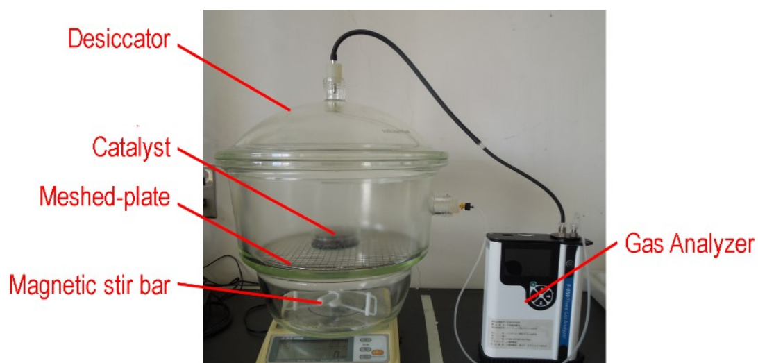
Figure S4. A reaction system for test reaction using ethylene gas to measure ethylene oxidation activity of the catalysts. Reaction conditions: catalyst Pt/A380 7.0 g, initial concentration of ethylene 50 ppm, rotational speed 1,000 rpm, initial relative humidity 50%, desiccator 10.5 L.
