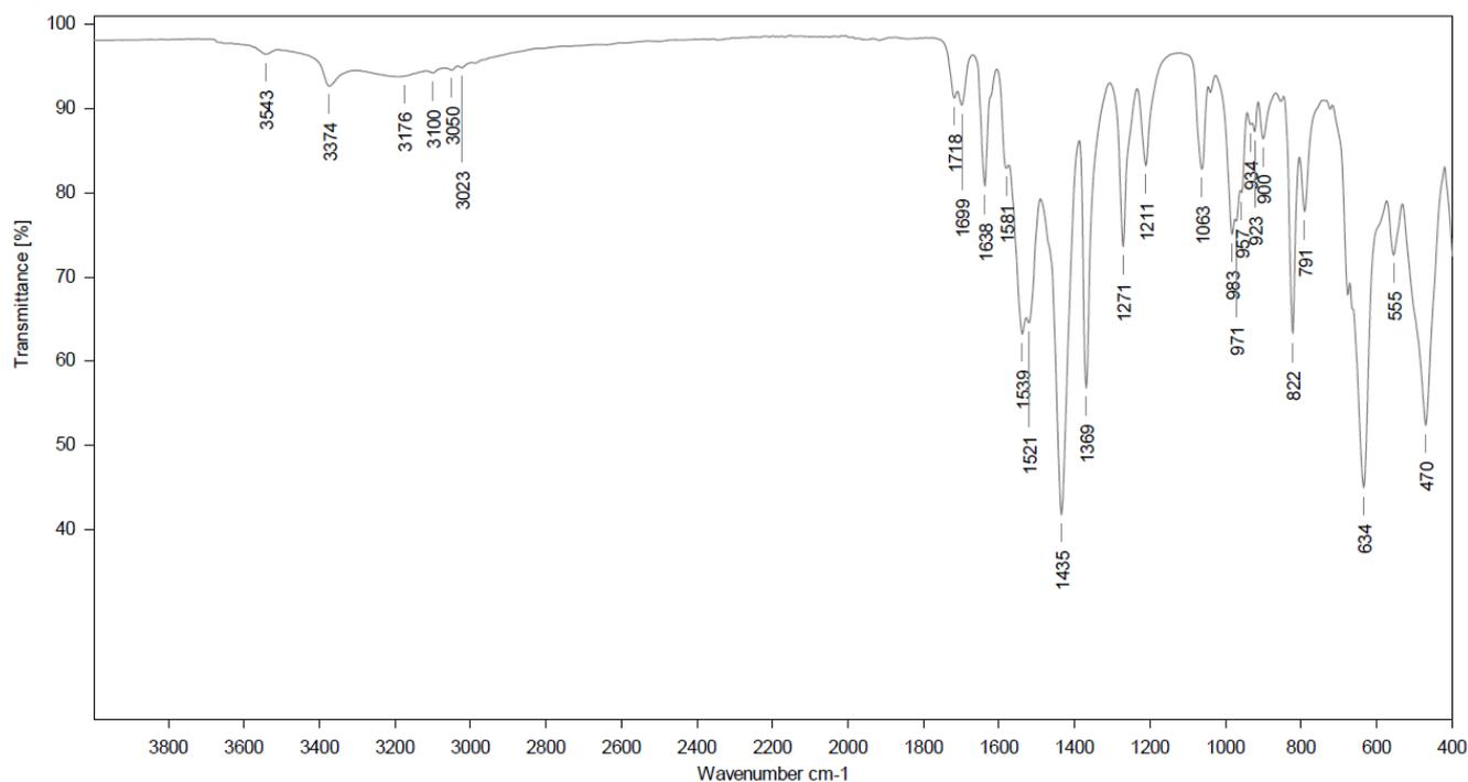
Figure S1. Infrared of  $Zr_{12}$  cluster as synthesized.
