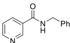
General procedure G was followed using **Zr<sub>12</sub>** cluster (10.0  $\mu\text{mol}$ , 34.8 mg), 4-nicotinic acid (62.0 mg, 0.500 mmol), benzylamine (0.16 g, 1.50 mmol), 1,4-Dioxane (0.15 mL). The reaction was stirred at 95 °C for 28 h. Analysis by  $^1\text{H}$  NMR with 3,5-bistrifluoromethyl-bromobenzene as internal standard, and comparison with previous spectral description, showed the product formation in 45% yield.<sup>16</sup>
