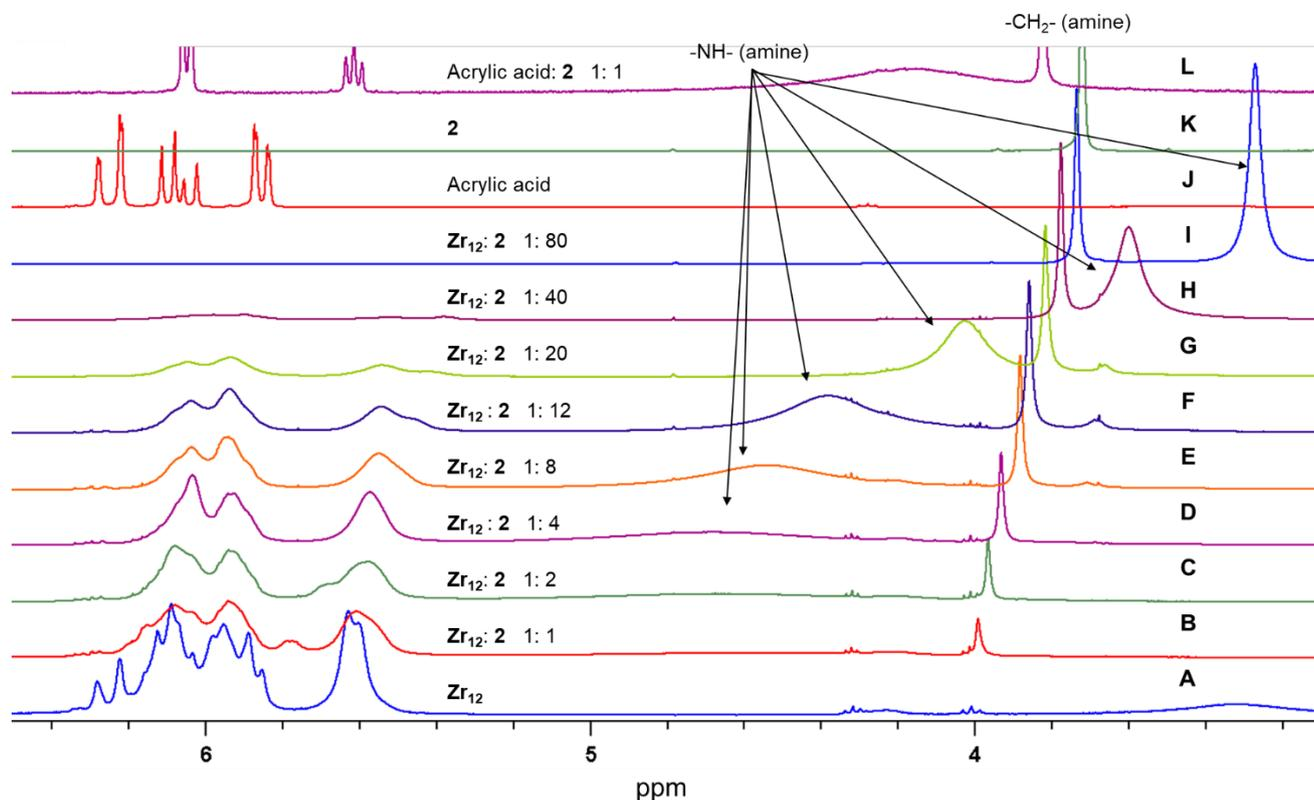
**Figure S5.**  $^1\text{H}$  NMR of benzylamine **2** and  $\text{Zr}_{12}$  cluster when **2** was slowly added to the solution of  $\text{Zr}_{12}$  cluster.  $\text{Zr}_{12}$  at equivalent concentration to the standard reaction condition (A). Solution (A) plus 1 equiv. (B), 2 equiv. (C), 4 equiv. (D), 8 equiv. (E), 12 equiv. (F), 20 equiv. (G), 40 equiv. (H), 80 equiv. (I) of **2**. Acrylic acid (J). **2** (K). Mixture of acrylic acid and **2** with a ratio of 1:1 (L).
