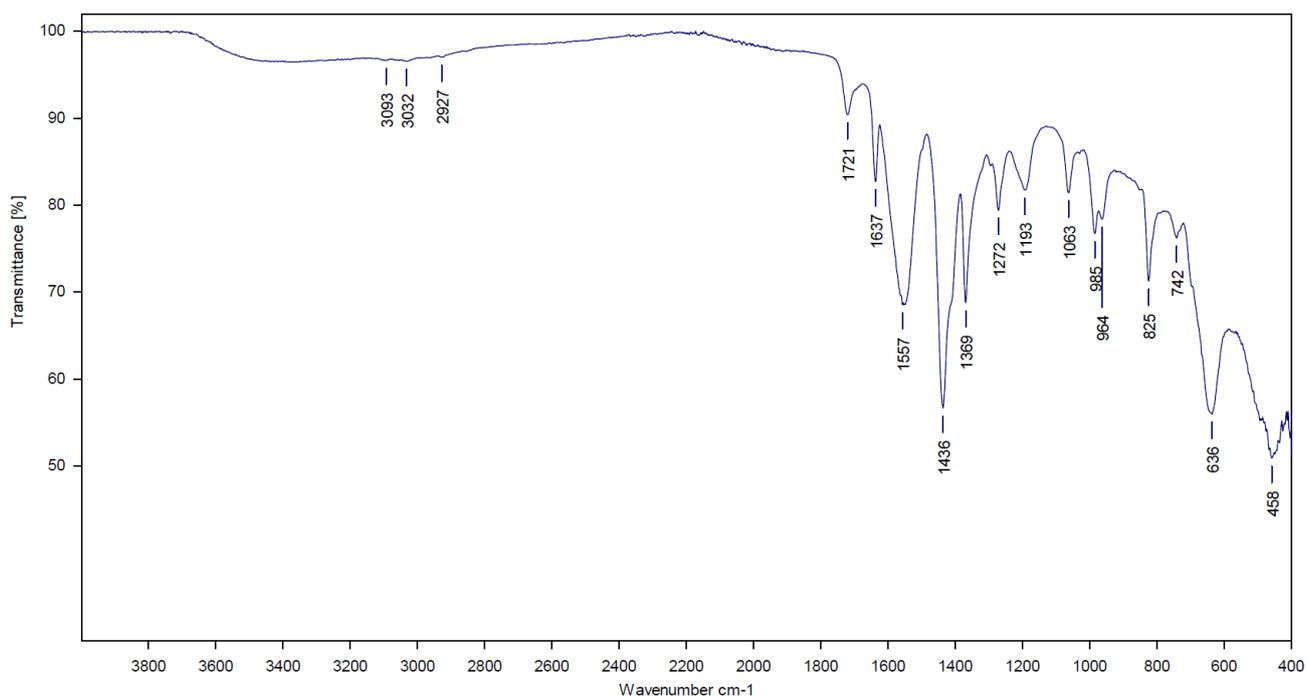
**Figure S7.** Infrared of recovered  $Zr_{12}$  cluster after treating it with an excess of acrylic acid.
