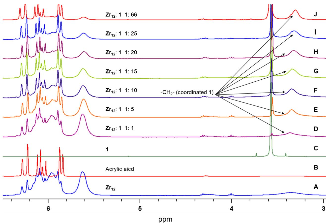
**Figure S3.**  $^1$ H NMR of phenylacetic acid **1** and  $Zr_{12}$  cluster mixtures.  $Zr_{12}$  at equivalent concentration to the standard reaction condition (A). Acrylic acid (B). **1** (C). Solution (A) plus 1 equiv. (D), 5 equiv. (E), 10 equiv. (F), 15 equiv. (G), 20 equiv. (H), 25 equiv. (I), 66 equiv. (J) of **1**.
