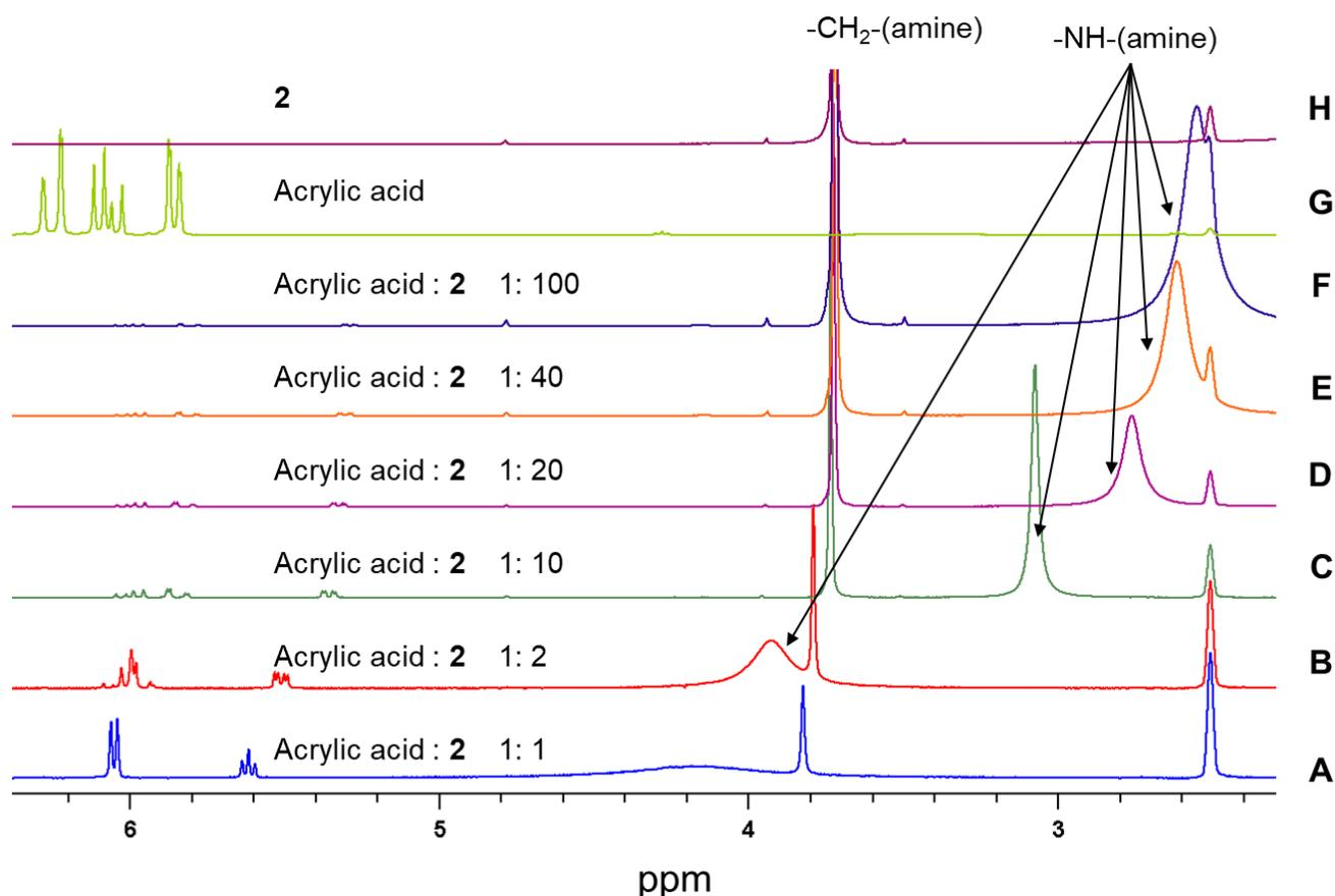
**Figure S4.**  $^1\text{H}$  NMR of acrylic acid and **2** mixture. Acrylic acid (0.0075 mmol) plus 1 equiv. (A), 2 equiv. (B), 10 equiv. (C), 20 equiv. (D), 40 equiv. (E), 100 equiv. (F) of **2**. Acrylic acid (G). Pure **2** (H).
