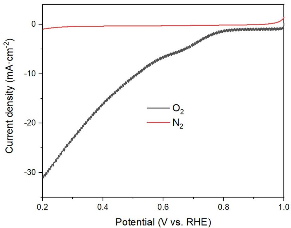
**Figure S3** LSV curves of Co<sub>1</sub>/NC measured in N<sub>2</sub>-saturated and O<sub>2</sub>-saturated solution.
