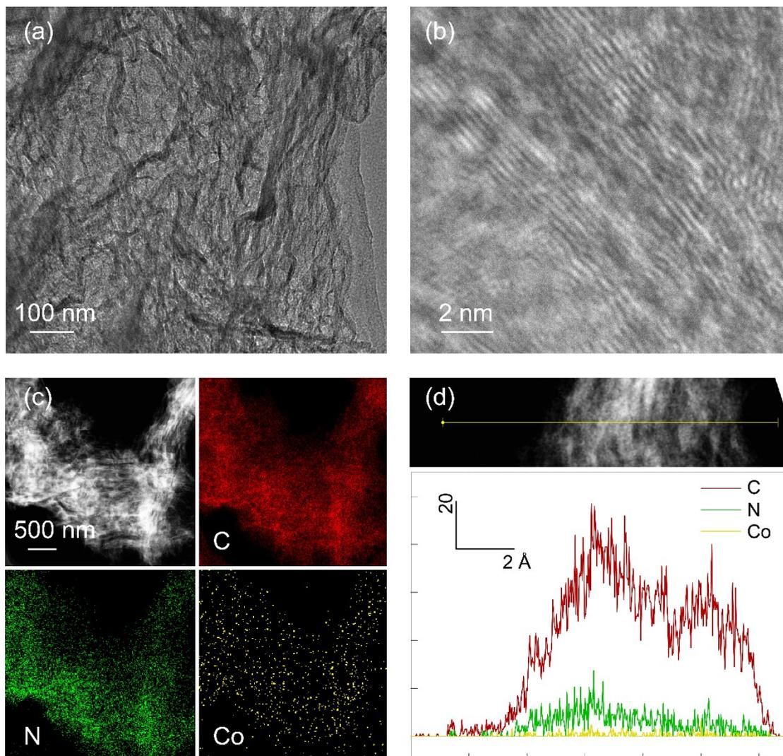
**Figure S1** (a-b) TEM images of Co<sub>1</sub>/NC. (c) EDS elemental mappings of Co<sub>1</sub>/NC. (d) Line scans of Co<sub>1</sub>/NC.
