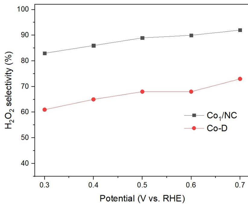
**Figure S4** H<sub>2</sub>O<sub>2</sub> selectivity of Co<sub>1</sub>/NC and Co-D.
