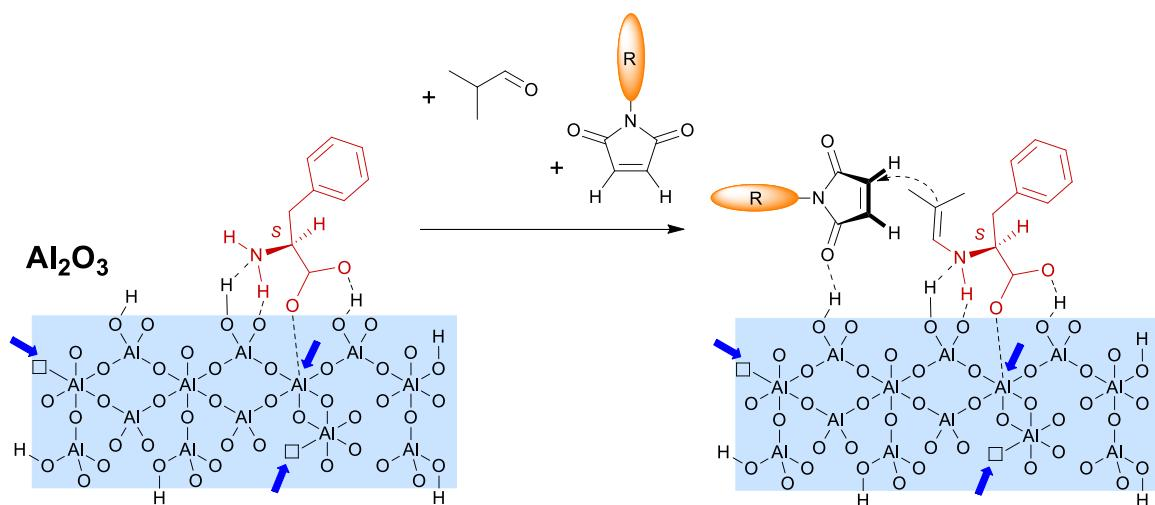
**Fig. S17** Possible adsorption mode of L-Phe on Al<sub>2</sub>O<sub>3</sub> surface and the structure of the surface transition state.
