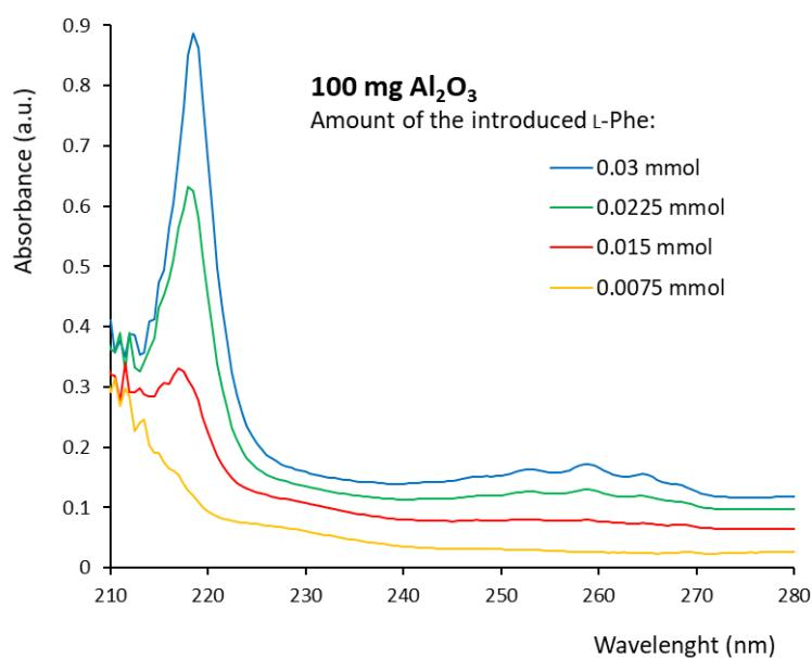
**Fig. S11** UV-Vis spectra of L-Phe solutions obtained from the supernatant resulted following stirring the given amount of amino acid and 100 mg Al<sub>2</sub>O<sub>3</sub> in 1 cm<sup>3</sup> MeOH for 2 h.
