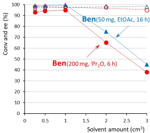
**Fig. S4** Effect of the solvent amount on the Conv (closed symbols) and ee (open symbols) in the addition isobutyraldehyde (**1a**) to *N*-benzylmaleimide (**2a**) using 50 mg Ben in EtOAc for 16 h (**▲**, **△**) and 200 mg Ben in *i*Pr<sub>2</sub>O for 6 h (**●**, **○**). Reaction conditions: L-Phe 0.03 mmol (10 mol%), 1.2 mmol **1a**, 0.3 mmol **2a**, rt.
