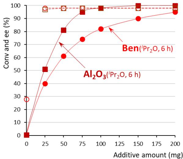
**Fig. S1** Effect of the additive amount on the Conv (closed symbols) and ee (open symbols) obtained in the addition of isobutyraldehyde (**1a**) to *N*-benzylmaleimide (**2a**) using Ben (●, ○) or  $\text{Al}_2\text{O}_3$  (■, □) additive in diisopropyl ether. Reaction conditions: 0.03 mmol (10 mol%) L-Phe, 1.2 mmol **1a**, 0.3 mmol **2a**, 1 cm<sup>3</sup>  $i\text{Pr}_2\text{O}$ , rt, 6 h.
