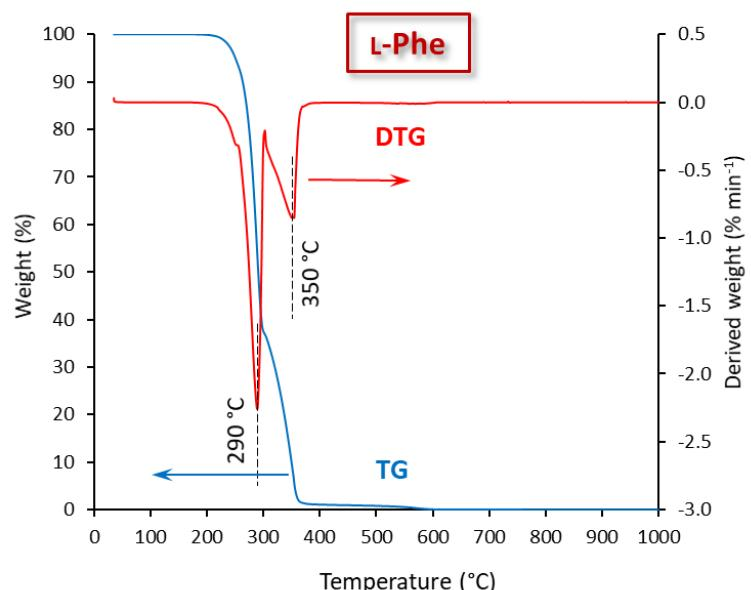
**Fig. S13** Thermogravimetric analysis of L-Phe.
