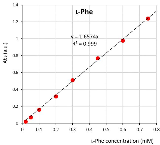
**Fig. S9** Calibration plot used to determine the concentration of L-Phe remained in or desorbed to the liquid phase.
