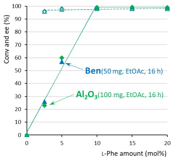
**Fig. S2** Effect of L-Phe amount on the Conv (closed symbols) and ee (open symbols) in the addition of isobutyraldehyde (**1a**) to *N*-benzylmaleimide (**2a**) using 50 mg Ben (▲, △) or 100 mg  $\text{Al}_2\text{O}_3$  (◆, ◇) additive. Reaction conditions: 1.2 mmol **1a**, 0.3 mmol **2a**, 1 cm<sup>3</sup> solvent, rt, 16 h.
