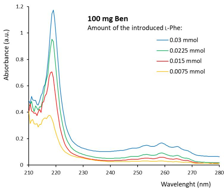
**Fig. S10** UV-Vis spectra of L-Phe solutions obtained from the supernatant resulted following stirring the given amount of amino acid and 100 mg Ben in 1 cm<sup>3</sup> MeOH for 2 h.
