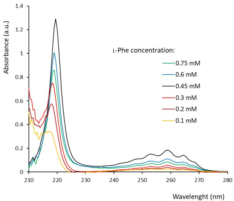
**Fig. S8** UV-Vis spectra of L-Phe solutions of increasing concentrations in MeOH used for calibration.
