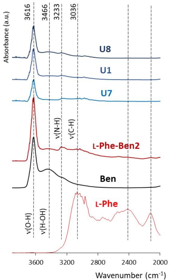
**Fig. S16** Selected ranges of the FT-IR spectra of L-Phe, Ben, L-Phe-Ben2 and three materials used in reactions of **1a** and **2a** in 1 cm<sup>3</sup> *t*Pr<sub>2</sub>O; **U1** (see Fig. 7); 55 mg of L-Phe-Ben2 after first use in a 6 h reaction at 50°C, Conv 99 %, ee 96.5 %, (**U7**); *in situ* formed material from 200 mg Ben and 0.03 mmol L-Phe, in 6 h reactions at rt: **U5** after ten uses, last run Conv 62 %, ee 98 % (**U8**).
