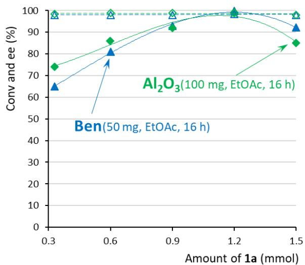
**Fig. S3** Effect of the isobutyraldehyde (**1a**) amount on the Conv (closed symbols) and ee (open symbols) in the addition to *N*-benzylmaleimide (**2a**) using 50 mg Ben (**▲**, **△**) or 100 mg  $\text{Al}_2\text{O}_3$  (**◆**, **◇**) additive. Reaction conditions: L-Phe 0.03 mmol (10 mol%), 0.3 mmol **2a**, 1 cm<sup>3</sup> EtOAc, rt, 16 h.
