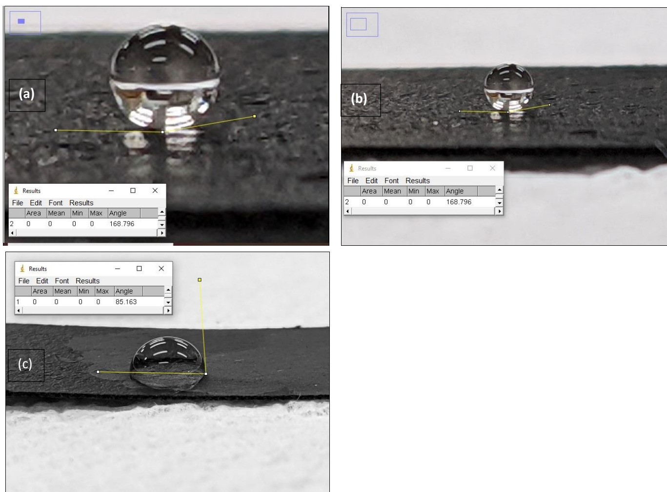
Figure S3. (a, b) Photograph of water droplets on CFP. (c) Photograph of water droplets on NiSe 2 @CFP illustrating better wetting interaction on the NiSe 2 -modified electrode.
