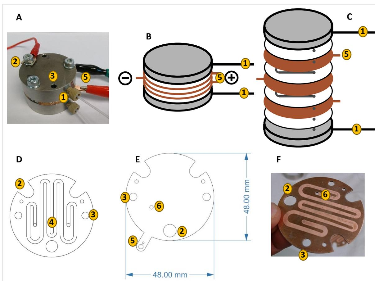
Figure S1: Continuous electrochemical reactor, A: picture of the assembled reactor, B: drawing of the assembled reactor, C: drawing of the elements of the reactor, D: spacer drawing, E: electrode drawing, F: picture of the electrode, 1: inlet and outlet, 2: holes for bolts, 3: holes for alignment, 4: flow channel, 5: connection lip, 6: hole for flow through.
