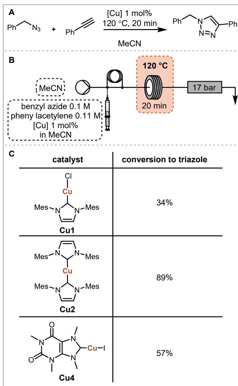
Figure S9: Model click reaction with benzyl azide and phenyl acetylene, **A**: reaction scheme; **B**: flow setup; **C**: catalyst screen, <sup>1</sup>H NMR spectroscopic triazole conversions.
