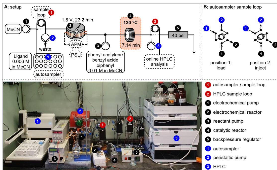
Figure S16: A: Telescoped reaction setup with autosampler; B: sample loop configuration.
