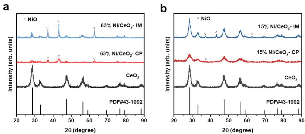
**Fig S2: a** XRD patterns of the calcined 63% Ni/CeO<sub>2</sub>-CP and 63% Ni/CeO<sub>2</sub>-IM catalysts, **b** XRD patterns of the calcined 15% Ni/CeO<sub>2</sub>-CP and 15% Ni/CeO<sub>2</sub>-IM catalysts.
