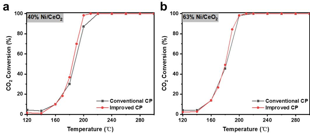
**Figure S1:** The activity comparison of Ni/CeO<sub>2</sub> catalysts synthesized by the improved and conventional co-precipitation methods a 40% Ni/CeO<sub>2</sub> b 63% Ni/CeO<sub>2</sub>
