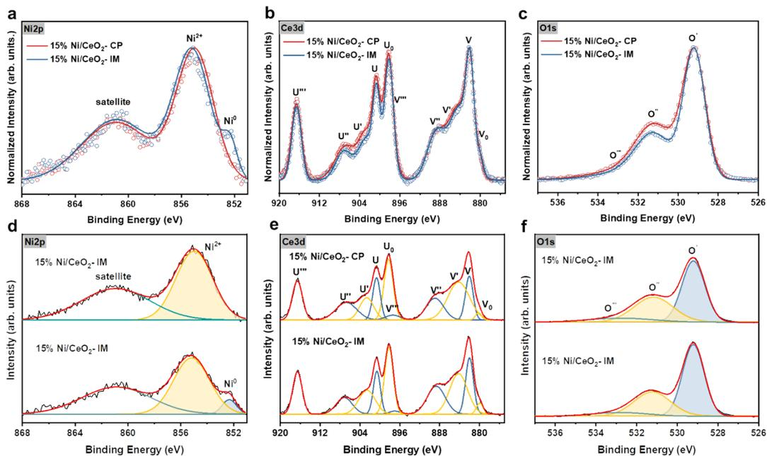
**Fig S7:** XPS spectra of **a** Ni2p, **b** Ce3d, and **c** O1s for the reduced 15% Ni/CeO<sub>2</sub>-CP and 15% Ni/CeO<sub>2</sub>-IM catalysts. Fitting XPS spectra of **d** Ni2p, **e** Ce3d, and **f** O1s for the reduced 15% Ni/CeO<sub>2</sub>-CP and 15% Ni/CeO<sub>2</sub>-IM catalysts.
