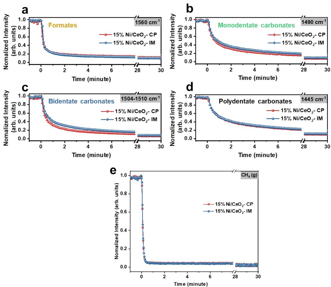
**Fig S10:** Intensity variation curves of **a**  $1560\text{ cm}^{-1}$  (Formates), **b**  $1490\text{ cm}^{-1}$  (Monodentate carbonates), **c**  $1504\sim 1510\text{ cm}^{-1}$  (Bidentate carbonates), **d**  $1445\text{ cm}^{-1}$  (Polydentate carbonates), and **e** gaseous  $\text{CH}_4$  upon switching from  $\text{CO}_2+\text{H}_2$  ( $n(\text{H}_2):n(\text{CO}_2) = 80:1$ ) to  $\text{H}_2$  at  $350\text{ }^\circ\text{C}$  during 30 minutes.
