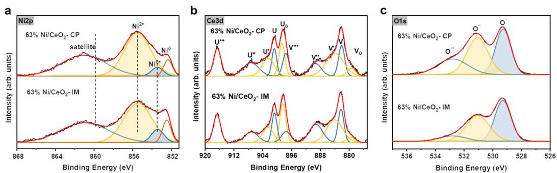
**Fig S5:** Fitting XPS spectra of **a** Ni2p, **b** Ce3d, and **c** O1s for the reduced 63% Ni/CeO<sub>2</sub>-CP and 63% Ni/CeO<sub>2</sub>-IM catalysts.
