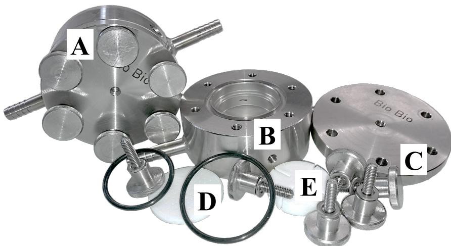
**Figure S1.** Membrane reactor used within this study (fully assembled, A) consisting of a lower part (B) and an upper part (C) together with the membrane holder for stabilization of the membrane (D) and the magnetic stirrer (E).
