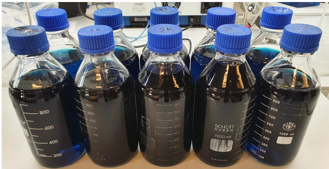
**Figure S9.** Continuous production of ABTS<sup>•+</sup>-radical (see also Figure 6). Conditions:  $1 \text{ mL} \cdot \text{min}^{-1}$ , total produced volume: 10.2 L, total run time: 6.9 days, reactor volume ( $V_R$ ): 2.36 mL,  $\tau_{\text{exp}}$ : 2.94 min (0.049 h).
