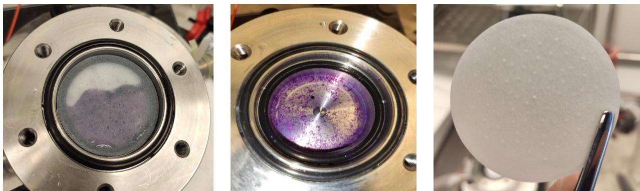
**Figure S2.** Top-down view of the membrane reactor after the first enzymatic run with a flow rate of  $0.5 \text{ mL}\cdot\text{min}^{-1}$  (with a flow-proportion of 90%  $0.3 \text{ mmol}\cdot\text{L}^{-1}$  ABTS and 10% of 3.5% (v/v)  $\text{H}_2\text{O}_2$  solution). Purple crystals were formed and in direct contact with the membrane (left) and dispersed throughout the entire volume of the reactor (middle). Due to resulting high pressures, the membrane was damaged (right).
