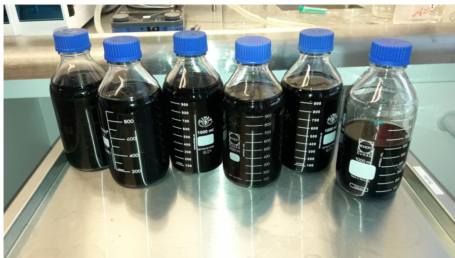
**Figure S7.** Continuous production of ABTS<sup>•+</sup>-radical (see Table 3, Figure 5).
