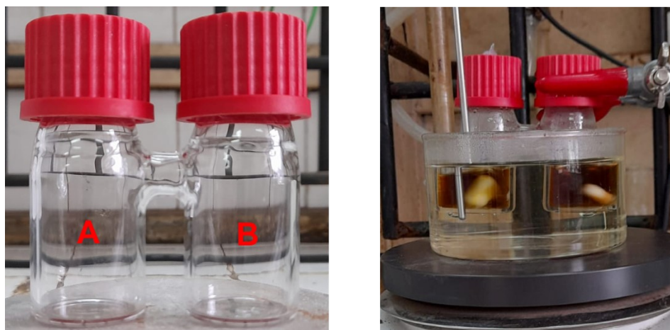
Figure S1. Glass apparatus used for the hydroformylation of safrole under isomerization conditions.
