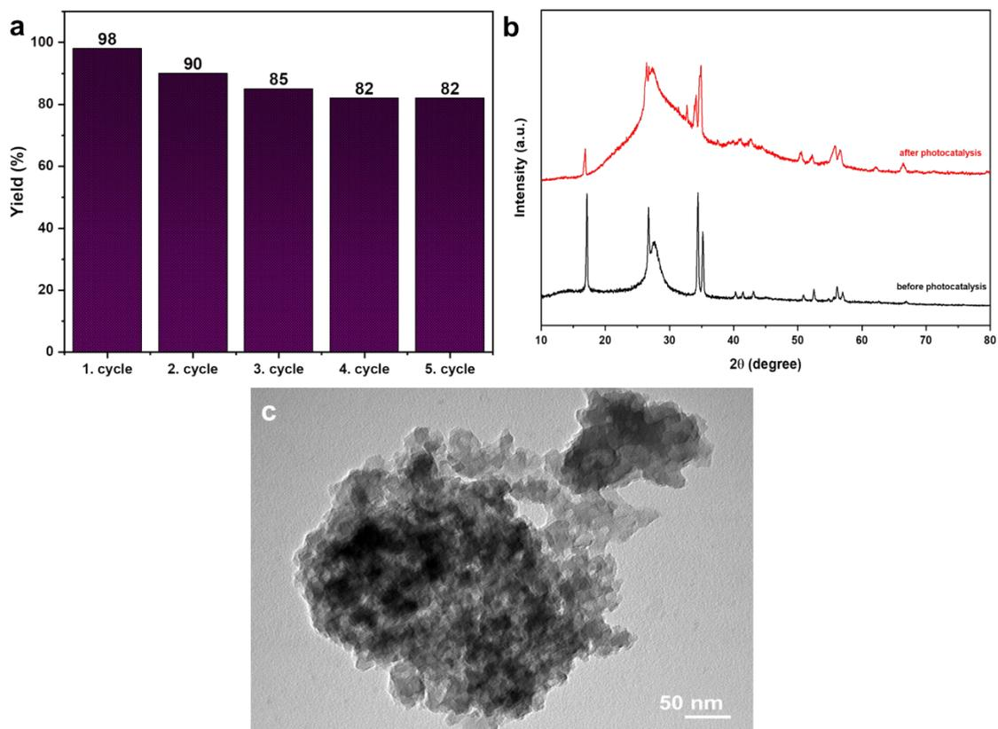
**Figure S4.** a. Five-run reusability test b. XRD pattern c. TEM image of FLBP/g-CN heterojunction.
