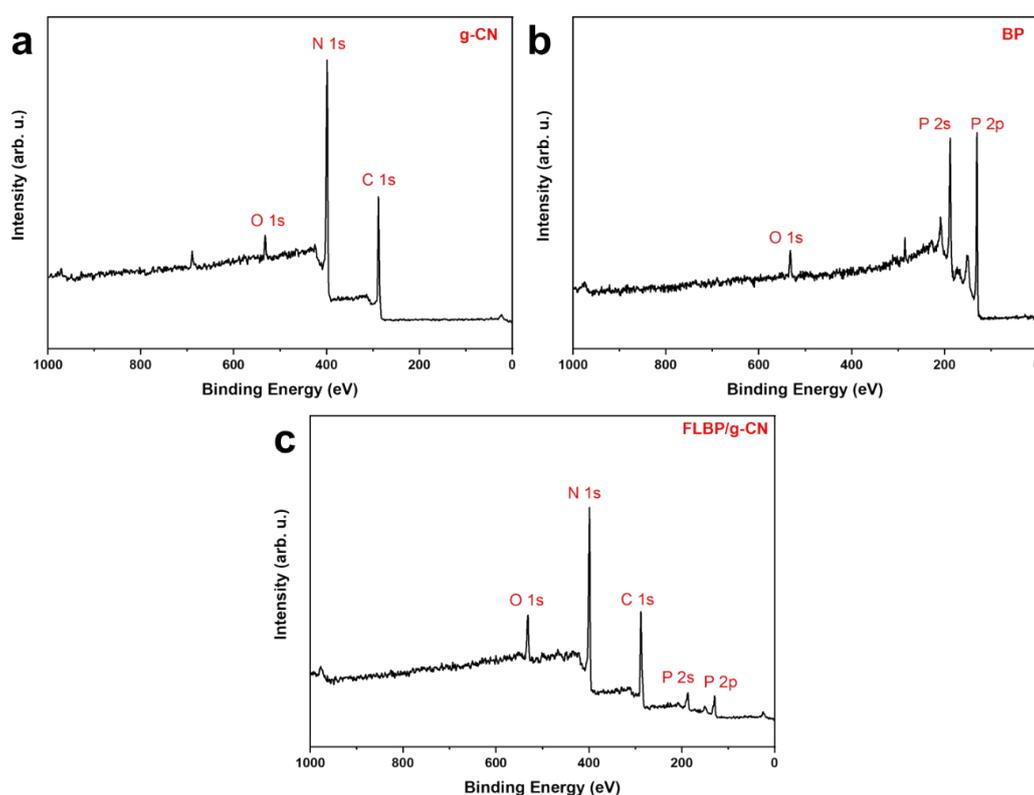
**Figure S1.** XPS survey spectra of **a.** BP, **b.** g-CN and **c.** FLBP/g-CN heterojunctions.
