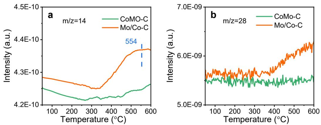
Fig. S9 MS signals of (a)  $m/z=14$  and (b)  $m/z=28$  during  $\text{N}_2$ -TPD.
