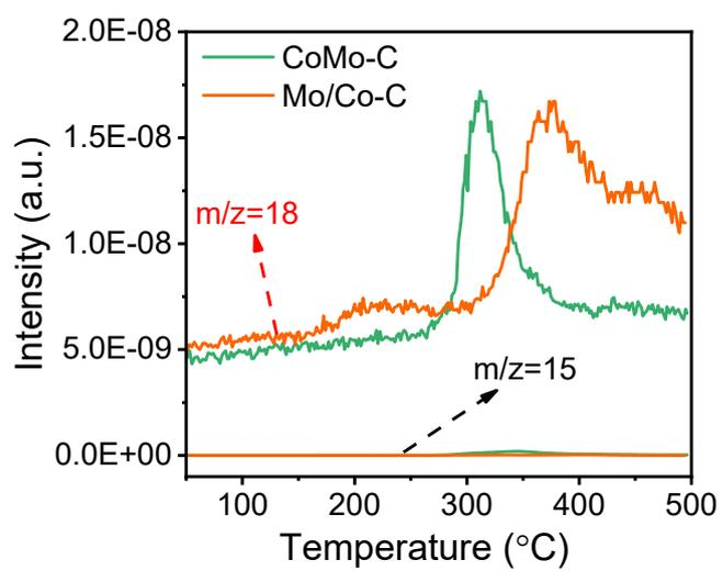
Fig. S6 MS signals of  $m/z=18$  and  $m/z=15$  during  $H_2$ -TPR.
