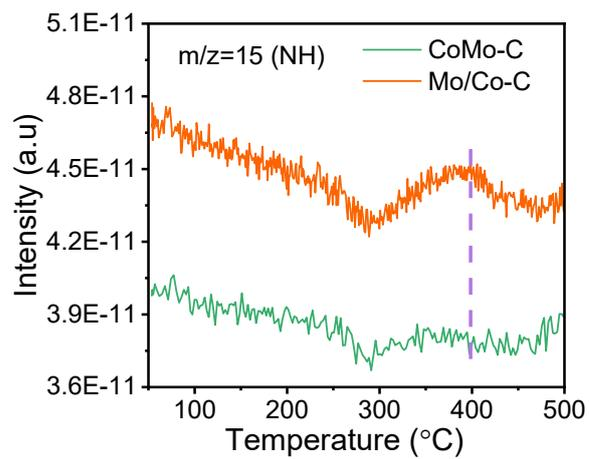
Fig. S13 MS signals of a  $m/z=15$  (NH) during TPSR over catalysts pre-adsorbed with  $D_2$ .
