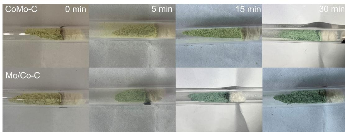
Fig. S11 **Color change photographs of the mixtures.** Photographs of samples made with  $\text{WO}_3$  mixed with the catalysts before treatment (0 min) and after treatment with  $\text{H}_2$  at  $300^\circ\text{C}$  for 5 min, 15 min and 30 min.
