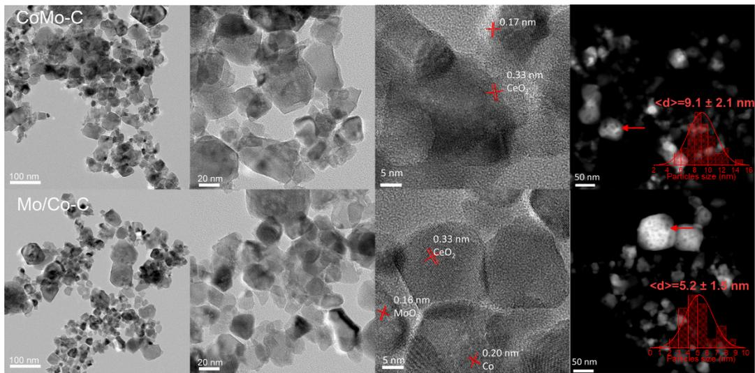
Fig. S3 TEM images and Co-Mo particle size distribution in the inset.
