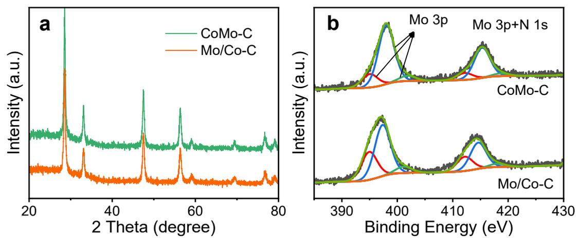
Fig S12 XRD pattern of used catalysts and Mo 3p+N 1s spectrum of catalysts with treatment in  $N_2$ - $H_2$  mixture.
