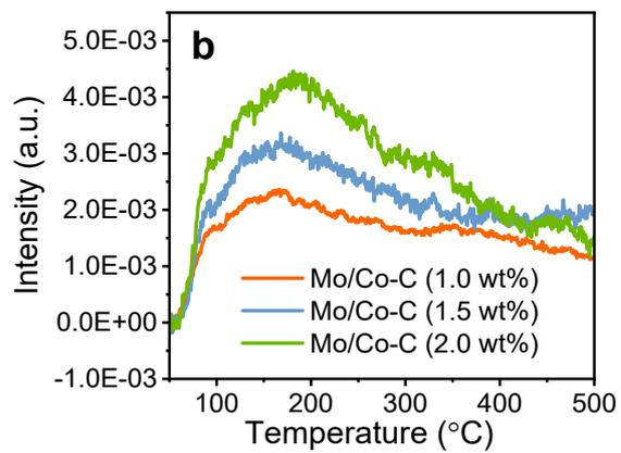
Fig. S10 H<sub>2</sub>-TPD profile over catalysts with different Co loadings.
