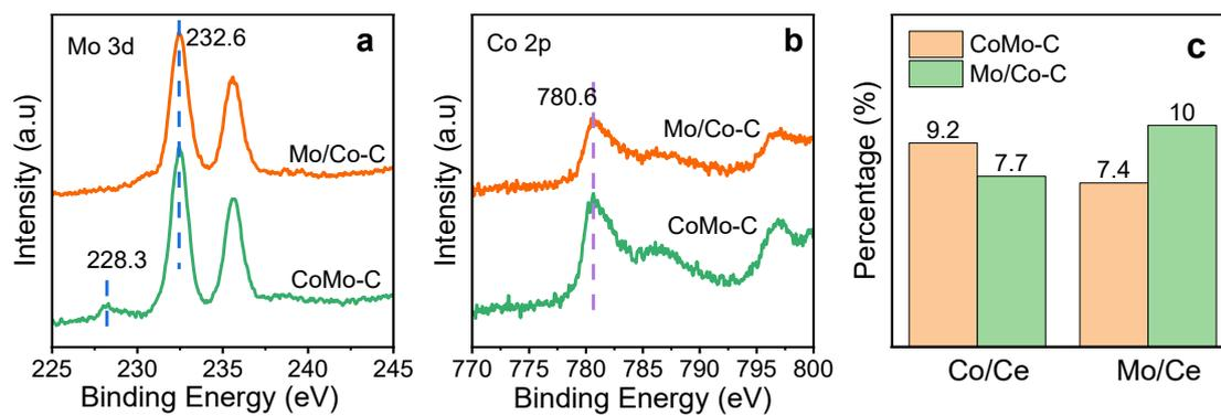
Fig. S4 XPS spectra of the as-prepared samples: (a) Mo 3d, (b) Co 2p and (c) the percentage of Co/Ce and Mo/Ce.
