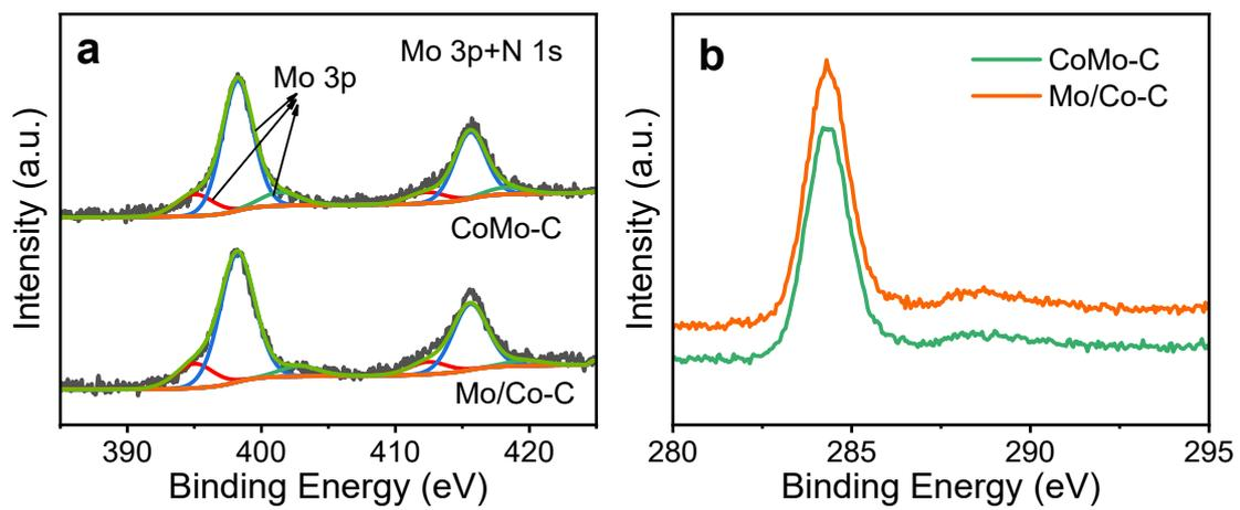
Fig. S5 XPS spectra of the as-prepared samples: (a) Mo 3p+N 1s, (b) C 1s.
