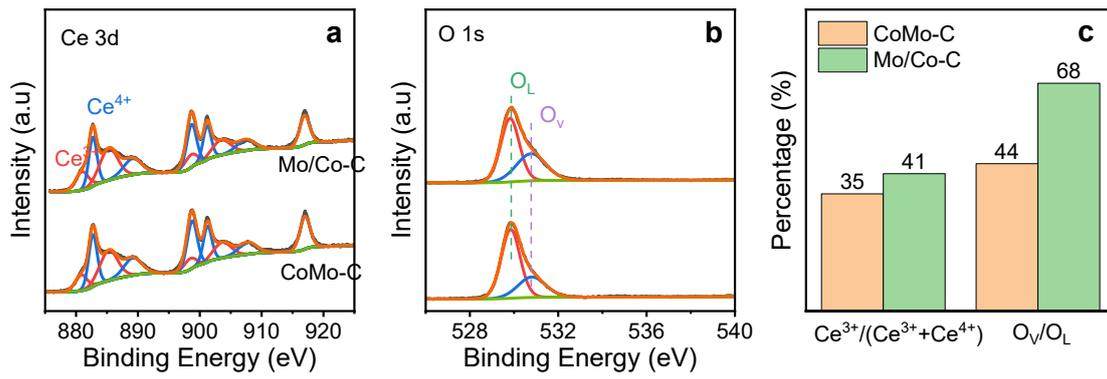
Fig. S8 XPS spectra of the reduced catalysts: (a) Ce 3d, (b) O 1s and (c) the ratios of  $Ce^{3+}/(Ce^{3+}+Ce^{4+})$  and  $O_V/O_L$ .
