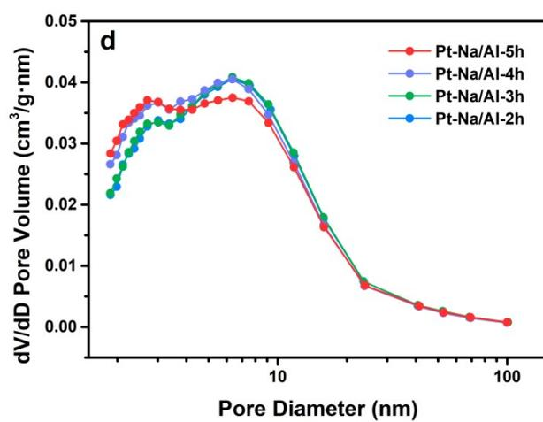
**Figure S5.** N<sub>2</sub> adsorption-desorption isotherms and the corresponding pore size distributions of Al-2h, Al-3h, Al-4h and Al-5h supports, and Pt-Na/Al-2h, Pt-Na/Al-3h, Pt-Na/Al-4h and Pt-Na/Al-5h catalysts.
