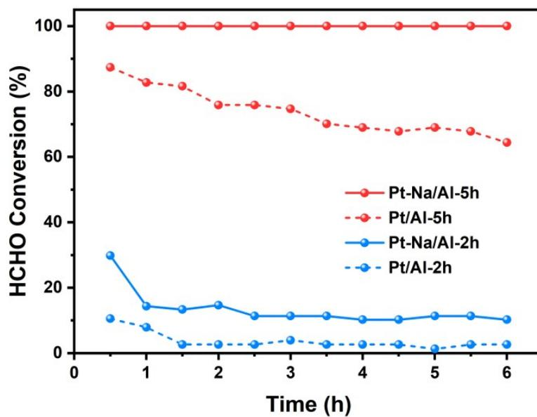
**Figure S10.** HCHO catalytic oxidation performance of Pt-Na/Al-5h, Pt-Na/Al-2h, Pt/Al-5h and Pt/Al-2h. Reaction conditions: 25 °C, 110 ppm of HCHO, 20 vol % O<sub>2</sub>, 35 % RH, N<sub>2</sub> balanced and WHSV of 200 000 mL/ (g h).
