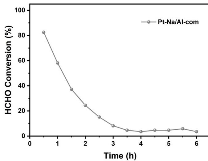
**Figure S1.** HCHO catalytic oxidation performance of Pt-Na/Al-com. Reaction conditions: 25 °C, 110 ppm of HCHO, 20 vol % O<sub>2</sub>, 35 % RH, N<sub>2</sub> balanced and WHSV of 200 000 mL/ (g h).
