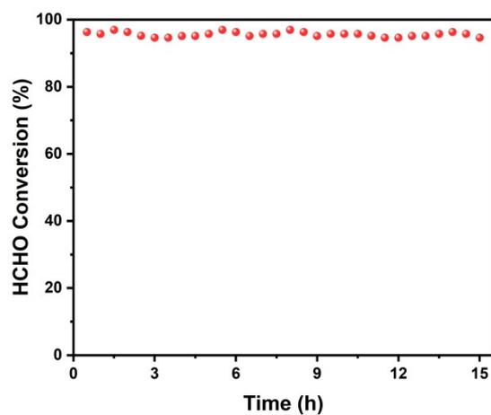
**Figure S3.** The HCHO oxidation stability of Pt-Na/Al-5h. Reaction conditions: 25 °C, 180 ppm of HCHO, 20 vol % O<sub>2</sub>, 35 % RH, N<sub>2</sub> balanced and WHSV of 120 000 mL/(g h).
