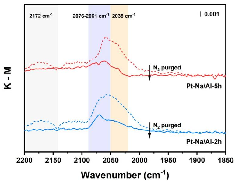
**Figure S9.** In-situ DRIFTS results of Pt-Na/Al-2h and Pt-Na/Al-5h at 30 °C. Reaction condition:  $\text{CO}+\text{N}_2$  adsorption for 30 min,  $\text{N}_2$  purged for 30 min.
