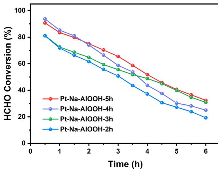
**Figure S8.** HCHO catalytic oxidation performance of Pt-Na-AIOOH-2h, Pt-Na-AIOOH-3h, Pt-Na-AIOOH-4h and Pt-Na-AIOOH-5h. Reaction conditions: 25 °C, 110 ppm of HCHO, 20 vol % O<sub>2</sub>, 35 % RH, N<sub>2</sub> balanced and WHSV of 200 000 mL/ (g h).
