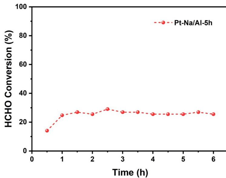
**Figure S11.** HCHO catalytic oxidation performance of Pt-Na/Al-5h. Reaction conditions: 25 °C, 110 ppm of HCHO, 20 vol % O<sub>2</sub>, 0 % RH, N<sub>2</sub> balanced and WHSV of 200 000 mL/(g h).
