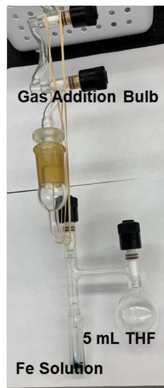
Figure S47. Teflon sealed UV-Vis cuvette with attached round bottom flask, affixed with 4 mL gas addition bulb.
