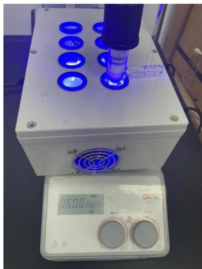
**Photograph of the Photocatalytic reactor used for reactions conducted under blue LED irradiation.**
