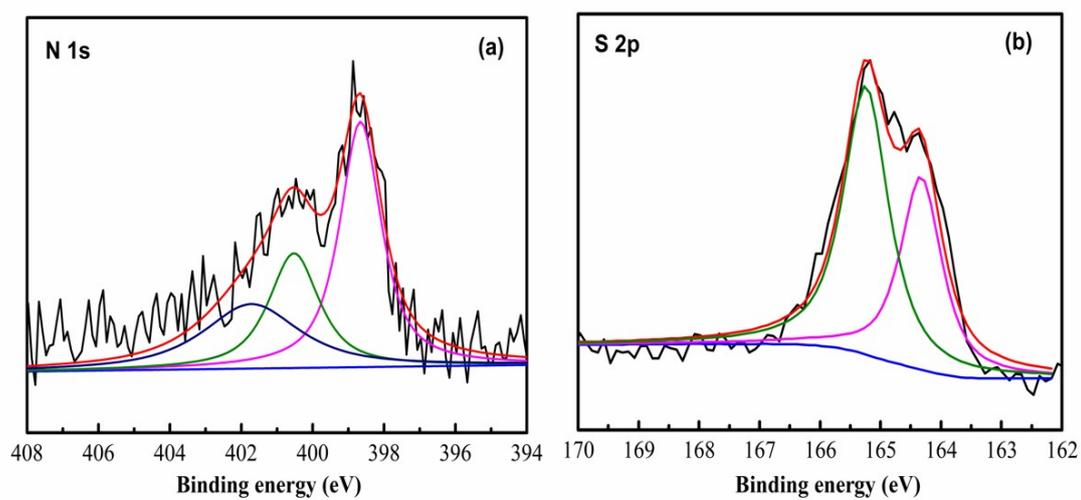
**Fig. S2** N 1s and S 2p XPS spectra of the C1-2N (a) and C5-0N (b) samples
