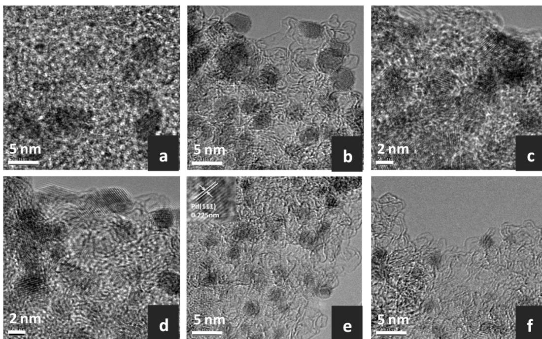
**Fig. S1** The high-resolution TEM images of the Pd/C catalysts: (a) Pd/C0, (b) Pd/C1, (c) Pd/C2, (d) Pd/C3, (e) Pd/C4, and (f) Pd/C5.
