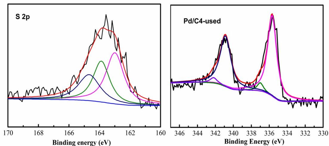
**Fig. S5** S 2p and Pd 3d XPS spectra of the Pd/C4-used catalyst
