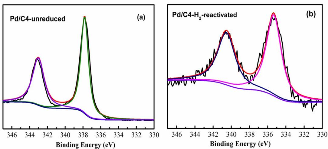
**Fig. S4** XPS spectra of the Pd/C4-unreduced (a) and Pd/C4-H<sub>2</sub>-reactivated (b) catalyst.
