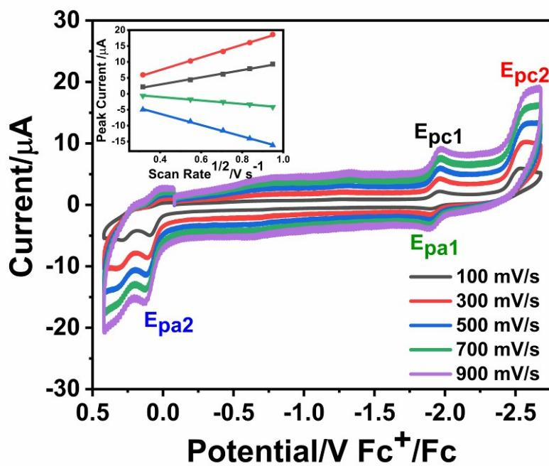
**Figure S14.** CVs of **4** recorded at scan rates from  $100 \text{ mV s}^{-1}$  to  $900 \text{ mV s}^{-1}$  in DMF solution with  $0.1 \text{ M}$  n-Bu<sub>4</sub>NPF<sub>6</sub> as the supporting electrolyte and using a glassy carbon working electrode. Inset: Plots of peak current versus the square root of scan rate.
