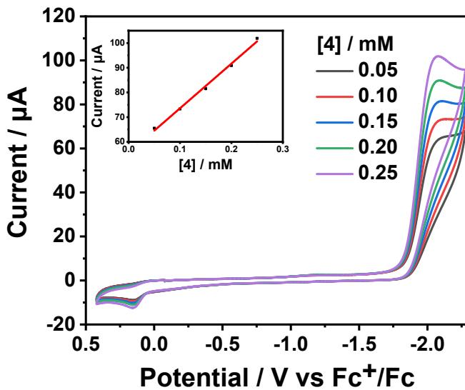
**Figure S24.** CVs of 0.05-0.25 mM **4** in DMF with 67.32 mM TFA at a scan rate of 100 mV s<sup>-1</sup> (0.1 M n-Bu<sub>4</sub>NPF<sub>6</sub> supporting electrolyte; glassy carbon working electrode). Insert: Plot of the  $i_{\text{cat}}$  against the complex **4** concentration.
