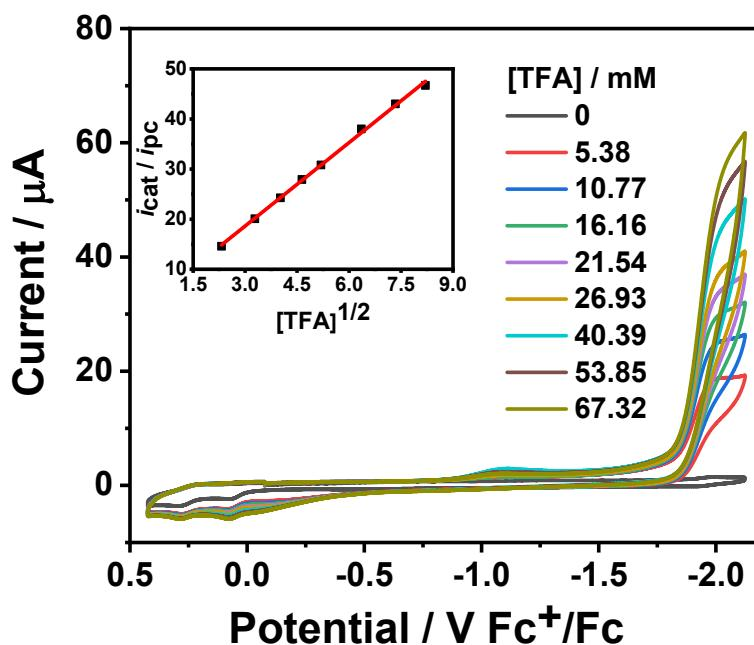
**Figure S19.** CVs of 0.25 mM **5** in DMF with different TFA concentrations (0, 5.38, 16.15, 21.54, 26.92, 40.39, 53.85, and 67.32 mM) at a scan rate of 100 mV s<sup>-1</sup> (0.1 M n-Bu<sub>4</sub>NPF<sub>6</sub> supporting electrolyte; glassy carbon working electrode). Inset: Plot of the  $i_{\text{cat}} / i_{\text{pc}}$  against the square root of TFA concentration.
