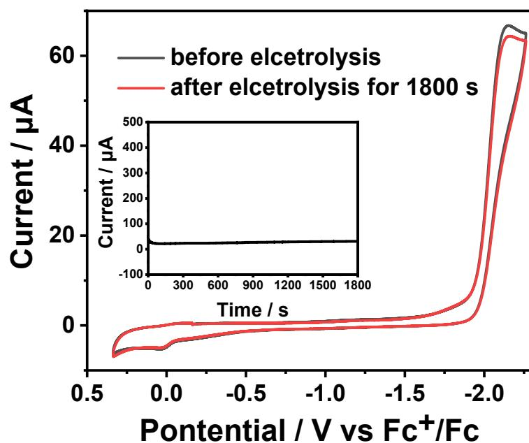
**Figure S40.** Cyclic voltammograms of 0.25 mM **3** with 26.93 mM TFA before and after electrolysis. Inset: Amperometric i-t curve of **3** at a constant potential of -2.00 V. (0.1 M n-Bu<sub>4</sub>NPF<sub>6</sub> supporting electrolyte; glassy carbon working electrode; scan rate 100 mV s<sup>-1</sup>).
