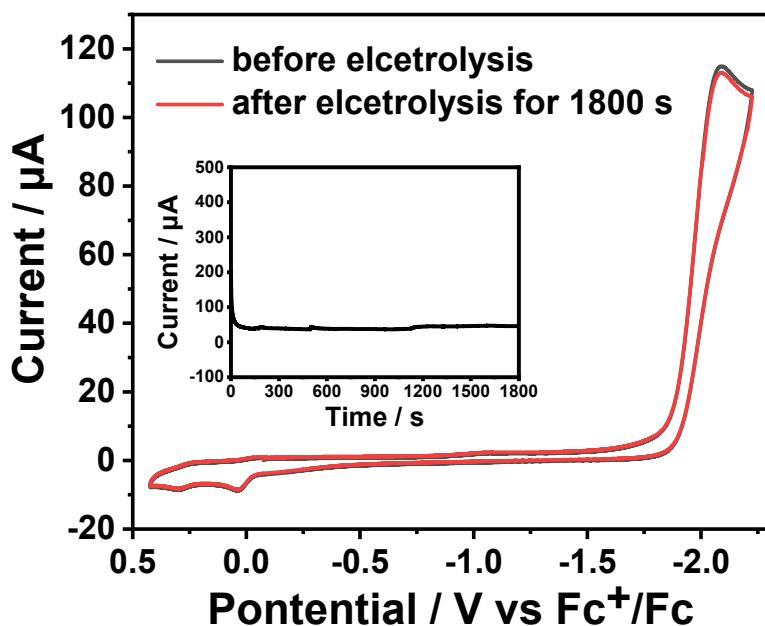
**Figure S39.** Cyclic voltammograms of 0.25 mM **2** with 26.93 mM TFA before and after electrolysis. Inset: Amperometric i-t curve of the **2** at a constant potential of -2.00 V. (0.1 M n-Bu<sub>4</sub>NPF<sub>6</sub> supporting electrolyte; glassy carbon working electrode; scan rate 100 mV s<sup>-1</sup>).
