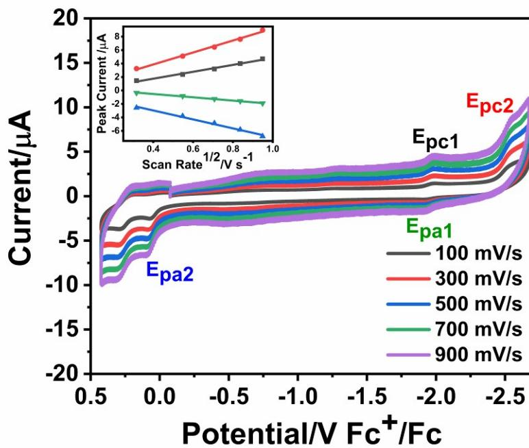
**Figure S15.** CVs of **5** recorded at scan rates from  $100 \text{ mV s}^{-1}$  to  $900 \text{ mV s}^{-1}$  in DMF solution with  $0.1 \text{ M n-Bu}_4\text{NPF}_6$  as the supporting electrolyte and using a glassy carbon working electrode. Inset: Plots of peak current versus the square root of scan rate.
