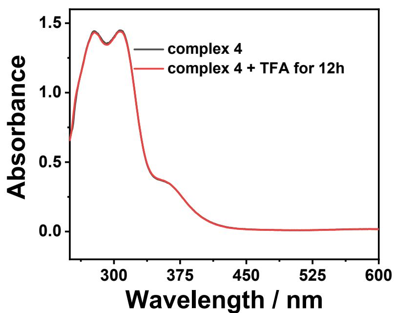
**Figure S33.** UV-Vis absorption spectra of 0.25 mM **4** in the presence of 5.38 mM TFA in MeCN.
