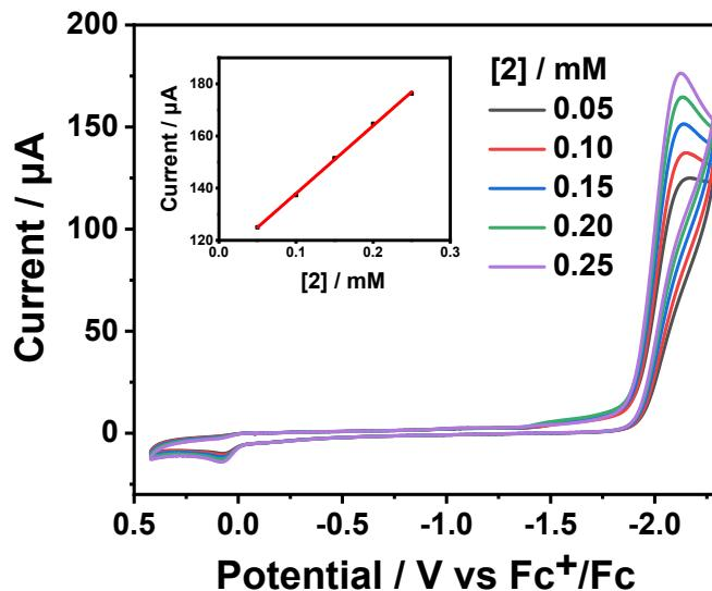
**Figure S22.** CVs of 0.05-0.25 mM **2** in DMF with 67.32 mM TFA at a scan rate of 100 mV s<sup>-1</sup> (0.1 M n-Bu<sub>4</sub>NPF<sub>6</sub> supporting electrolyte; glassy carbon working electrode). Insert: Plot of the  $i_{cat}$  against the complex **2** concentration.
