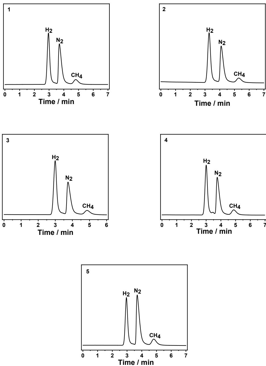
**Figure S38.** GC-TCD chromatograms of H<sub>2</sub> production of the controlled potential electrolysis of 0.25 mM **1 - 5** with 53.8 mM TFA in DMF over 18 h at a constant potential of -2.00 V, respectively.
