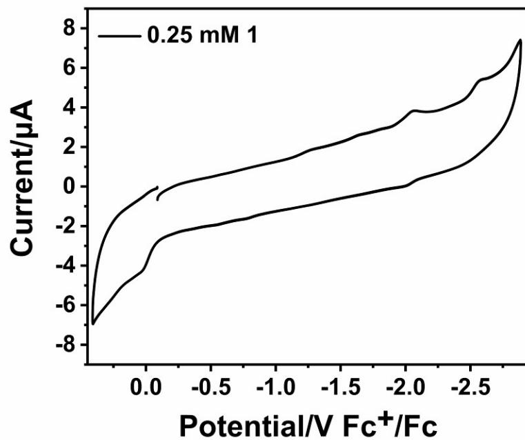
**Figure S11.** Cyclic voltammogram of 0.25 mM **1** recorded at 100 mV s<sup>-1</sup> scan rates in DMF solution with 0.1 M n-Bu<sub>4</sub>NPF<sub>6</sub> as the supporting electrolyte and using a glassy carbon working electrode.
