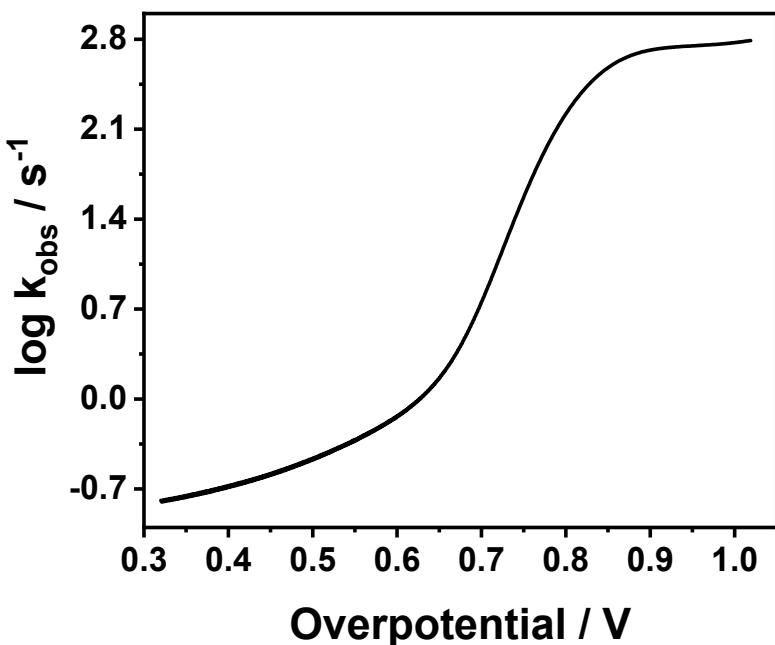
**Figure S28.** Plot of  $\log k_{\text{obs}}$  versus overpotential of 0.25 mM **4** in DMF in the presence of 67.32 mM TFA at a scan rate of 100 mV s<sup>-1</sup> (0.1 M n-Bu<sub>4</sub>NPF<sub>6</sub> supporting electrolyte; a glassy carbon working electrode).
