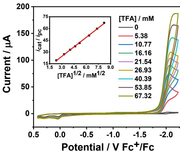
**Figure S16.** CVs of  $0.25 \text{ mM}$  **2** in DMF with different TFA concentrations ( $0, 5.38, 16.15, 21.54, 26.92, 40.39, 53.85$ , and  $67.32 \text{ mM}$ ) at a scan rate of  $100 \text{ mV s}^{-1}$  ( $0.1 \text{ M n-Bu}_4\text{NPF}_6$  supporting electrolyte; glassy carbon working electrode). Inset: Plot of the  $i_{\text{cat}}/i_{\text{pc}}$  against the square root of TFA concentration.
