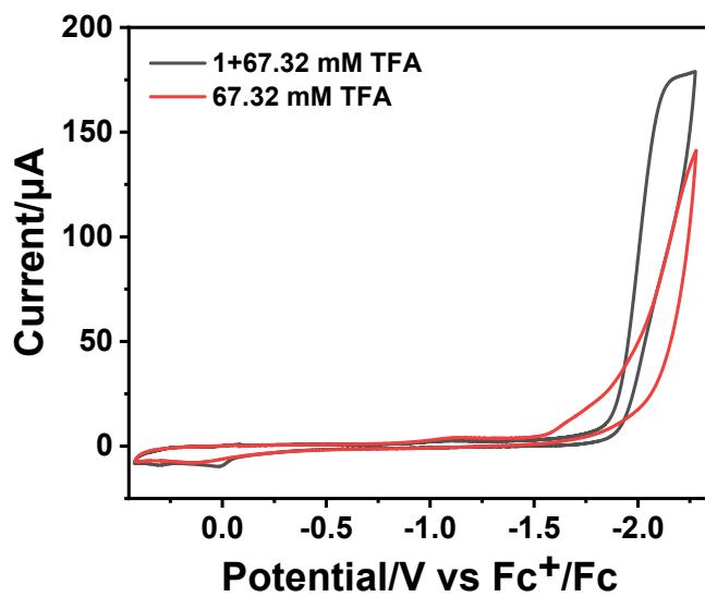
**Figure S21.** Red: Cyclic voltammogram of 67.32 mM TFA without **1** in DMF. Black: Cyclic voltammogram of 0.25 mM **1** with 67.32 mM TFA in DMF. Conditions: 0.1 M n-Bu<sub>4</sub>NPF<sub>6</sub> supporting electrolyte; glassy carbon working electrode; 100 mV s<sup>-1</sup> scan rate.
