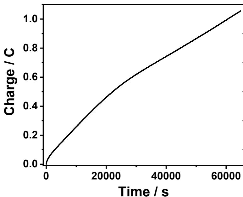
**Figure S37.** Cumulative coulombs in the presence of 53.8 mM TFA electrolysis for 18 h at a constant potential of -2.00 V (0.1 M n-Bu<sub>4</sub>NPF<sub>6</sub> supporting electrolyte; glassy carbon working electrode).
