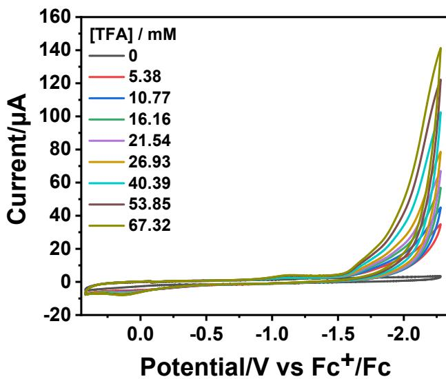
**Figure S20.** CVs of different TFA concentrations without complex in DMF (0, 5.38, 16.15, 21.54, 26.92, 40.39, 53.85, and 67.32 mM) at a scan rate of 100 mV s<sup>-1</sup> (0.1 M n-Bu<sub>4</sub>NPF<sub>6</sub> supporting electrolyte; glassy carbon working electrode). Inset: Plot of the  $i_{\text{cat}} / i_{\text{pc}}$  against the square root of TFA concentration.
