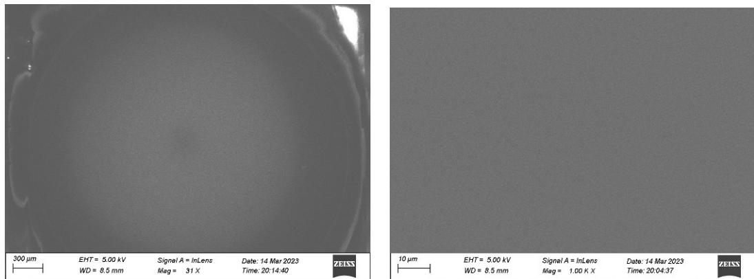
**Figure S43.** SEM images of the surface of the rinsed glassy carbon electrode after 18 hours of CPE testing at 0.25 mM 1 and 53.8 mM TFA.
