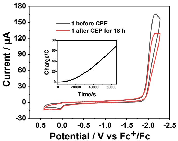
**Figure S45.** Cyclic voltammograms of 0.25 mM **1** with 53.8 mM TFA before and after CPE for 18 h (0.1 M n-Bu<sub>4</sub>NPF<sub>6</sub> supporting electrolyte; glassy carbon working electrode).
