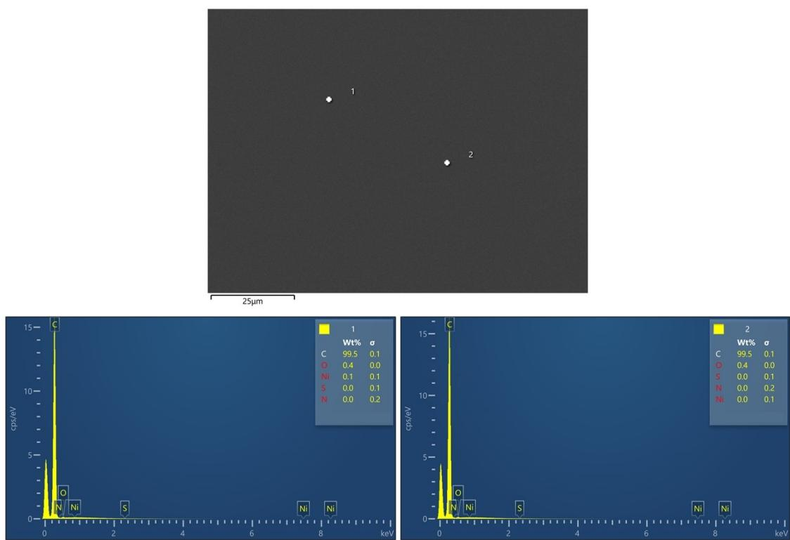
**Figure S44.** EDS diagrams of the surface of the rinsed glassy carbon electrode after 18 hours of CPE testing at 0.25 mM 1 and 53.8 mM TFA.
