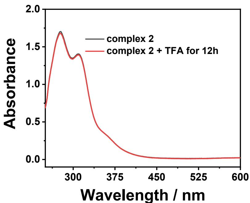
**Figure S31.** UV-Vis absorption spectra of 0.25 mM **2** in the presence of 5.38 mM TFA in MeCN.
