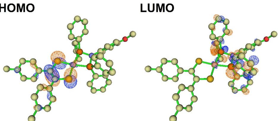
**Figure S47.** Electron density profiles of the highest occupied molecular orbital (HOMO) and lowest unoccupied molecular orbital (LUMO) of **2**.
