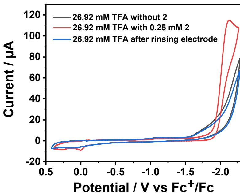
**Figure S35.** Cyclic voltammograms of **2** (0.25 mM) in DMF with 26.92 mM TFA (red) and a subsequent CV using the same electrode after rinsing and transfer to fresh in DMF of 26.92 mM TFA without adding **2** (blue). For comparison, CV of 26.92 mM TFA without **2** is shown in grey (0.1 M n-Bu<sub>4</sub>NPF<sub>6</sub> supporting electrolyte; glassy carbon working electrode; scan rate 100 mV s<sup>-1</sup>).
