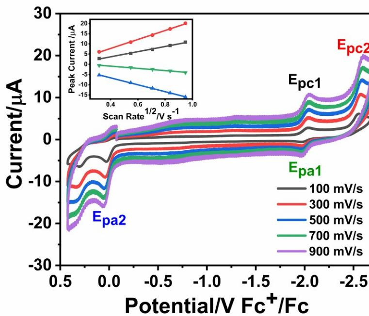
**Figure S12.** CVs of **2** recorded at scan rates from 100 mV s<sup>-1</sup> to 900 mV s<sup>-1</sup> in DMF solution with 0.1 M n-Bu<sub>4</sub>NPF<sub>6</sub> as the supporting electrolyte and using a glassy carbon working electrode. Inset: Plots of peak current versus the square root of scan rate.
