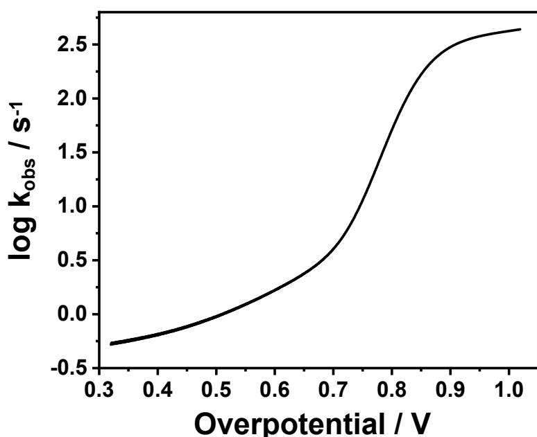
**Figure S29.** Plot of  $\log k_{\text{obs}}$  versus overpotential of 0.25 mM **5** in DMF in the presence of 67.32 mM TFA at a scan rate of 100 mV s<sup>-1</sup> (0.1 M n-Bu<sub>4</sub>NPF<sub>6</sub> supporting electrolyte; a glassy carbon working electrode).
