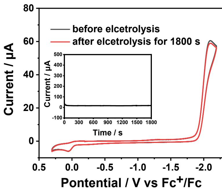
**Figure S41.** Cyclic voltammograms of 0.25 mM **4** with 26.93 mM TFA before and after electrolysis. Inset: Amperometric i-t curve spectra of **4** at a constant potential of -2.00 V. (0.1 M n-Bu<sub>4</sub>NPF<sub>6</sub> supporting electrolyte; glassy carbon working electrode; scan rate 100 mV s<sup>-1</sup>).
