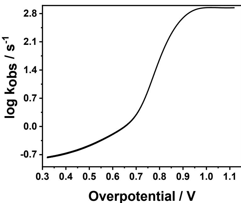
**Figure S27.** Plot of  $\log k_{\text{obs}}$  versus overpotential of 0.25 mM **3** in DMF in the presence of 67.32 mM TFA at a scan rate of 100 mV s<sup>-1</sup> (0.1 M n-Bu<sub>4</sub>NPF<sub>6</sub> supporting electrolyte; a glassy carbon working electrode).
