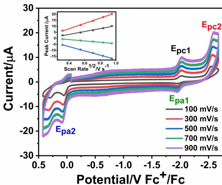
**Figure S13.** CVs of **3** recorded at scan rates from  $100 \text{ mV s}^{-1}$  to  $900 \text{ mV s}^{-1}$  in DMF solution with  $0.1 \text{ M}$  n-Bu<sub>4</sub>NPF<sub>6</sub> as the supporting electrolyte and using a glassy carbon working electrode. Inset: Plots of peak current versus the square root of scan rate.
