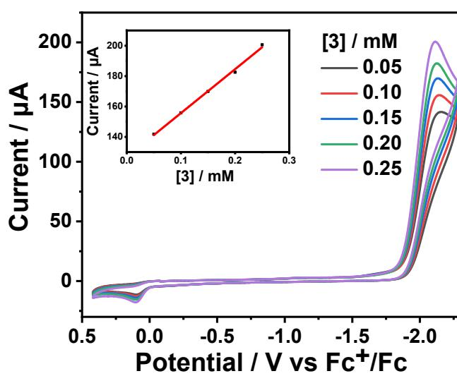
**Figure S23.** CVs of 0.05-0.25 mM **3** in DMF with 67.32 mM TFA at a scan rate of 100 mV s<sup>-1</sup> (0.1 M n-Bu<sub>4</sub>NPF<sub>6</sub> supporting electrolyte; glassy carbon working electrode). Insert: Plot of the  $i_{\text{cat}}$  against the complex **3** concentration.
