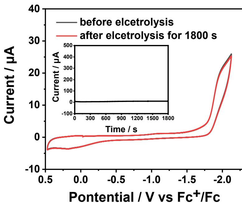
**Figure S42.** Cyclic voltammograms of 0.25 mM **5** with 26.93 mM TFA before and after electrolysis. Inset: Amperometric i-t curve spectra of **5** at a constant potential of -2.00 V. (0.1 M n-Bu<sub>4</sub>NPF<sub>6</sub> supporting electrolyte; glassy carbon working electrode; scan rate 100 mV s<sup>-1</sup>).
