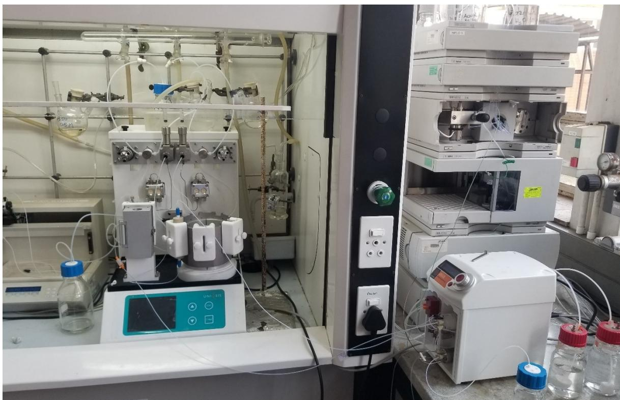
Figure S6. Photo of automated flow reactor.
