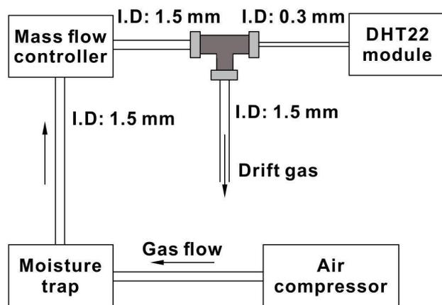
**Figure S2.** Schematic diagram showing gas flow in the portable IMS platform.
