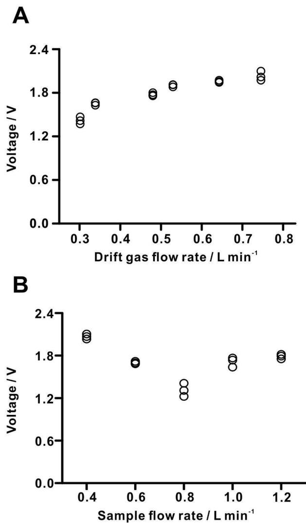
**Figure S6.** System optimization based on the dimer peak of 2,4-lutidine (drift time:  $10.23 \pm 0.01$ ,  $n = 3$ ); (A) Drift gas flow rate; (B) sample flow rate. Default values: sample flow rate,  $1.2 \text{ L min}^{-1}$ ; drift gas flow rate,  $0.746 \text{ L min}^{-1}$ .
