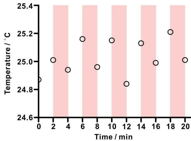
**Figure S4.** Temperature-time plot showing temperature variations around the drift tube. High voltage was always on. White part: cleaning fan and cooling fan were off. Pink part: cleaning fan and cooling fan were on (2-min interval).
