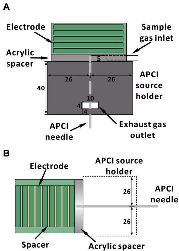
Figure S1. Schematic of the modified APCI source: (A) top-view; (B) side-view. Unit: mm
