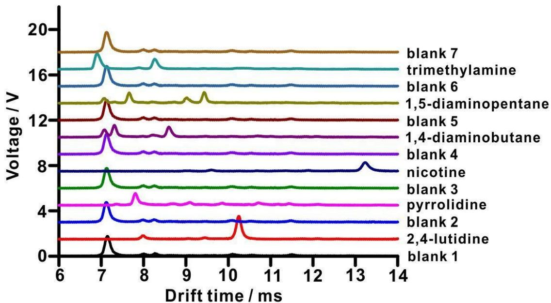
**Figure S7.** Verification of carryover using the spectra recorded to produce the PCA result shown in **Figure 4**. The amounts of analytes: 30 nmol 2,4-lutidine; 200 nmol pyrrolidine; 600 nmol nicotine; 80 nmol 1,4-diaminobutane; 600 nmol 1,5-diaminopentane; 200 nmol trimethylamine.
