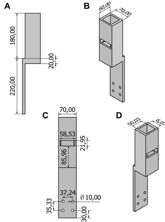
**Figure S3.** Technical drawing of the GPS module holder: (A) left side view; (B) side view; (C) front view; (D) side view. Unit: mm.
