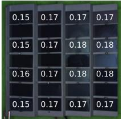
Figure S4. Exemplary light intensity calibration result of MIT Gen. 1 chamber. Intensities shown as Suns experienced by MAPbI 3 solar cells.
