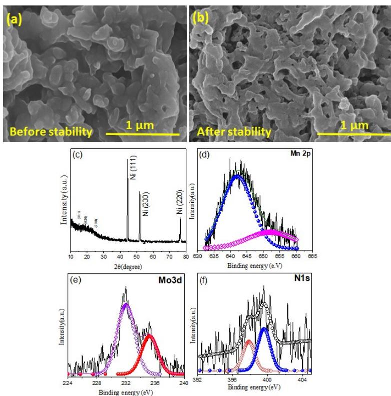
**Fig. S4.** SEM image's view of the PM-10 electrode (a) before and (b) after stability testing for 100 h in a 1M KOH solution. (c) XRD patterns, (d), (e) and (f) XPS spectra after stability.
