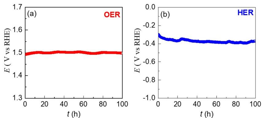
**Fig. S3.** Long term durability test: (a), (b) chronopotentiometry curves of PM-10 for OER and HER test at a constant current density of  $30 \text{ mAcm}^{-2}$  and  $-10 \text{ mAcm}^{-2}$ , respectively.
