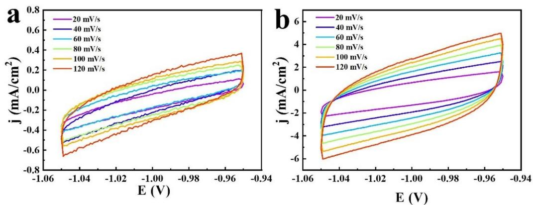
**Fig. S7** CV curves of (a) TF-NS/NF and (b) CS-NS/NF at different scan rates.
