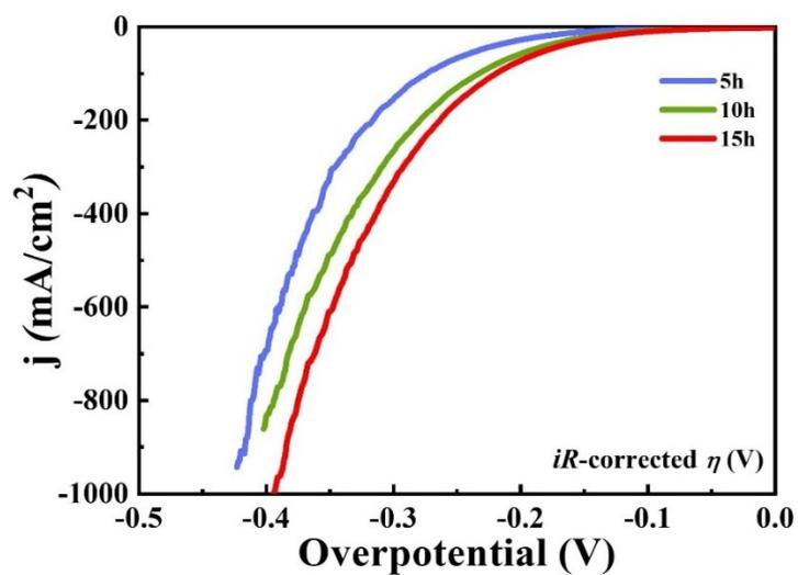
**Fig. S6** HER LSV curves obtained from control experiments under the different reaction time.
