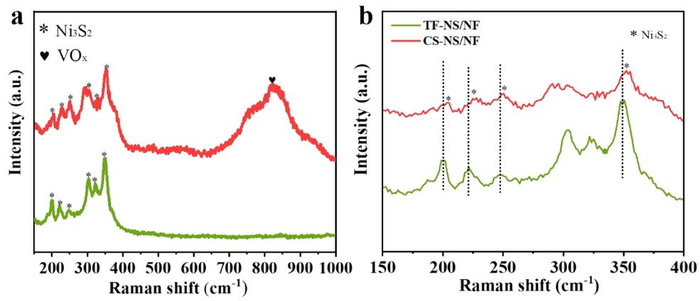
**Fig. S1** (a) Raman spectra and (b) local magnification of CS-NC/NF and TF-NS/NF.
