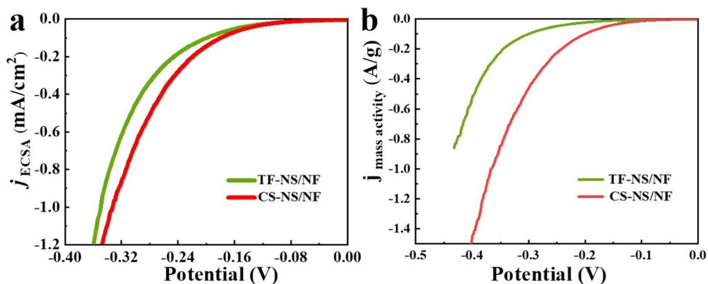
**Fig. S8** (a)HER ECSA-normalized LSV curves of CS-NS/NF and TF-NS/NF. (b) The mass normalized current density of two catalysts.
