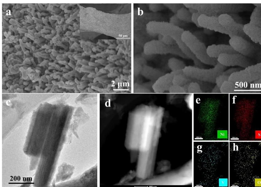
**Fig. S9** (a, b) SEM images; (c) TEM image; (d) The STEM image and (e-h) EDS elemental mapping images Ni, V, O and S of the CS-NS/NF electrode after the HER stability test.
