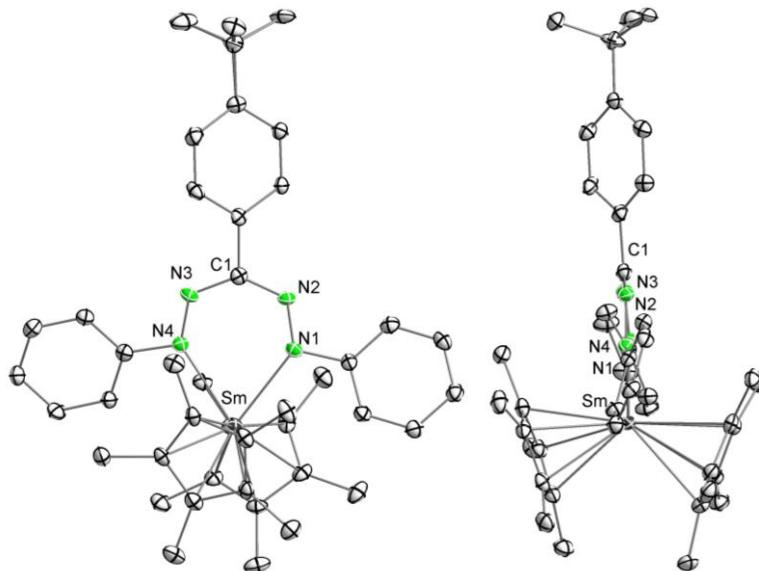
**Fig. S23** Molecular structure of **4** in the solid state with thermal ellipsoids at the 30% probability level (left-front view; right-side view). All hydrogen atoms are omitted for clarity. Selected bond lengths ( $\text{\AA}$ ) and bond angles [ $^\circ$ ]: Sm-N1 2.489(4), Sm-N4 2.475(5), N1-N2 1.306(6), N2-C1 1.335(7), N3-N4 1.290(6), N3-C1 1.349(7); N1-Sm-N4 72.15(15), N2-N1-Sm 133.3(4), N1-N2-C1 122.7(5), N4-N3-C1 122.3(5), N3-N4-Sm 134.3(4), N2-C1-N3 134.6(5).
