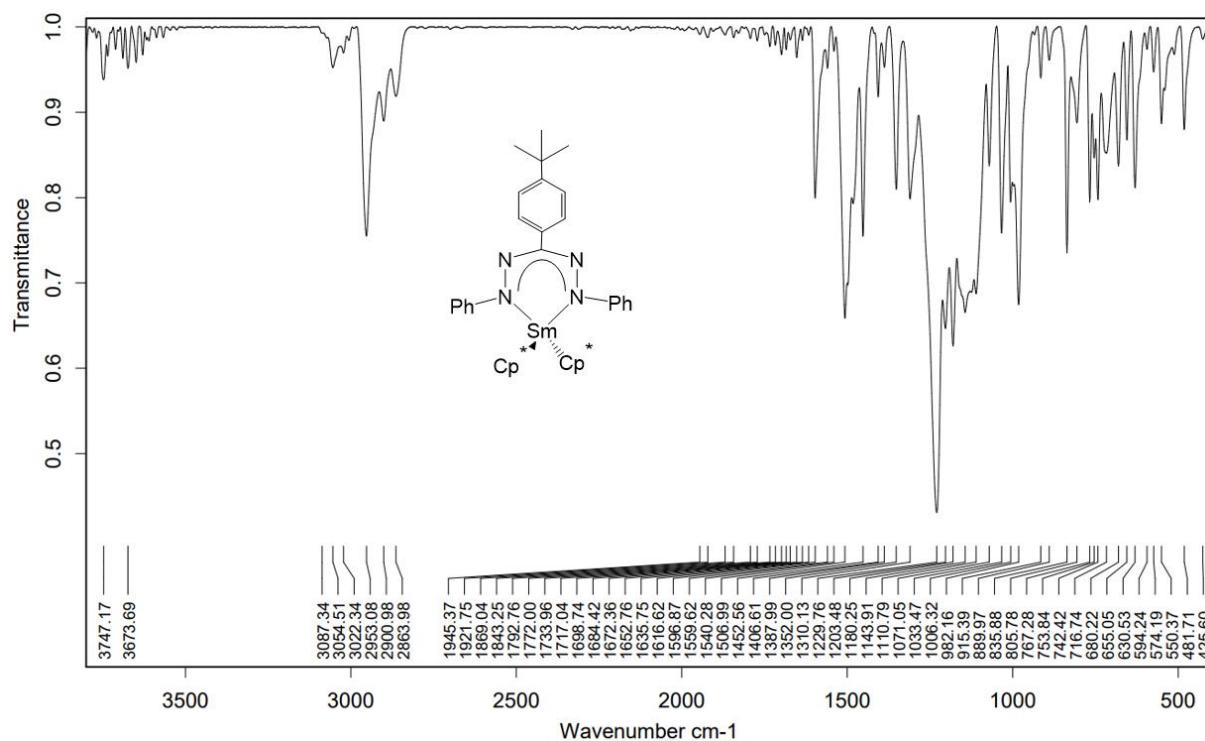
**Fig. S15** IR spectrum of [{PhNNC(4-*t*BuPh)NNPh}SmCp\*] (**4**).
