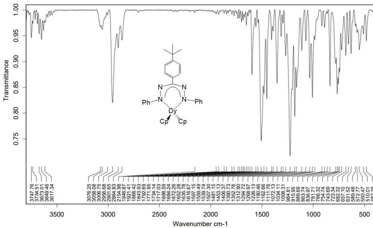
**Fig. S16** IR spectrum of [{PhNNC(4-*t*BuPh)NNPh}DyCp<sub>2</sub>] (**5**).
