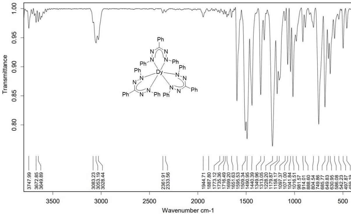
**Fig. S14** IR spectrum of  $[PhNNC(Ph)NNPh]_3Dy$  (**3**).
