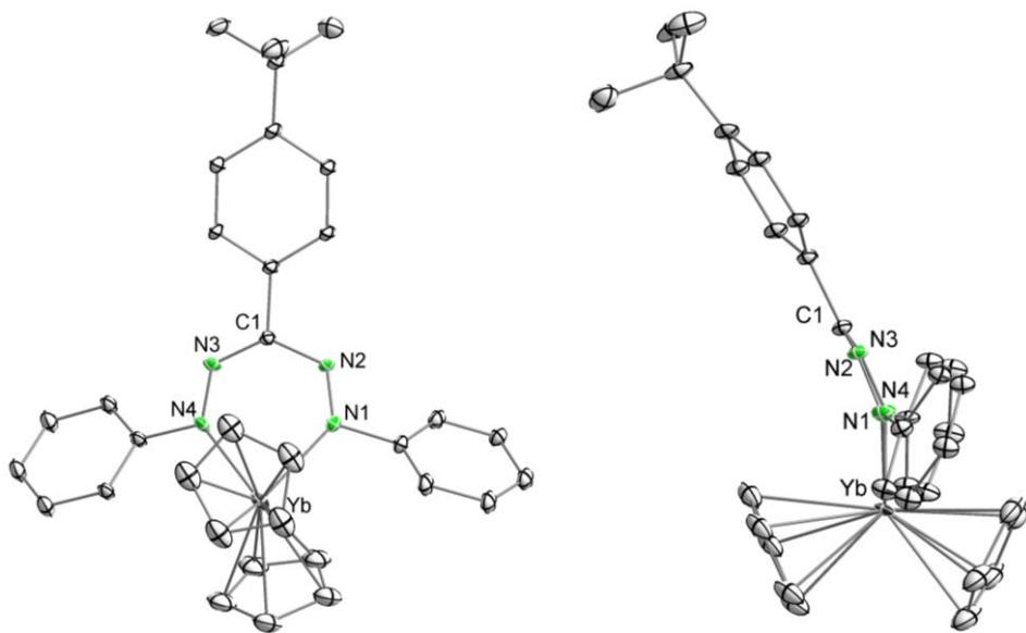
**Fig. S25** Molecular structure of **6** in the solid state with thermal ellipsoids at the 25% probability level (left-front view; right-side view). All hydrogen atoms are omitted for clarity. Selected bond lengths ( $\text{\AA}$ ) and bond angles [ $^\circ$ ]: Yb-N1 2.37(2), Yb-N4 2.335(15), N1-N2 1.26(3), C1-N2 1.39(3), N3-C1 1.31(3), N3-N4 1.29(2); N1-Yb-N4 73.8(7), N2-N1-Yb 130.4(15), N1-N2-C1 122(2), N4-N3-C1 124(2), N3-N4-Yb 129.5(13), N3-C1-N2 130(2).
