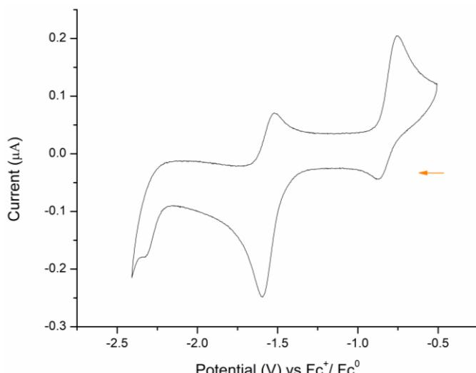
**Fig. S19** Cyclic voltammogram of  $\text{L}^2\text{H}$  (THF, 0.1 M  $[\text{Bu}_4\text{N}] [\text{PF}_6]$ ) recorded at  $250 \text{ mVs}^{-1}$
