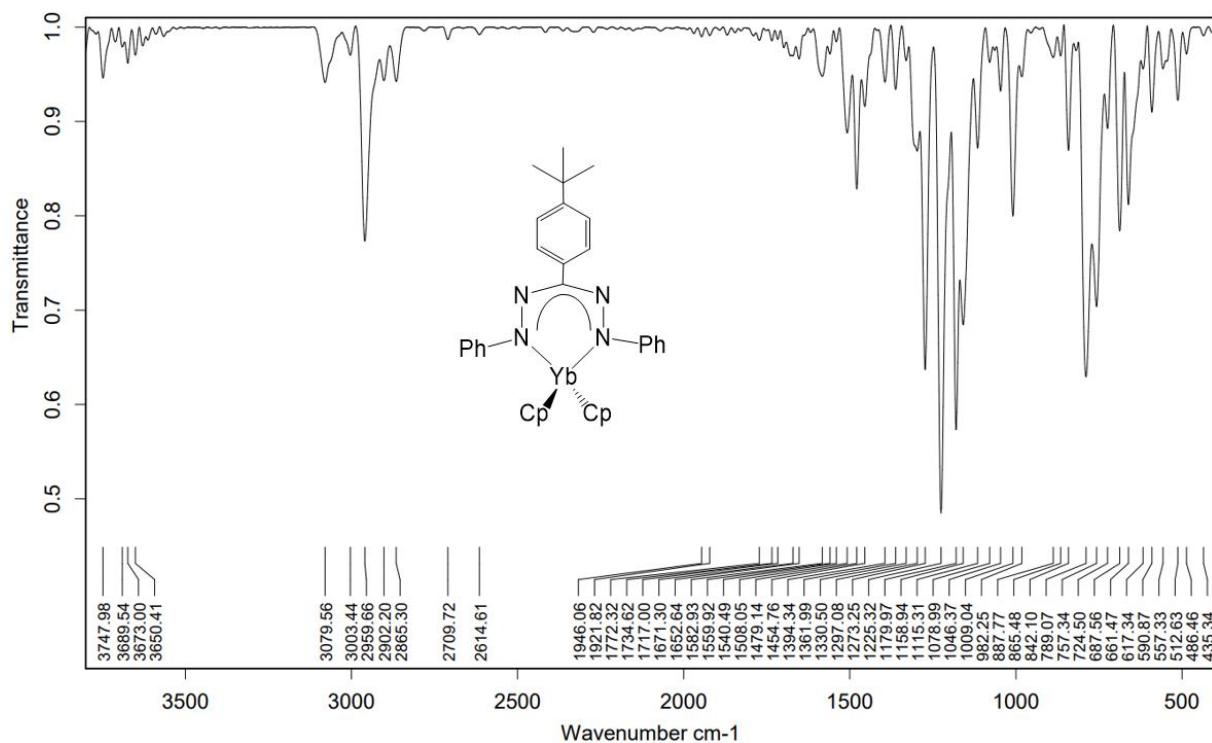
**Fig. S17** IR spectrum of  $\text{[}\{\text{PhNNC(4-tBuPh)NNPh}\}\text{YbCp}_2\text{]}$  (**6**).
