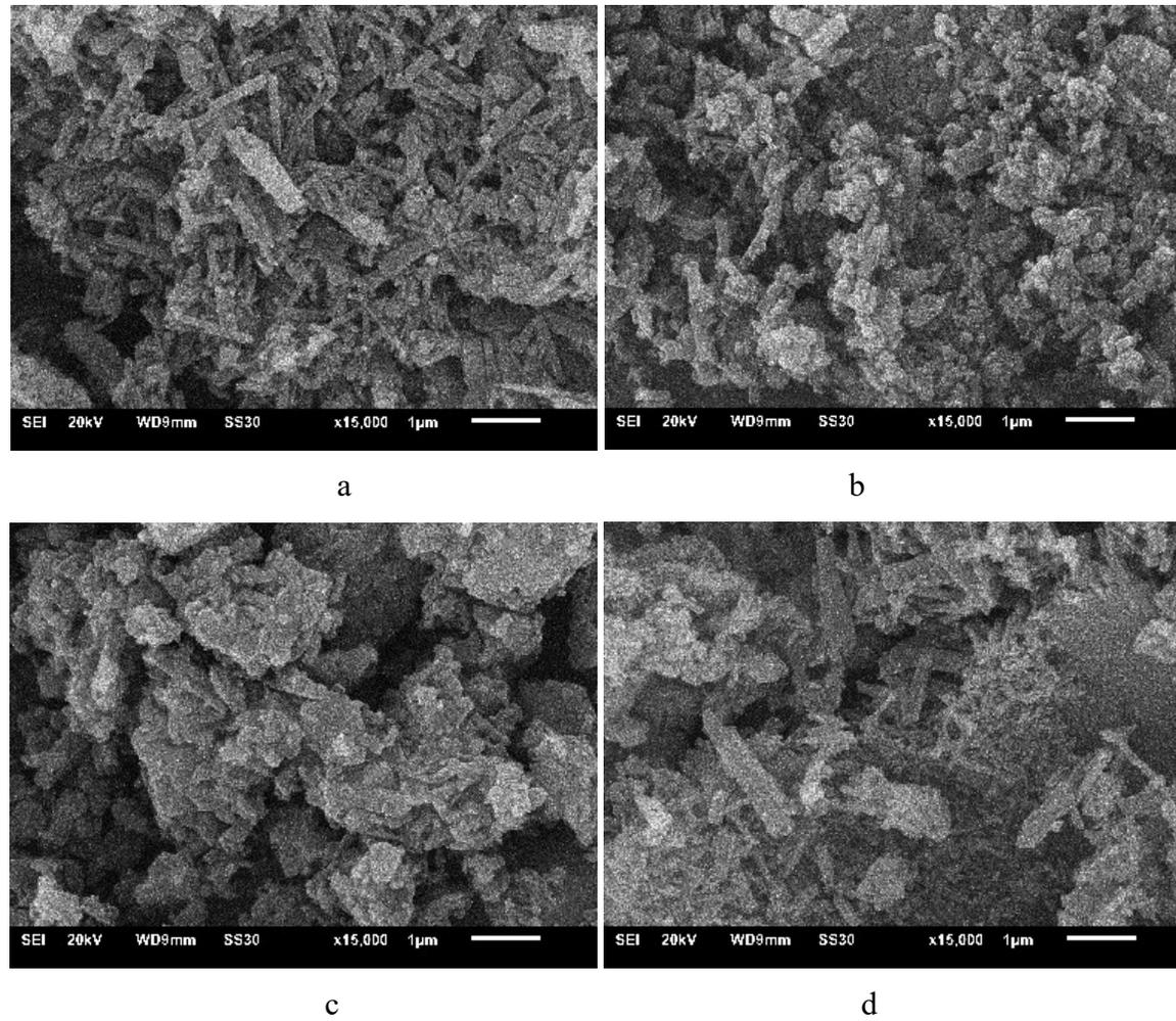
**Fig. S4.** SEM images of MOF MIL-53-TDC modified with PE: PAA (a), CMC (b), DexS (c), CAR (d).
