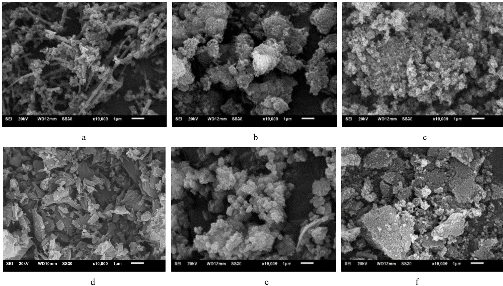
**Fig. S3.** SEM images of the neat MOFs: MIL-101(Cr) (a), Al-fum (b), Basolite® A520 (c), MIL-53-TDC (d), UiO-66 (e), Zr-fum (fe).
