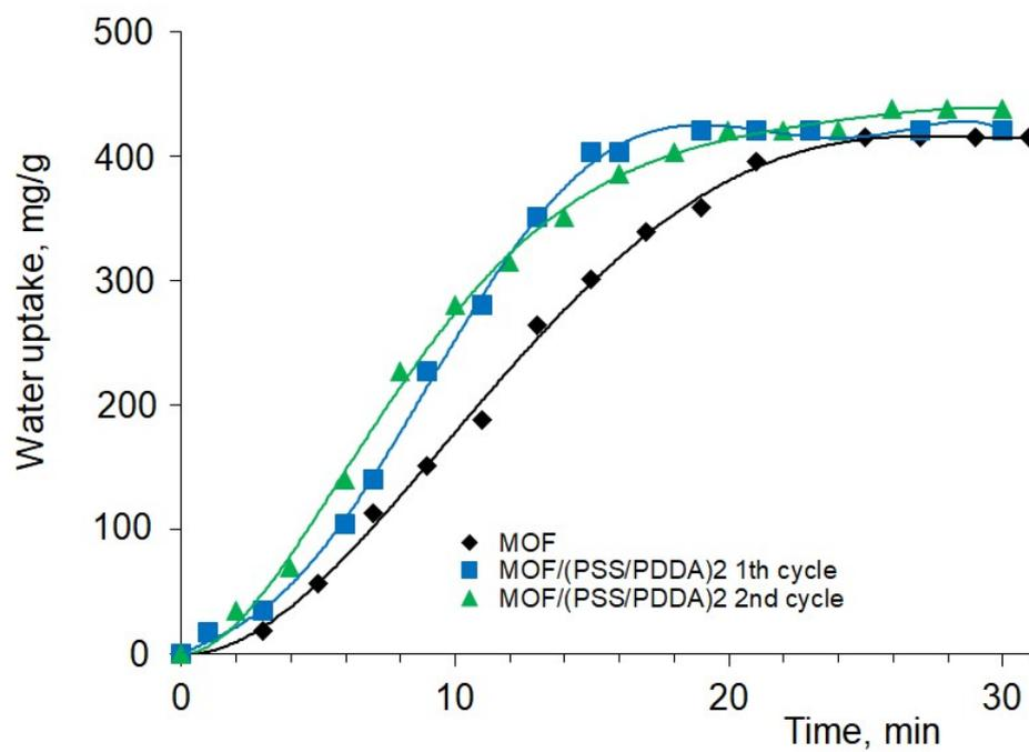
**Fig. S14.** Water vapor uptake by Al fumarate and Al fumarate / thick (PSS/PDDA)<sub>2</sub> shell composite (23 °C, RH 70%).
