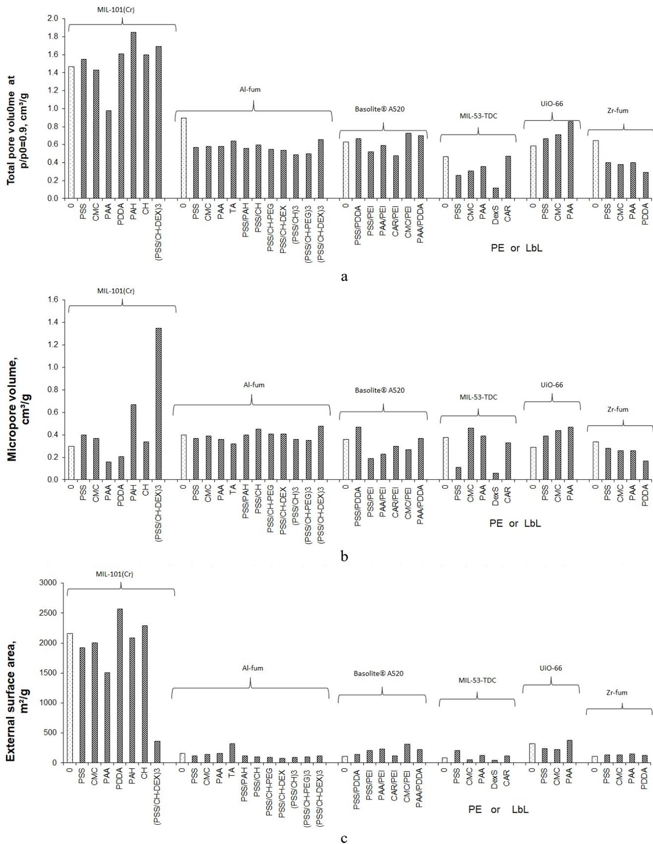
**Fig. S10.** Total pore volume (a), micropore volume (b), and external surface area (c) of the MOFs after single polyelectrolyte modification as evaluated by nitrogen sorption.
