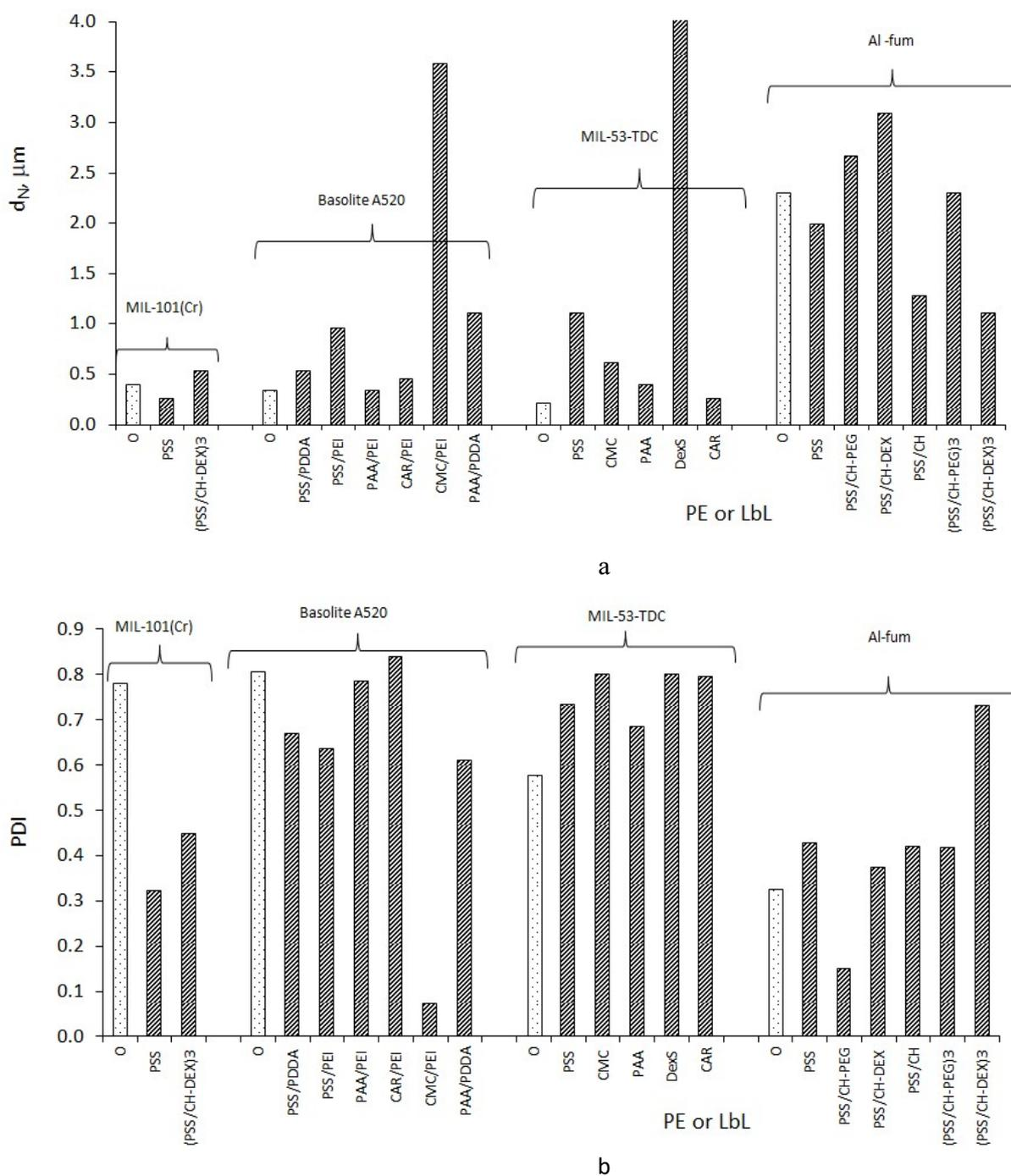
**Fig. S5.** Hydrodynamic diameter ( $d_N$ ) (a) and polydispersity index (PDI) (b) of MOF powders coated with a single polyelectrolyte layer or a LbL shell as indicated on the X-axis, determined by DLS in a water dispersion.
