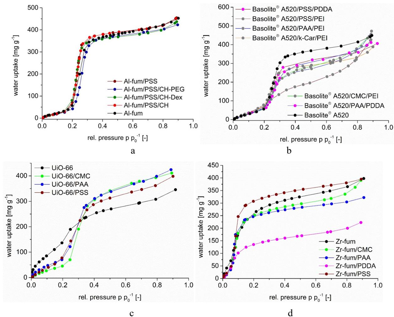
**Fig. S11.** Isotherms of water vapor sorption by MOF/PE and MOF/LbL composites: a) Al-fum, b), Basolite®A520, c) UiO-66, d) Zr-fum.
