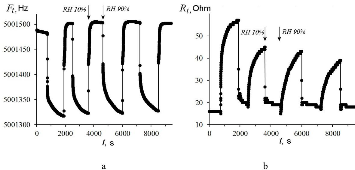
**Fig. S12.** Changes of  $F_t$  (a) and  $R_t$  (b) of a 5 MHz resonator with Al-fum/(PSS/PDDA)<sub>3</sub> deposit in the process of alternately changing humidity.  $T = 25.4$  °C.
