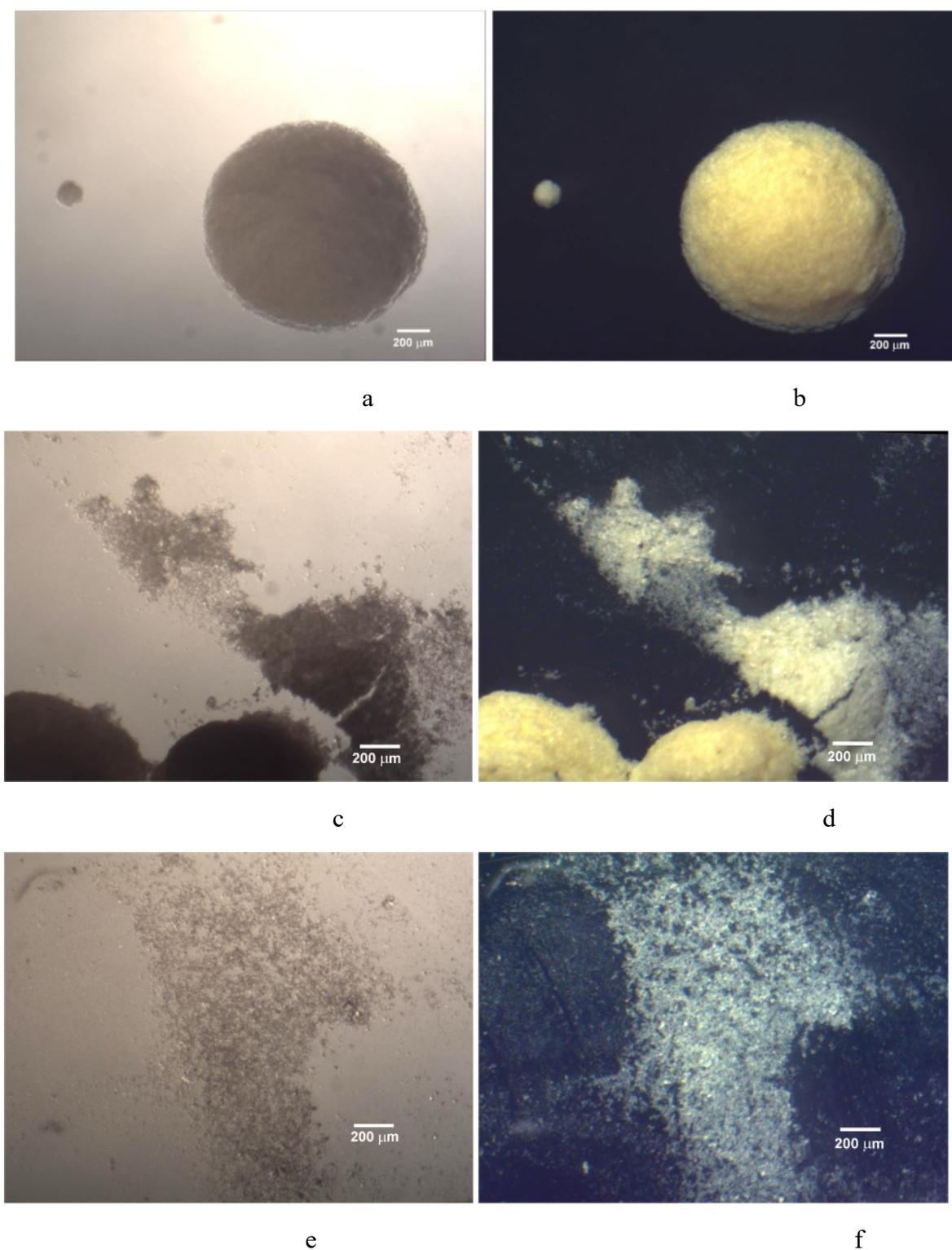
**Fig. S8.** Micrographs of dry Al fumarate microparticles coated with a  $(\text{PSS}/\text{PAH-FITC})_2$  shell of different degree of agglomeration obtained in transmitted (a,c,e) and reflected (b,d,f) light. Yellow color shows the distribution of LbL shell containing FITC-labeled PAH 15 kDa.  $T=25\text{ }^\circ\text{C}$ . The images were taken using a LOMO MSP-1 option 5 stereoscopic microscope equipped with a TCA-5.0C camera.
