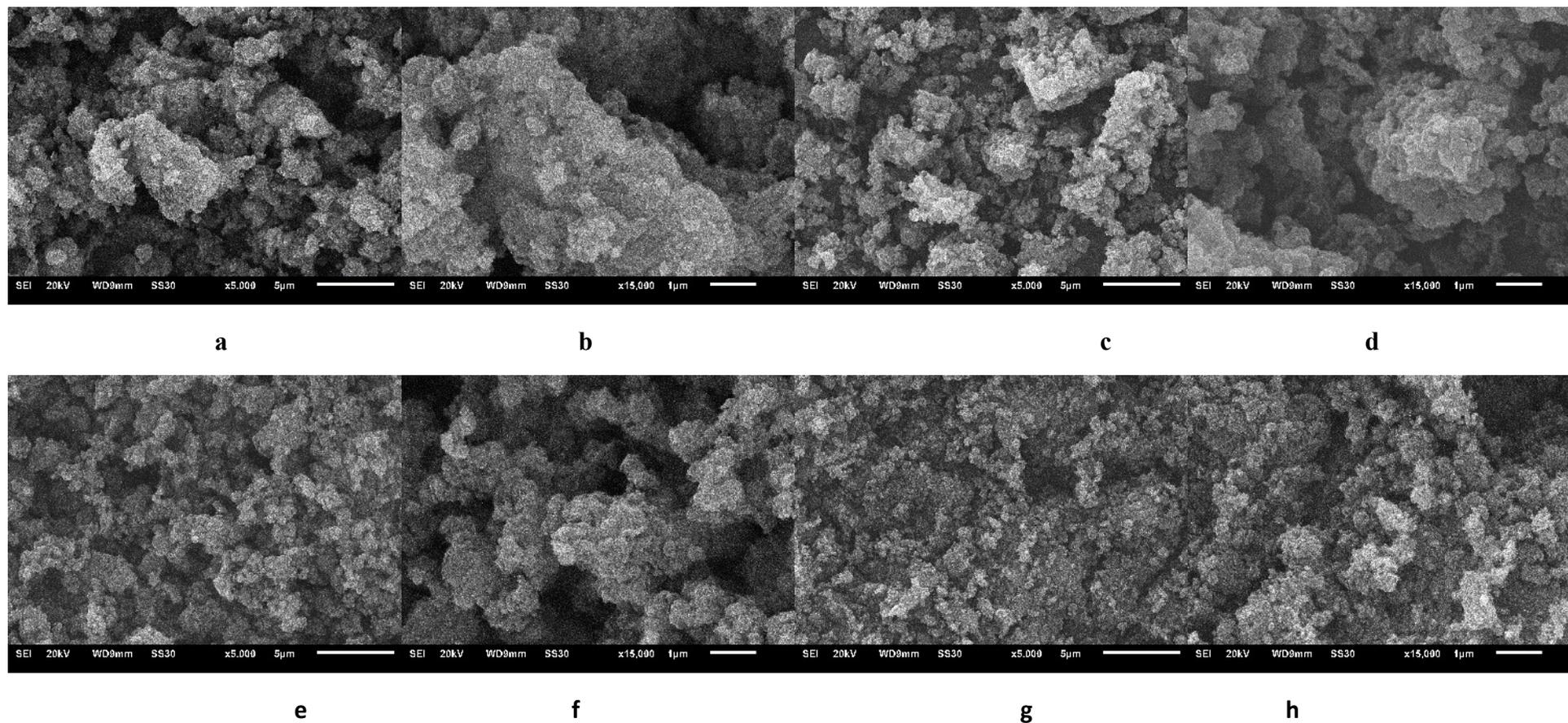
**Fig. S7.** SEM images of MOF Basolite<sup>®</sup> A520 modified with a LbL shell of PSS/PDDA (a,b), CMC/PEI (c,d), PAA/PDDA (e,f), PAA/PEI (g,h).
