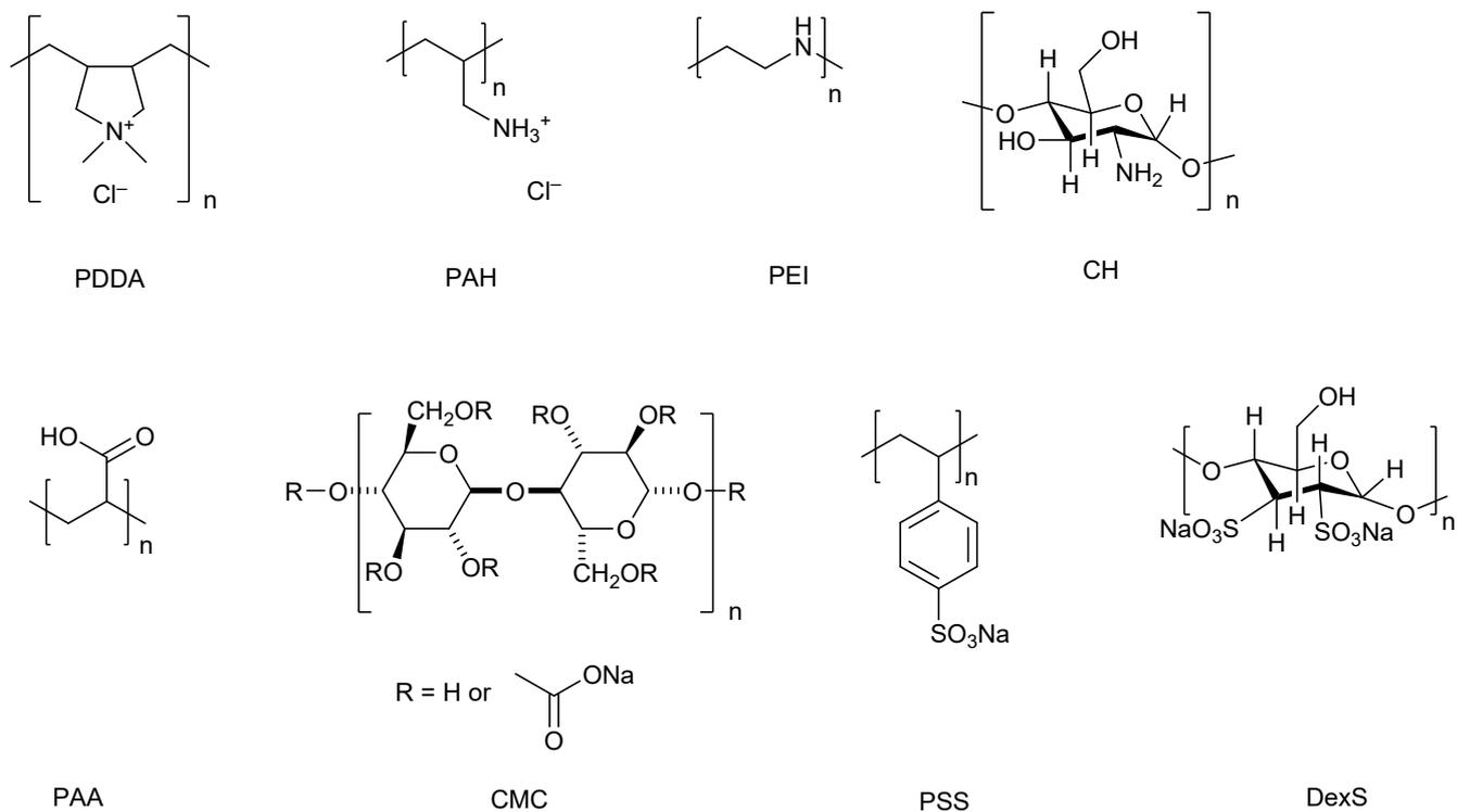
**Fig. S1. Structure of the used polyelectrolytes :** poly(diallyldimethylammonium chloride) (PDDA), polyallylamine hydrochloride (PAH), polyethyleneimine (PEI), and chitosan (CH), polyacrylic (PAA), carboxymethyl cellulose (CMC), polystyrene sulfonic acid sodium salt (PSS), dextran sulfate (DexS).
