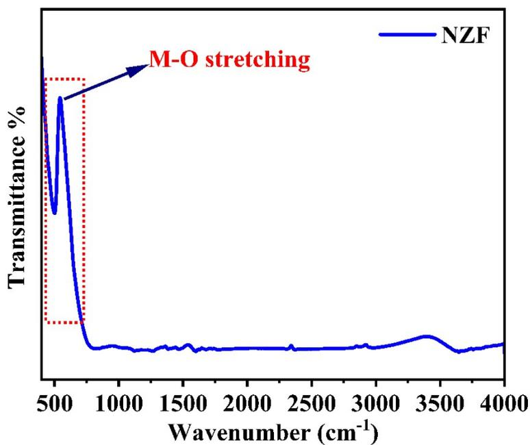
**Fig. S5** FTIR of the pure NZF material.<sup>1</sup>
