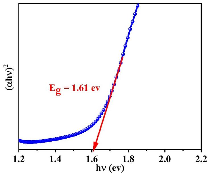
**Fig. S6** Tauc plot for the optical bandgap of the NZF-PANI nanohybrids
