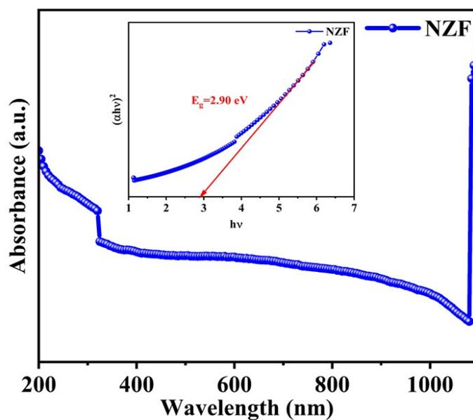
**Fig. S7** UV-visible spectroscopy of the pure nickel zinc iron oxide and tauc plot in the inset image.
