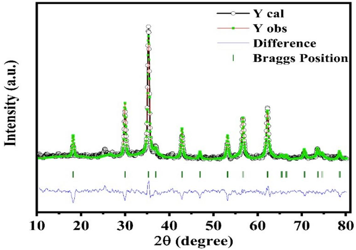
Fig. S1 Reitveld refinement of pure nickel zinc iron oxide (NZF) nanomaterial.
