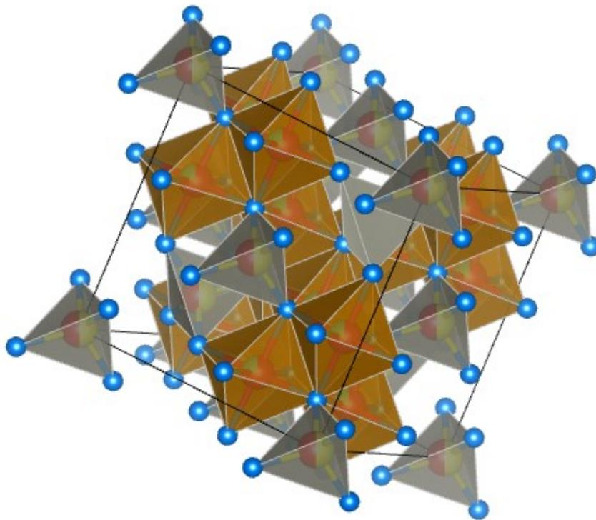
Fig. S2 Crystal structure of the nickel zinc iron oxide from the reitveld refinement.
