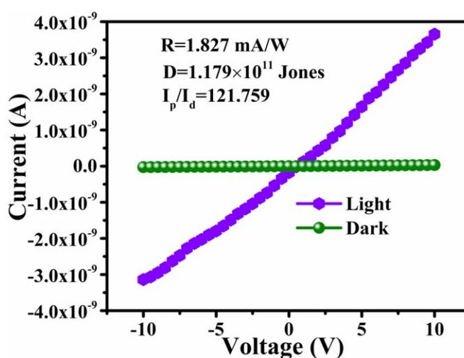
**Fig. S8** I-V characteristics of the NZF under dark and light conditions.
