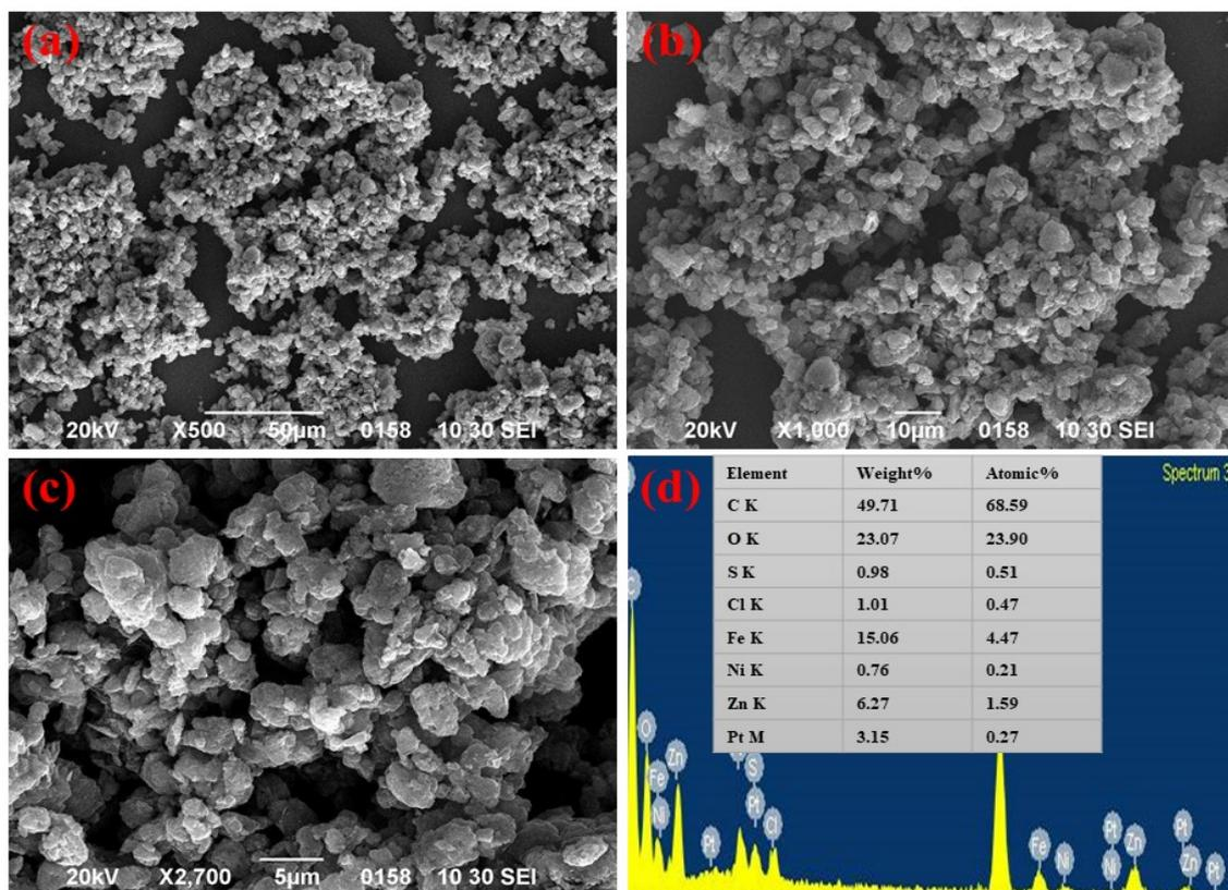
**Fig. S3** SEM micrographs at different magnifications (a), (b) and (c); (d) EDS spectrum of the NZF/PANI hybrid material and their elemental composition.
