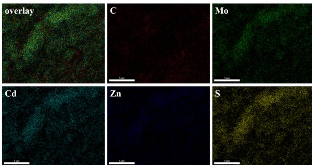
Fig. S2 SEM-mapping images of overlay, C, Mo, Cd, Zn and S in 2-MMC/ZCS.
