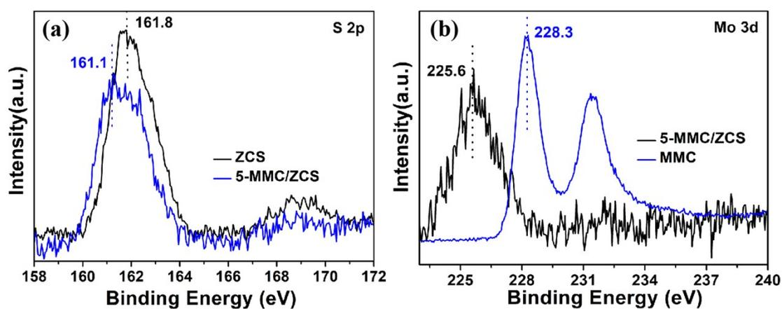
**Fig. S4** (a) S 2p in the prepared ZCS and 5-MMC/ZCS sample, (b) Mo 3d in the prepared MMC and 5-MMC/ZCS sample.
