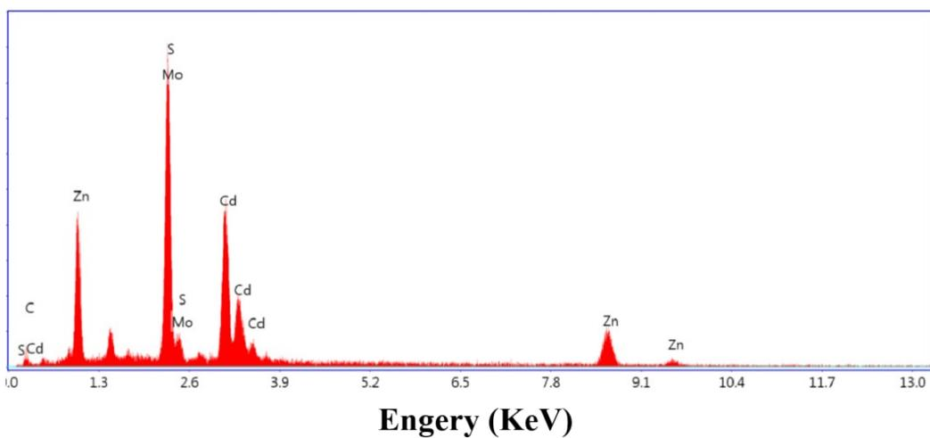
**Fig. S3** EDS spectra of 2-MMC/ZCS sample
