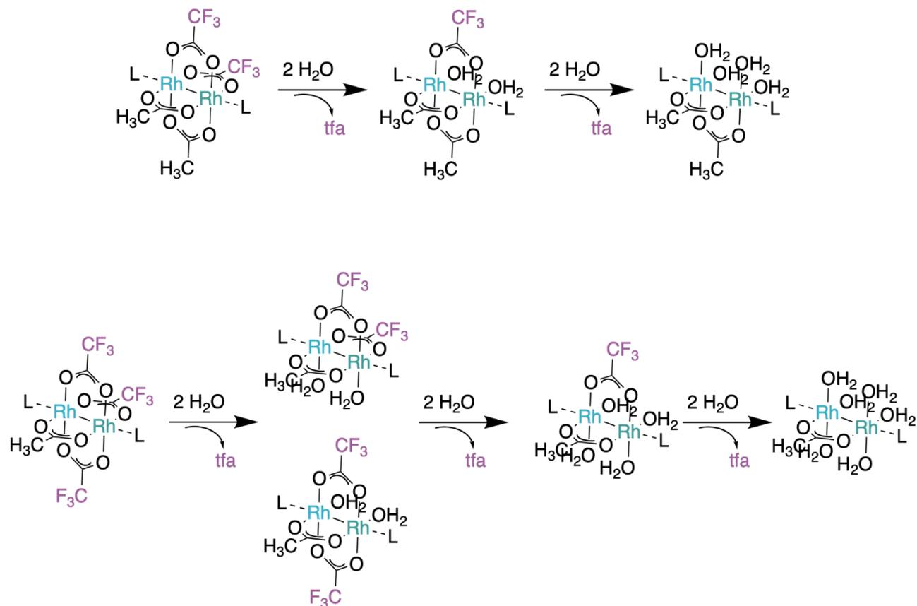
**Scheme S2.** Hydrolytic pathway of  $[cis\text{-Rh}_2(\text{OAc})_2(\text{tfa})_2]$  and  $[\text{Rh}_2(\text{OAc})(\text{tfa})_3]$ .
