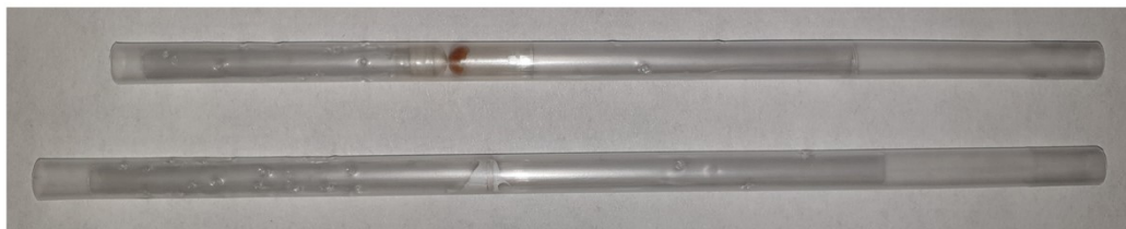
Figure S 1: Preparation of the samples. Top: compound in eicosan-matrix in plastic capsule. Bottom: compound ground and pressed into a pellet.
