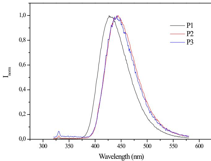
**Figure S22.** Emission spectra of phosphanes **P1-3**.
