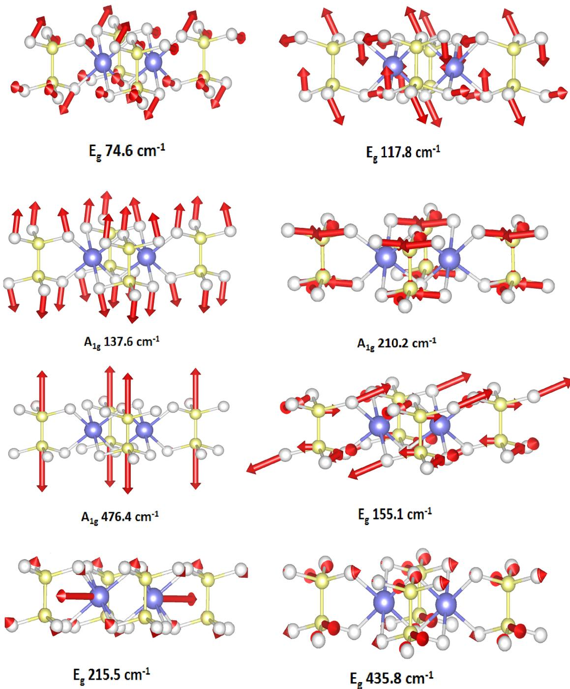
**Figure S3:** Vibrational eigenvectors of the zone-centered Raman phonon modes shown in the low dimensional MgPSe<sub>3</sub> structure. The light blue, white, and yellow balls represent Mg, Se, and P atoms, respectively.
