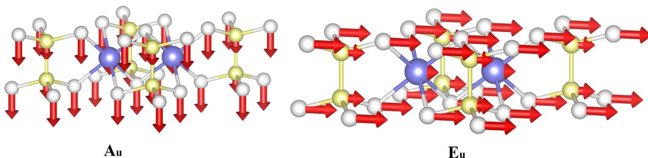
**Figure S1** : Vibrational eigenvectors of the zone-centered acoustic phonon modes shown in the low dimensional MgPSe<sub>3</sub> structure. The light blue, white, and yellow balls represent Mg, Se, and P atoms, respectively.
