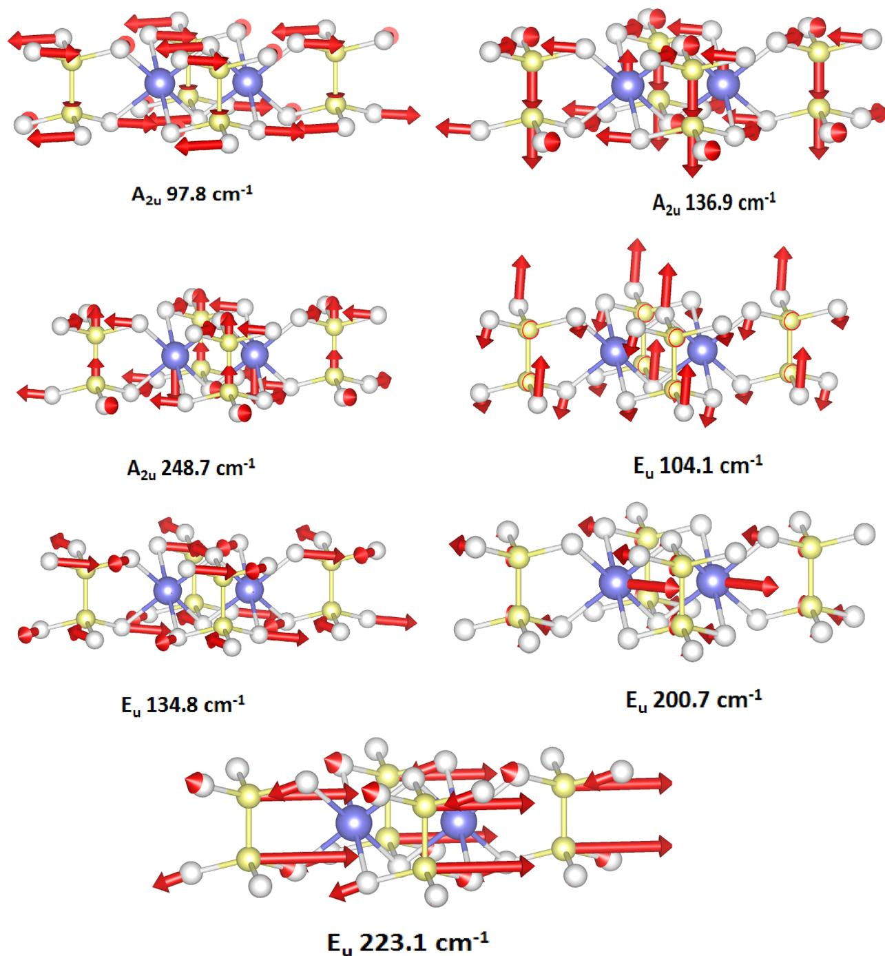
**Figure S4:** Vibrational eigenvectors of the zone-centered Infrared phonon modes shown in the low dimensional MgPSe<sub>3</sub> structure. The light blue, white, and yellow balls represent Mg, Se, and P atoms, respectively.
