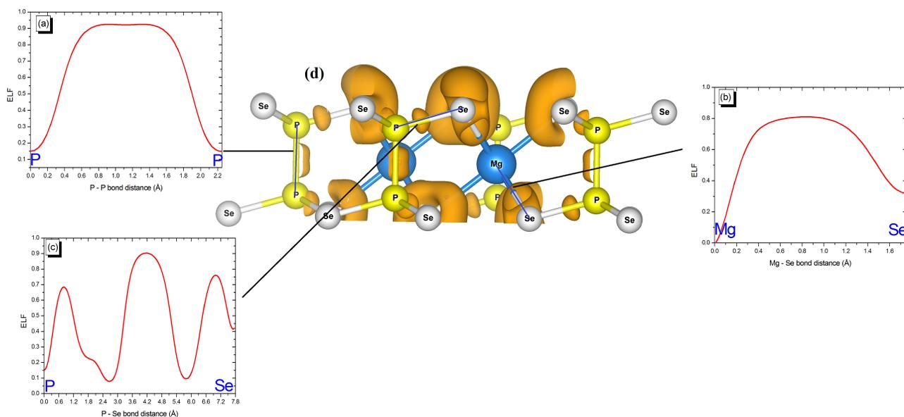
**Figure S5:** 1D ELF profile analyzed for the (a) P–P, (b) Mg–Se and (c) P–Se bonds. The plot in (d) depicts 3D ELF isosurface for  $\eta=0.84$ . The profile near the P and Se in (c) represents only the shadow of the other bonds' directions. It is noted that due to the fact that our work is done within the PAW method, only valence electrons are taken into account in the calculation, and for this reason, we have a zero value in the ELF profile in the core of the atoms.
