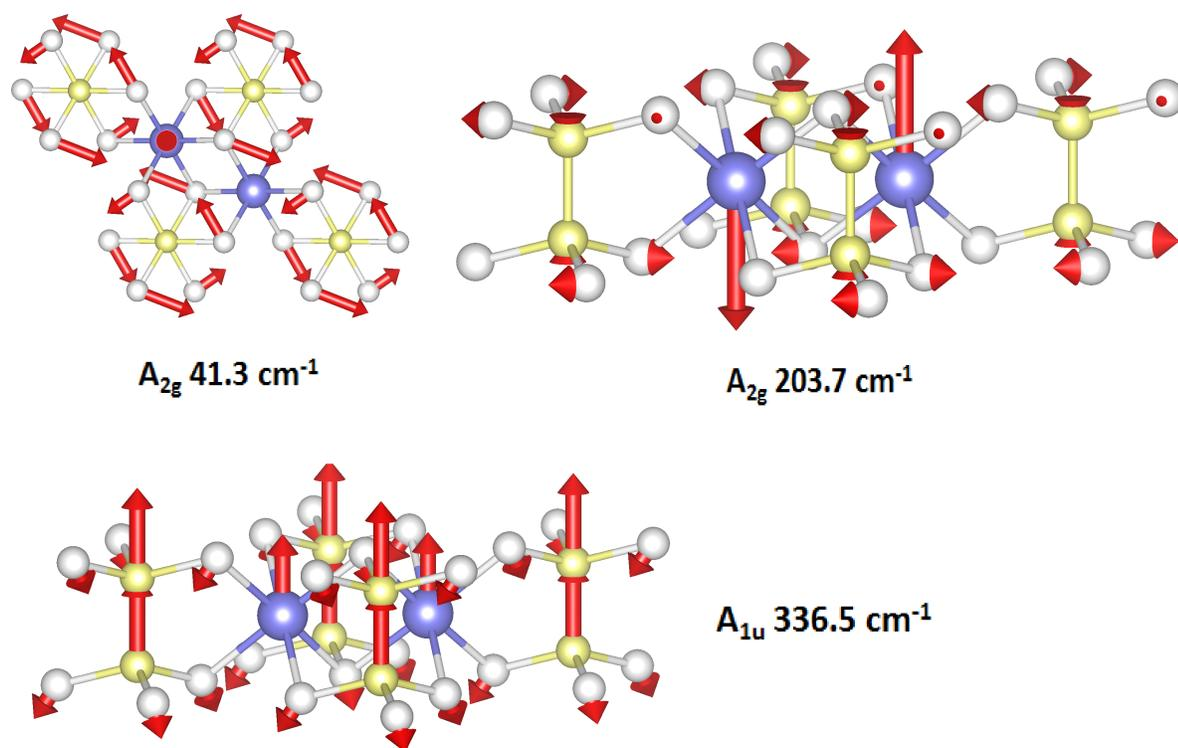
**Figure S2**: Vibrational eigenvectors of the zone-centered silent phonon modes shown in the low dimensional MgPSe<sub>3</sub> structure. The light blue, white, and yellow balls represent Mg, Se, and P atoms, respectively.
