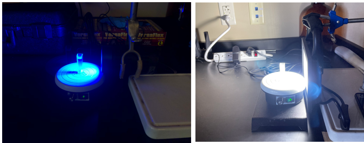
Figure S3. Photolysis setup used to study photoinduced ligand ejection processes from complexes. The samples were dissolved in 3 mL of deionized water and illuminated with a (left) Kessil PR160 lamp (467 nm, 120 \text{mW}/\text{cm}^2 at 5 cm) or (right) GLORIOUS-LITE 30W LED (240W halogen equivalent), 3000 LM broad spectrum white light that was held 5 cm away from the sample with constant stirring.
