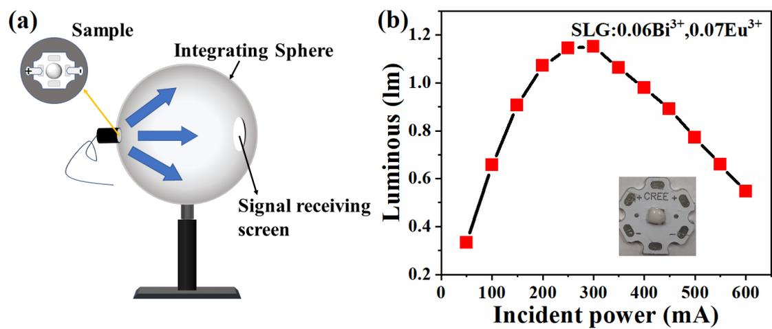
**Figure S5.** (a) Illustration of the irradiance measurement device of the luminous flux tester; (b) The luminous flux variation curve of WLED3 (320 nm UV chip + SLG:0.06Bi<sup>3+</sup>,0.07Eu<sup>3+</sup> sample) under different input currents.
