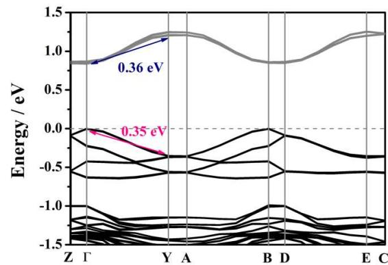
**Fig. S9** Band structure of **CdCl-ONDI** marked with dispersion width value.
