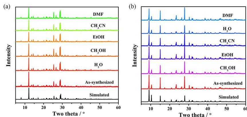
**Fig. S17** PXRD patterns of **Mn-ONDI-1** (a) and **CdCl-ONDI** (b) after immersion in different solvents for 3 days. From their PXRD patterns, **Mn-ONDI-1** and **CdCl-ONDI** both exhibited high stability in common solvents, which could be assigned to strong metal-hydroxamate bonds.<sup>1</sup>
