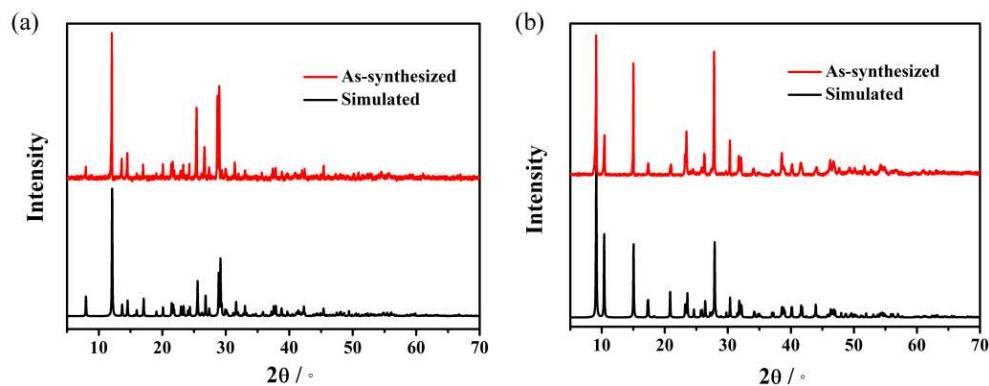
**Fig. S12** PXRD patterns of **Mn-ONDI-1** (a) and **CdCl-ONDI** (b);  $\lambda(\text{Cu-K}_{\alpha 1}) = 1.54060 \text{ \AA}$ .
