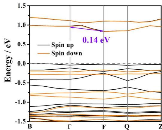
**Fig. S7** Band structure of **Mn-ONDI-1** marked with dispersion width value.
