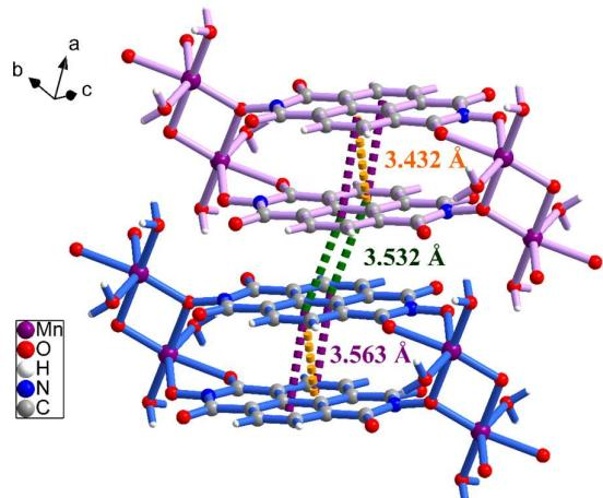
**Fig. S2**  $\pi-\pi$  interactions in **Mn-ONDI-1**; same colour as in **Fig. 2**; dashed lines represent equivalent centroid–centroid distances.
