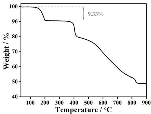
**Fig. S14** TG curve of **Mn-ONDI-1**. The weight loss of 9.33% at 150-200 °C corresponds to the loss of coordinated H<sub>2</sub>O molecules (calculated weight loss 9.30%).
