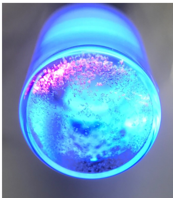
Figure S1. Top: Picture of \text{K}_5\text{Na}[\text{Eu}_2(\text{SO}_4)_6] crystals through a microscope lens. Bottom: Picture of \text{K}_5\text{Na}[\text{Eu}_2(\text{SO}_4)_6] crystals excited with a 405 nm laser pen.
