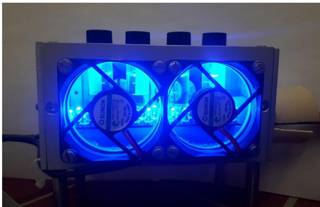
Figure S3. Custom-made microreactor equipped with four air ventilation units and one LED-stick irradiating the samples from the bottom of the GC vial utilized as reaction vessel ( \lambda = 470 \pm 20 nm, 45 \pm 5 W cm -1 ).
