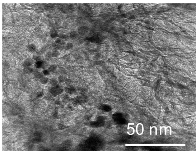
**Fig. S3** TEM image of Pd-NPs/N-C.
