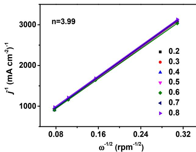
Fig. S7 Koutecky-Levich plots of Pd<sub>1</sub>/N-C at diverse potentials (0.2~0.8 V).
