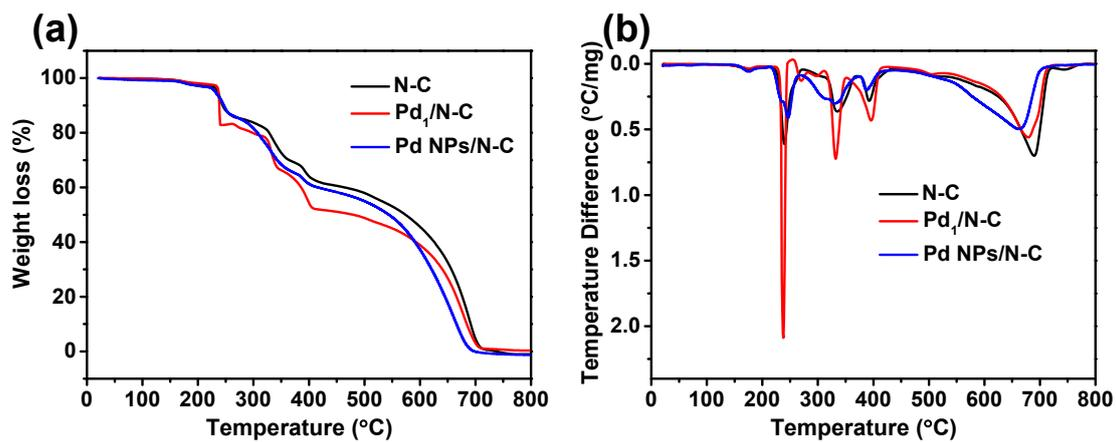
Fig. S6 TGA of N-C, Pd<sub>1</sub>/N-C and Pd-NPs/N-C.
