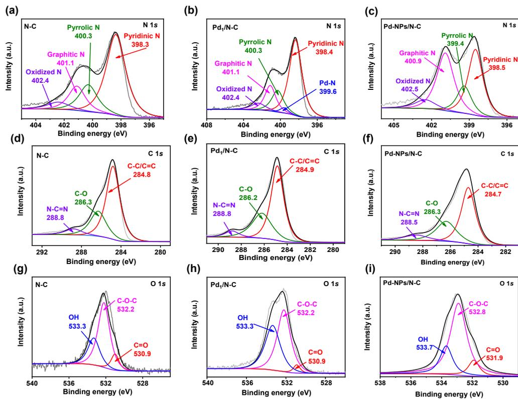
**Fig. S4** High-resolution XPS spectra of (a-c) N 1s, (d-f) C 1s, (g-i) O 1s for N-C, Pd<sub>1</sub>/N-C and Pd-NPs/N-C.
