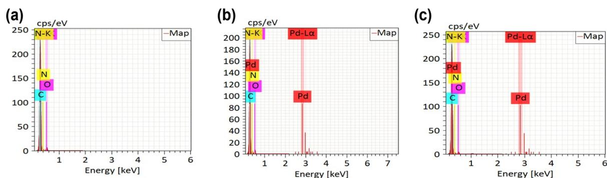
**Fig. S1** EDS spectra of (a) N-C, (b) Pd<sub>1</sub>/N-C and (c) Pd-NPs/N-C samples.
