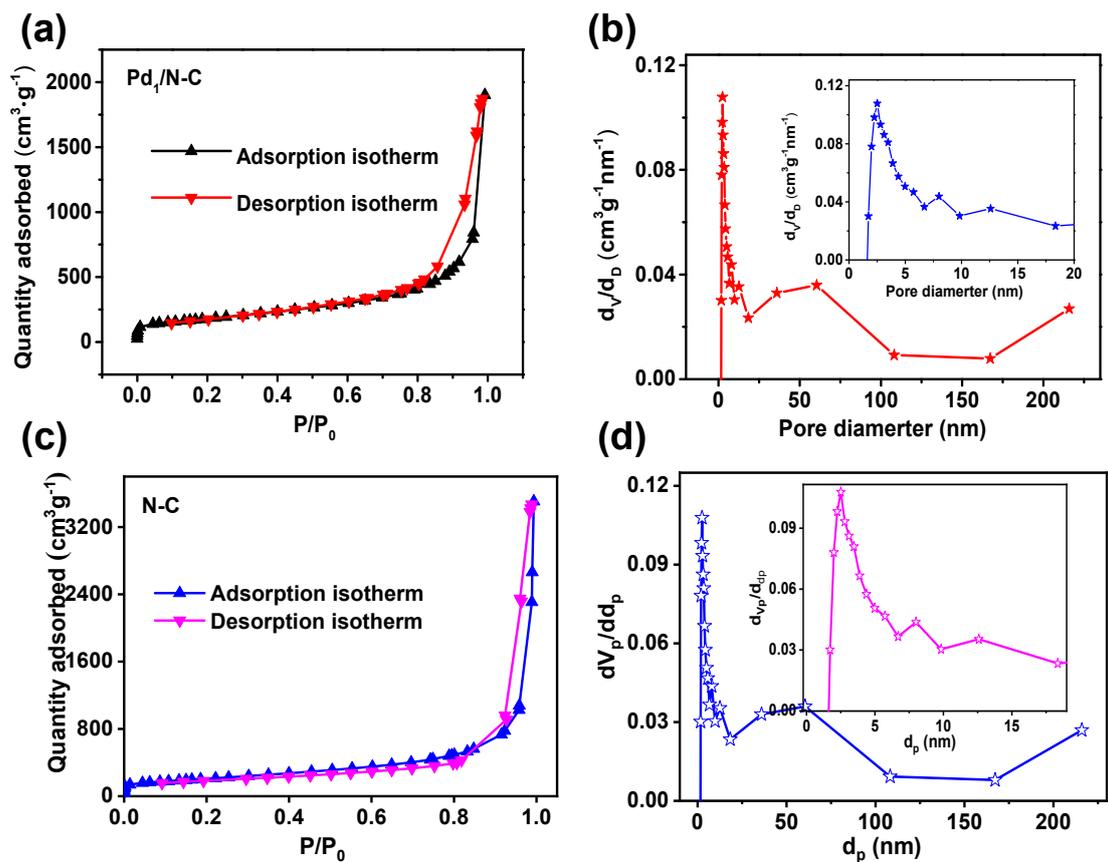
Fig. S5 (a) N<sub>2</sub> sorption isotherms, (b) and (inset) pore size distribution curves of Pd<sub>1</sub>/N-C, (c) N<sub>2</sub> adsorption-desorption isotherms of N-C, (d) and (inset) the pore size distribution curve.
