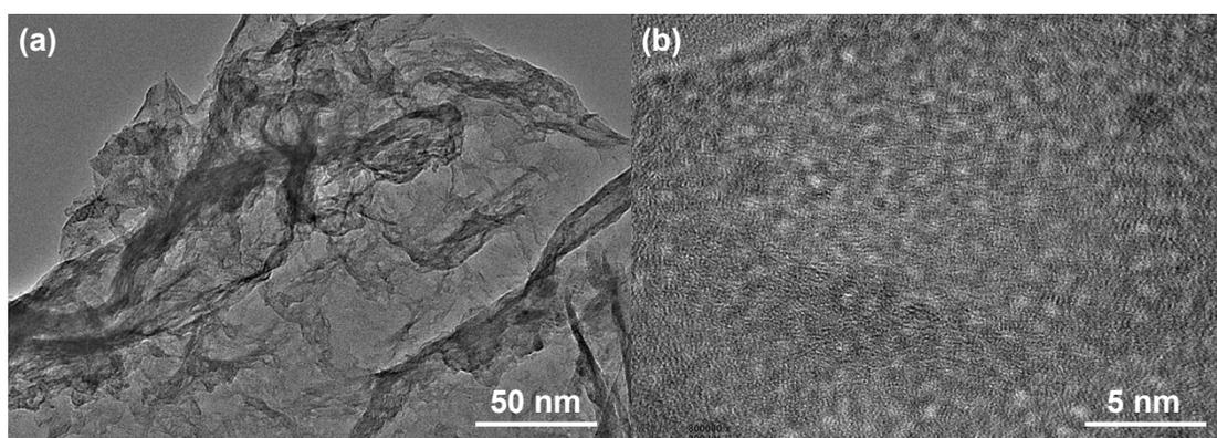
Fig. S8 TEM images of Pd<sub>1</sub>/N-C after stability tests.
