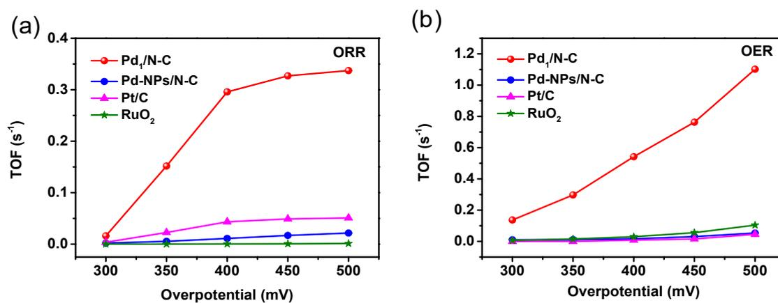
Fig. S9 TOF as a function of overpotential during (a) ORR and (b) OER.
