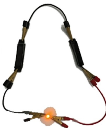
Fig. S5 The Led powered by two \text{CoWO}_4@/\text{WO}_3 -1// \text{O}_v - \text{NiMoO}_4 ASCs devices in series.
