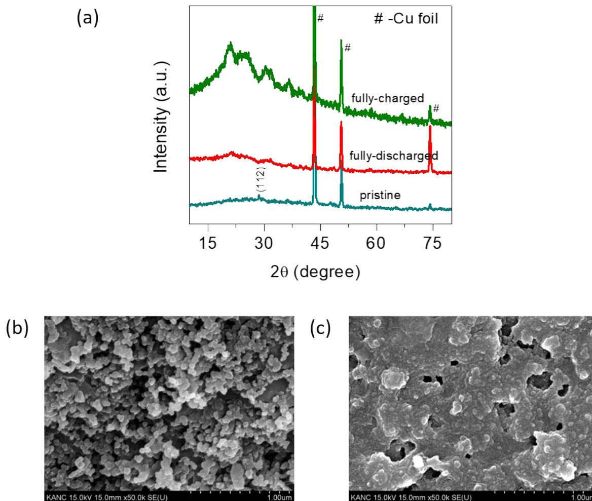
**Figure S6.** (a) Ex-situ X-ray diffraction spectra of CCTS in the fully charged to 3.0 V and fully discharged to 0.01 V states. Ex-situ SEM morphologies of the CCTS anode electrode (b) as grown CCTS electrode onto Cu-foil paper, (c) after Li-ion battery test.
