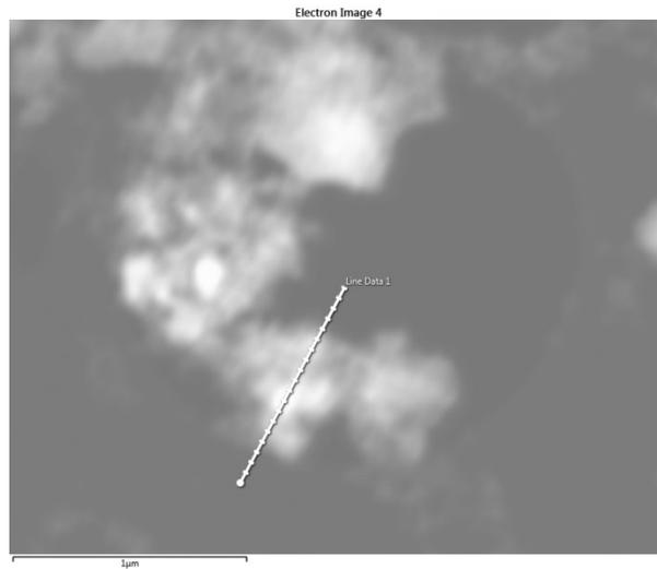
**Figure S3.** High-angle annular dark-field-scanning transmission electron microscopy (HAADF-STEM) image where the STEM elemental line scan profile was recorded (Figure 2(g) in the main text).
