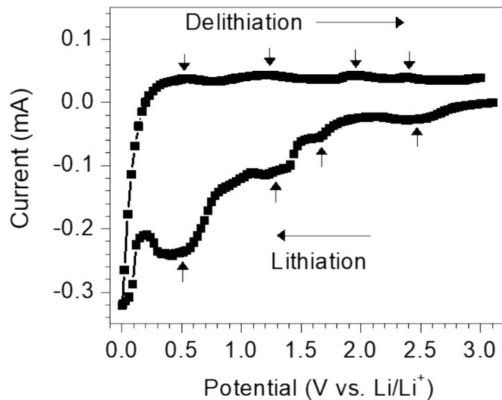
**Figure S5.** The first CV curve of the CCTS anode electrode recorded in the potential window between 0.01 and 3.0 V (vs. Li/Li<sup>+</sup>) at a scan rate of 0.1 mVs<sup>-1</sup>. The multiple cathodic and anodic peaks marked with arrows are associated with the phase transition and structural rearrangement during the initial surge of the Li<sup>2+</sup> ions.
