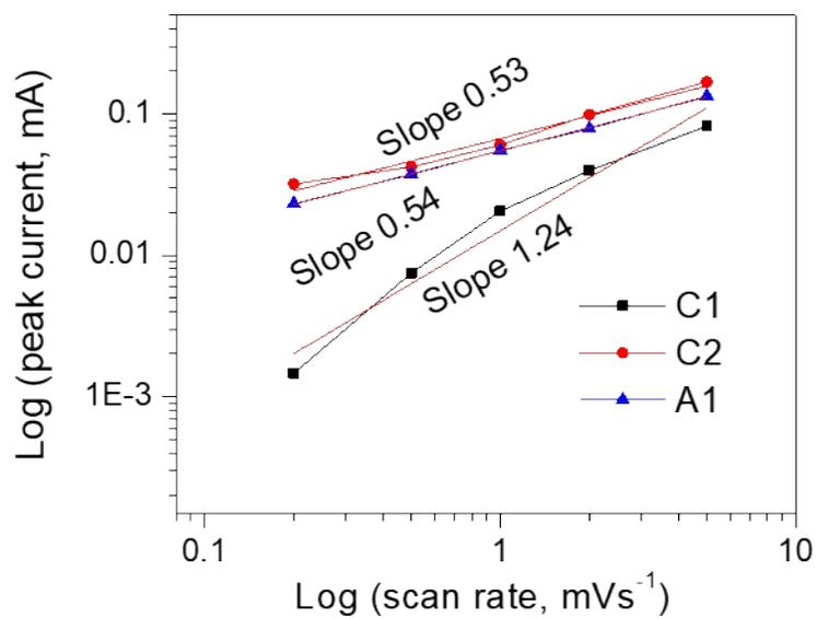
**Figure S7.** The slope of  $\log(i)$  vs  $\log(v)$  curves giving information on the mechanism exhibited by into the electrode. If the slope is less than 0.5 it is diffusion controlled and if the slope is more than 1 it is controlled by the capacitive-type storage mechanism.
