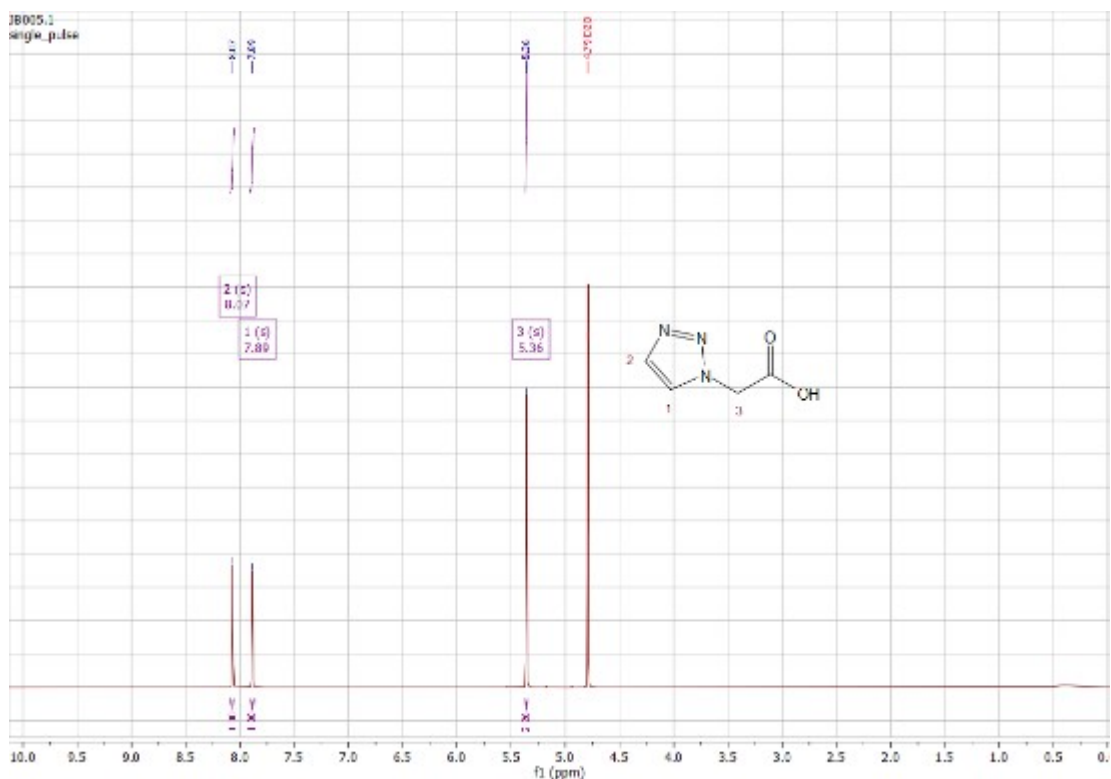
Figure S2.7. 1 H NMR spectrum of 2-(1 H -1,2,3-triazol-1-yl)acetic acid in D 2 O.
