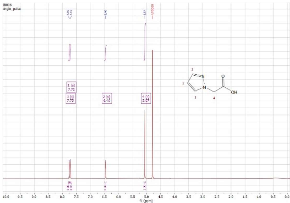
Figure S2.10. 1 H NMR spectrum of 2-(1 H -pyrazol-1-yl)acetic acid in D 2 O.
