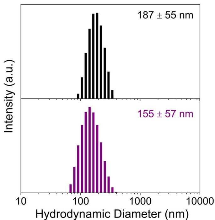
**Figure S12.** Size distributions of nanoparticles prepared by using **1/2/3/P3** (10/5/5/5 mol%) without (black bars) and with UV light (365 nm, 400 W, 5 min) irradiation (purple bars).
