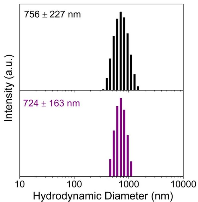
**Figure S14.** Size distributions of nanoparticles prepared by using **1/2/3/P5** (10/5/5/5 mol%) without (black bars) and with UV light (365 nm, 400 W, 5 min) irradiation (purple bars).
