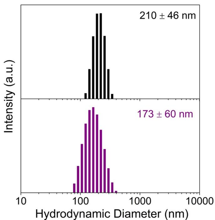
**Figure S11.** Size distributions of nanoparticles prepared by using **1/2/3/P2** (10/5/5/5 mol%) without (black bars) and with UV light (365 nm, 400 W, 5 min) irradiation (purple bars).
