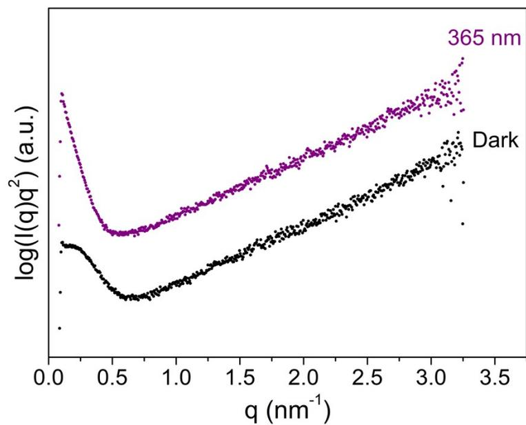
**Figure S15.** SAXS of nanoparticles prepared by using **1/2/3/P1** (10/5/5/5 mol%) without (black) and with UV light (365 nm, 400 W, 5 min) irradiation (purple).
