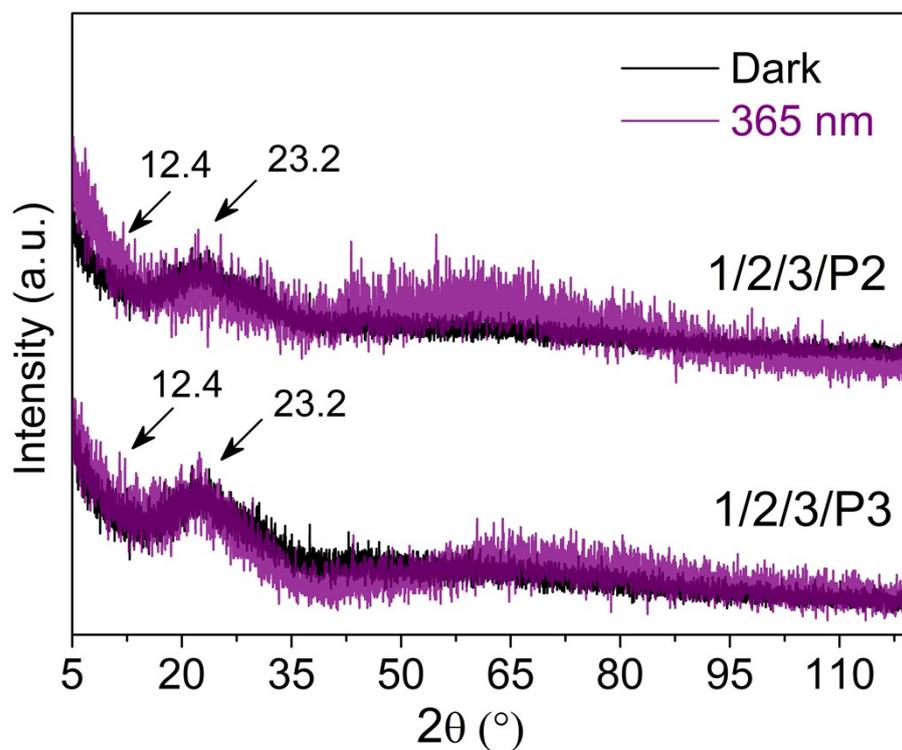
**Figure S16.** XRD patterns of nanocatalysts prepared by using **1/2/3/P2** (10/5/5/5 mol%) and **1/2/3/P3** (10/5/5/5 mol%) without or with UV light (365 nm, 400 W, 5 min) irradiation.
