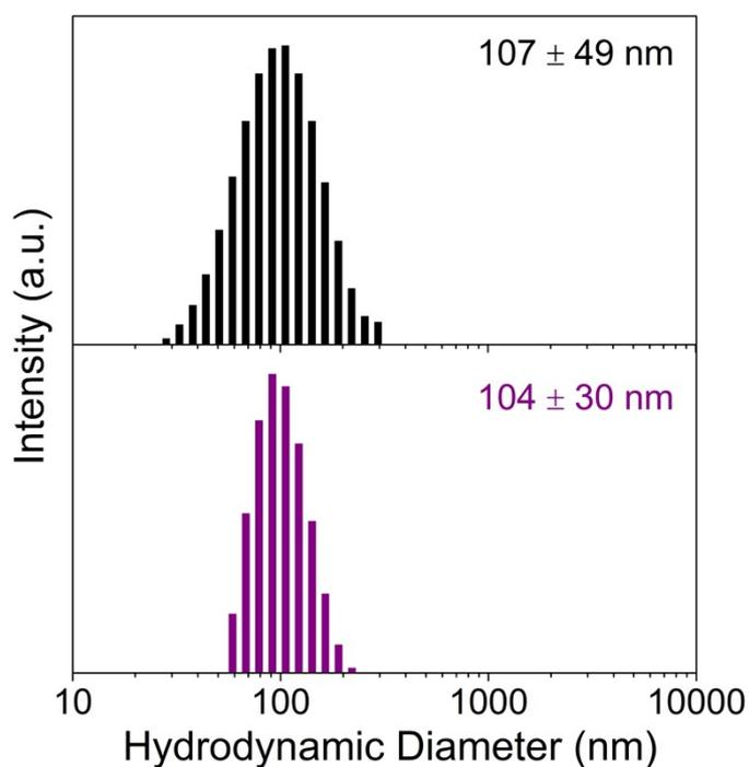
**Figure S13.** Size distributions of nanoparticles prepared by using **1/2/3/P4** (10/5/5/5 mol%) without (black bars) and with UV light (365 nm, 400 W, 5 min) irradiation (purple bars).
