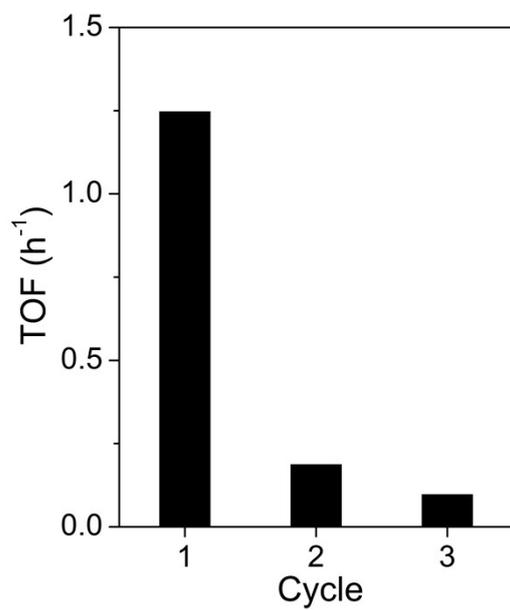
**Figure S17.** Recycling of the nanocatalyst prepared by using **1/2/3/P1** (10/5/5/5 mol%) with UV light (365 nm, 400 W, 5 min) irradiation.
