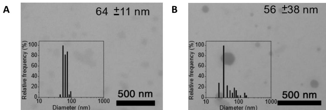
**Figure S8.** Typical TEM images of nanoparticle catalysts prepared by using **1/2/3/P1** (10/5/5/5 mol%, effective constituent ratio relative to BnOH) (A) without and (B) with UV light (365 nm, 400 W, 5 min) irradiation.
