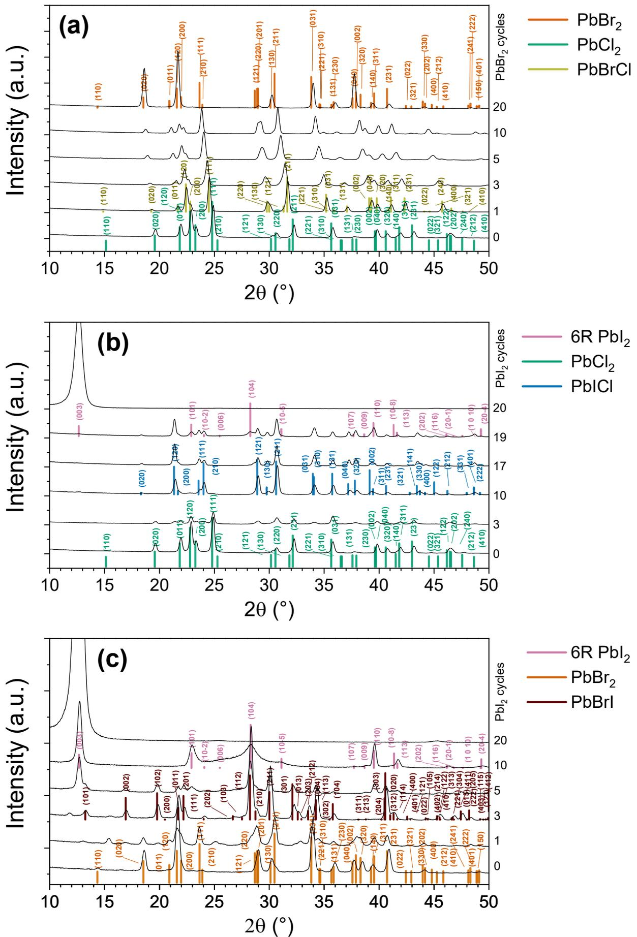
**Figure S21.** XRD patterns of (a)  $\text{PbBr}_x\text{Cl}_{2-x}$ , (b)  $\text{Pb}_x\text{Cl}_{2-x}$  and  $\text{PbBr}_x\text{I}_{2-x}$  films. Relevant XRD reference patterns, including  $\text{PbBr}_2$  (ICDD 31-679),  $\text{PbCl}_2$  (ICDD 26-1150),  $\text{PbBrCl}$  (ICDD 24-1088),  $6\text{R PbI}_2$  (COD 9009142),  $\text{PbI}_2$  (ICDD 43-949) and  $\text{PbBrI}$  (ICSD 22138) are shown. All films were deposited at 75 °C.
