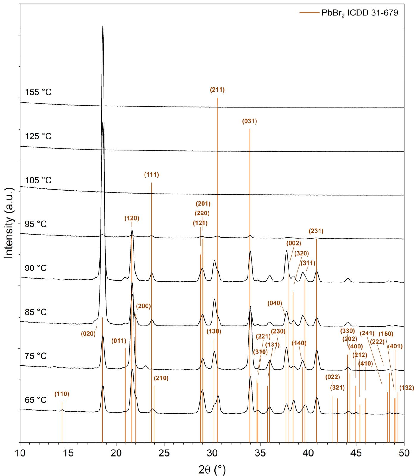
**Figure S14.** XRD patterns of PbBr<sub>2</sub> films deposited with Pb(btsa)<sub>2</sub> and TiBr<sub>4</sub> at different temperatures. The films were deposited with 1000 cycles. The pulse durations were 1.0 s and 1.5 s long for Pb(btsa)<sub>2</sub> and TiBr<sub>4</sub> respectively and were separated by 1.0 s long purges.
