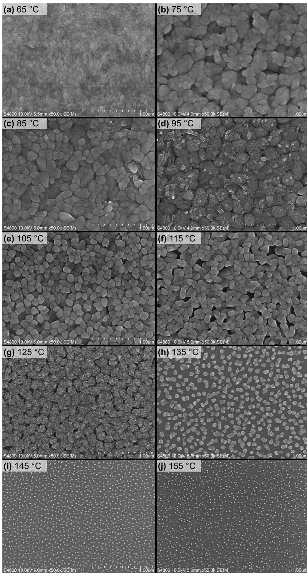
**Figure S11.** Top down FESEM images of  $\text{PbCl}_2$  films deposited at different temperatures. The films were deposited with 600 cycles of 1.5 s  $\text{Pb}(\text{btsa})_2$  pulse, 0.8 s  $\text{GaCl}_3$  pulse and 3.0 s purge durations.
