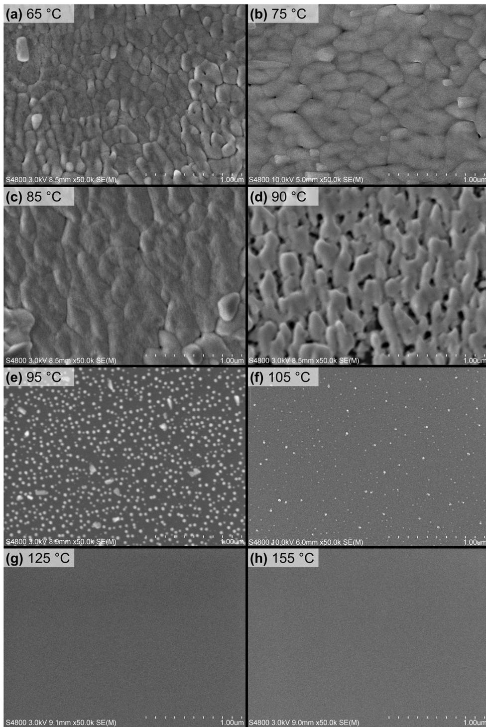
**Figure S15.** Top down FESEM images of  $\text{PbBr}_2$  films deposited at different temperatures. The films were deposited with 1000 cycles of 1.0 s  $\text{Pb}(\text{btsa})_2$  pulse, 1.5 s  $\text{TiBr}_4$  pulse and 1.0 s purge durations.
