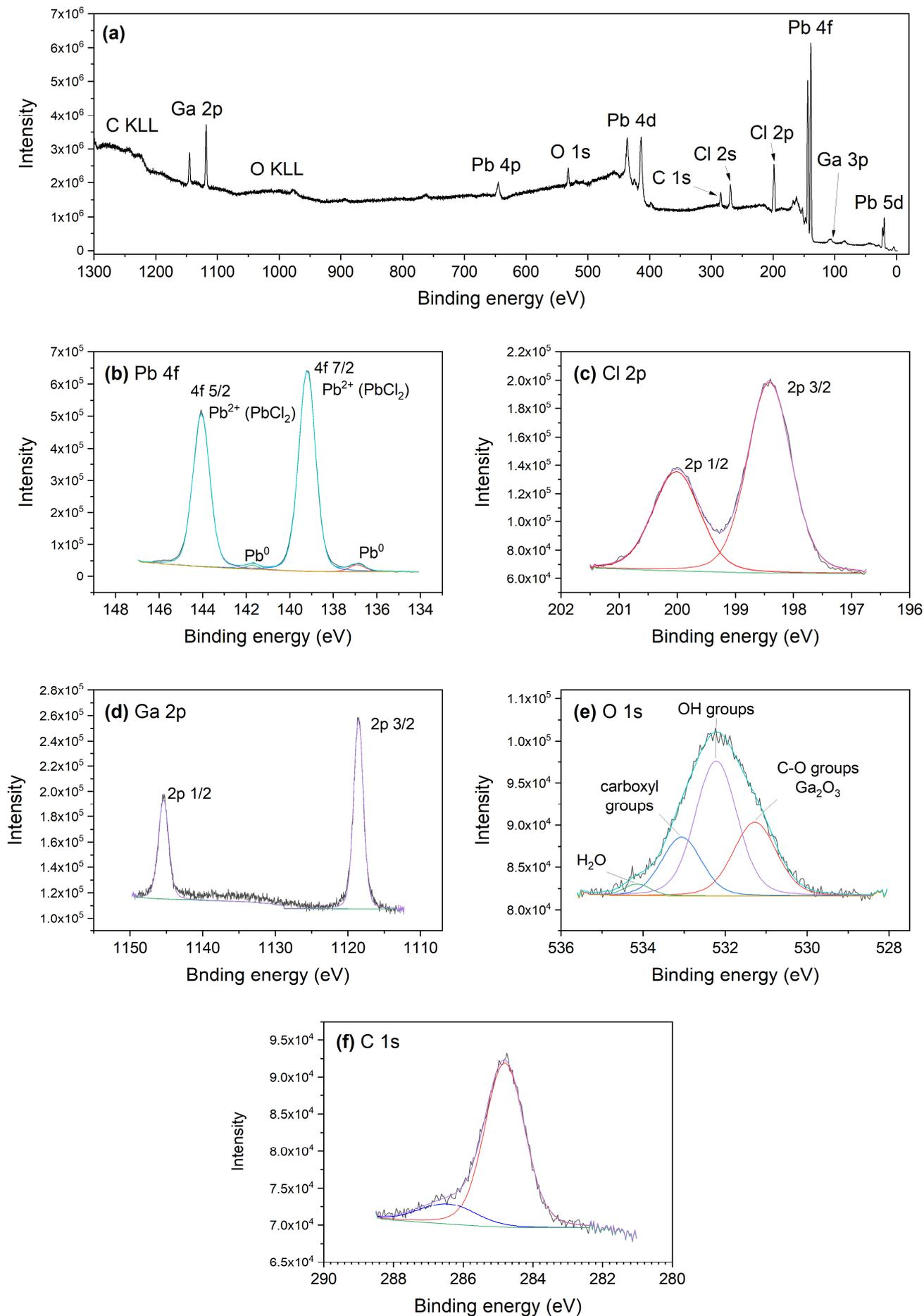
**Figure S10.** (a) XPS spectra of a  $\text{PbCl}_2$  film as well as high resolution spectra of Pb 4f (b), Cl 2p (c), Ga 2p (d), O 1s (e) and C 1s (f). The  $\text{PbCl}_2$  film was deposited at 85 °C with 600 cycles of 1.5 s and 0.8 s long pulses of  $\text{Pb}(\text{btsa})_2$  and  $\text{GaCl}_3$  respectively, separated by 3.0 s long purges.
