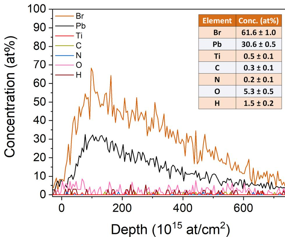
**Figure S16.** Elemental depth profile and composition of a  $\text{PbBr}_2$  film as analysed by ToF-ERDA. The  $\text{PbBr}_2$  film was deposited at 75 °C with 1000 cycles of 1.0 s  $\text{Pb}(\text{btsa})_2$  pulse, 1.5 s  $\text{TiBr}_4$  pulse and 1.0 s purge durations.
