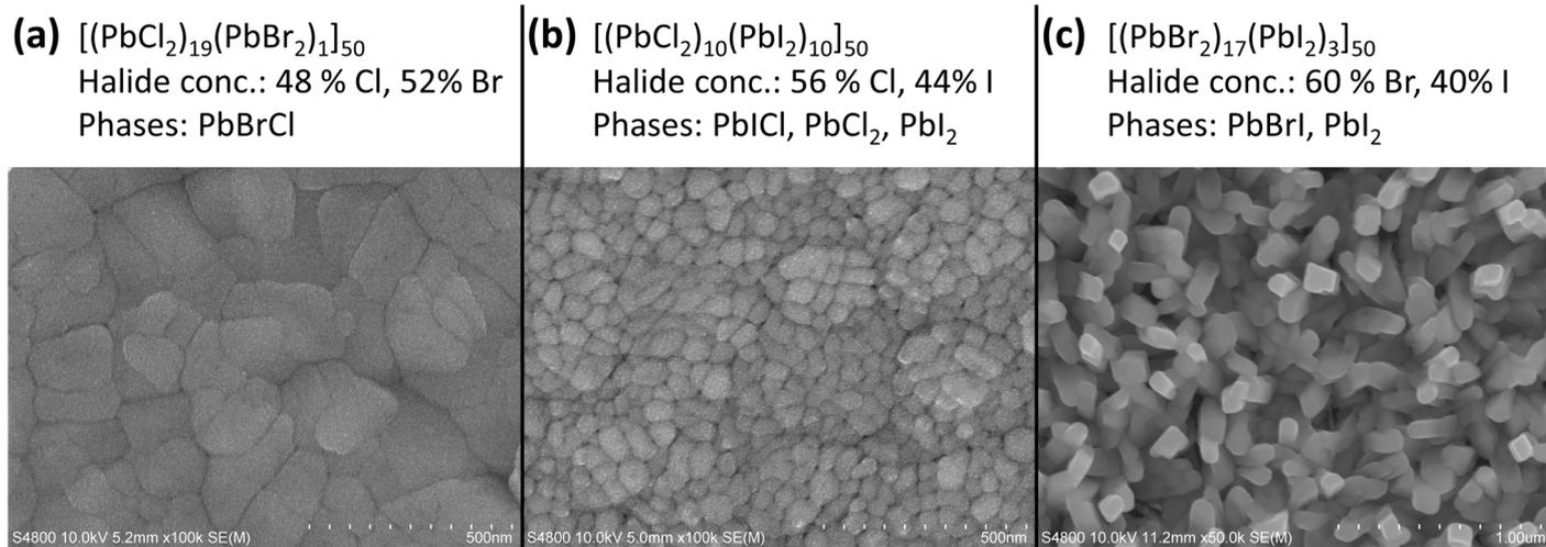
**Figure S22.** FESEM images of selected mixed lead halide films deposited at 75 °C.
