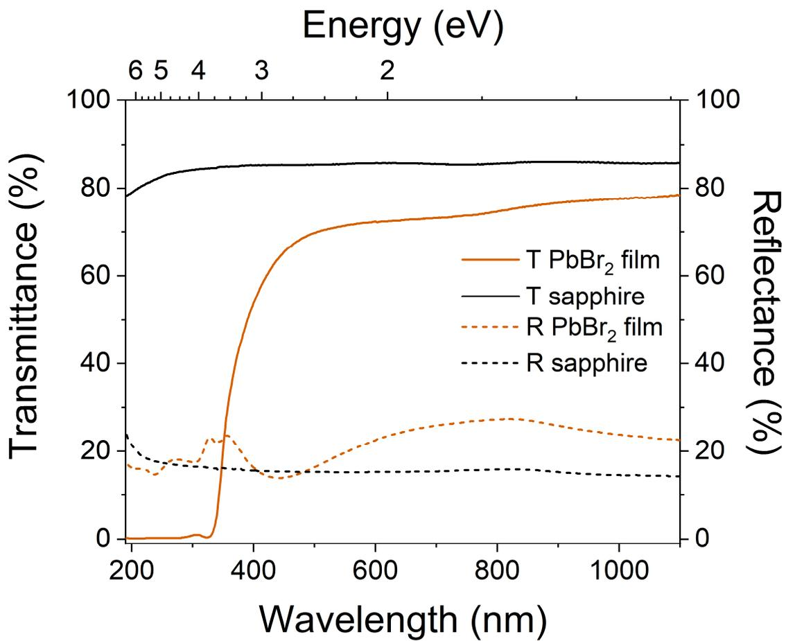
**Figure S19.** Transmittance and reflectance of a  $\text{PbBr}_2$  film deposited at  $75^\circ\text{C}$ , with 1000 cycles of 1.0 s  $\text{Pb}(\text{btsa})_2$ , 1.5 s  $\text{TiBr}_4$  pulse and 1.0 s purge durations. An evaporated aluminium mirror served as a reference for reflectance measurements.
