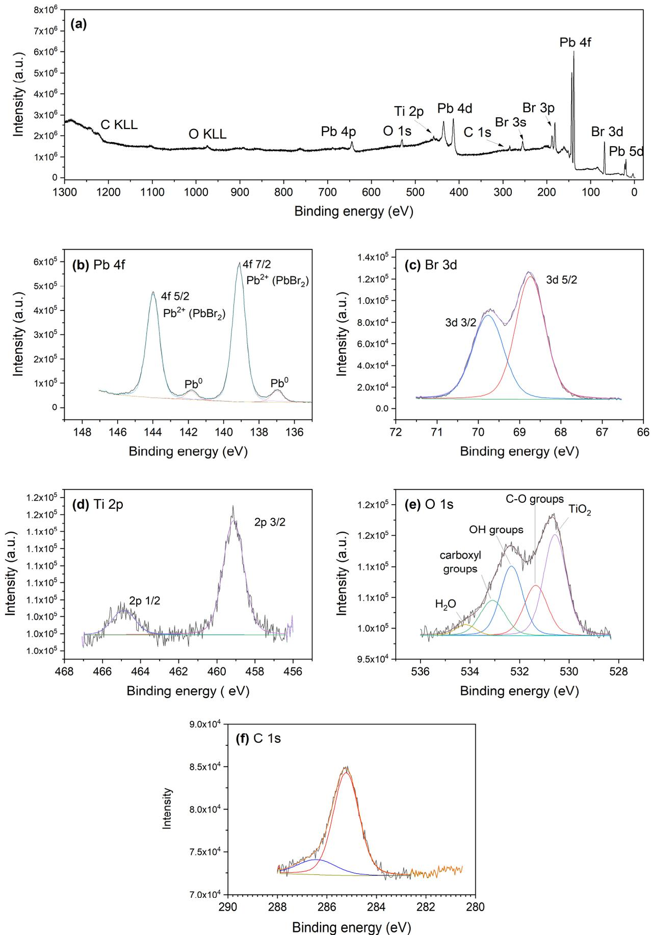
**Figure S17.** (a) XPS spectra of a PbBr<sub>2</sub> film as well as high resolution spectra of Pb 4f (b), Cl 2p (c), Ti 2p (d), O 1s (e) and C 1s (f). The PbBr<sub>2</sub> film was deposited at 75 °C with 1000 cycles of 1.0 s Pb(btsa)<sub>2</sub> pulse, 1.5 s TiBr<sub>4</sub> pulse and 1.0 s purge durations.
