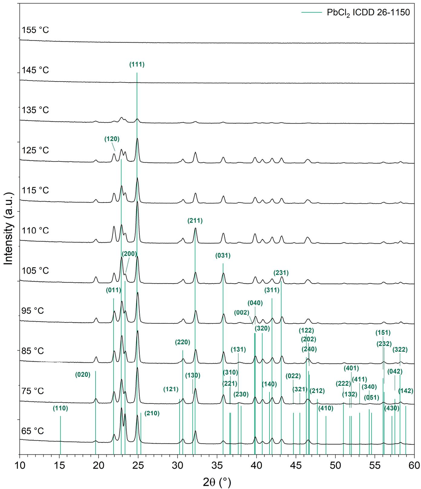
**Figure S7.** XRD patterns of  $\text{PbCl}_2$  films deposited with  $\text{Pb}(\text{btsa})_2$  and  $\text{GaCl}_3$  at different temperatures. The films were deposited with 600 cycles of 1.5 s  $\text{Pb}(\text{btsa})_2$  pulse, 0.8 s  $\text{GaCl}_3$  pulse and 3.0 s purge durations.
