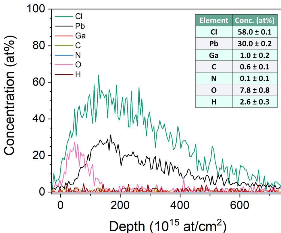
**Figure S8.** Elemental depth profile and composition of a  $\text{PbCl}_2$  film as analysed by ToF-ERDA. The  $\text{PbCl}_2$  film was deposited at 85 °C with 600 cycles of 1.5 s and 0.8 s long pulses of  $\text{Pb}(\text{btsa})_2$  and  $\text{GaCl}_3$  respectively, separated by 3.0 s long purges.
