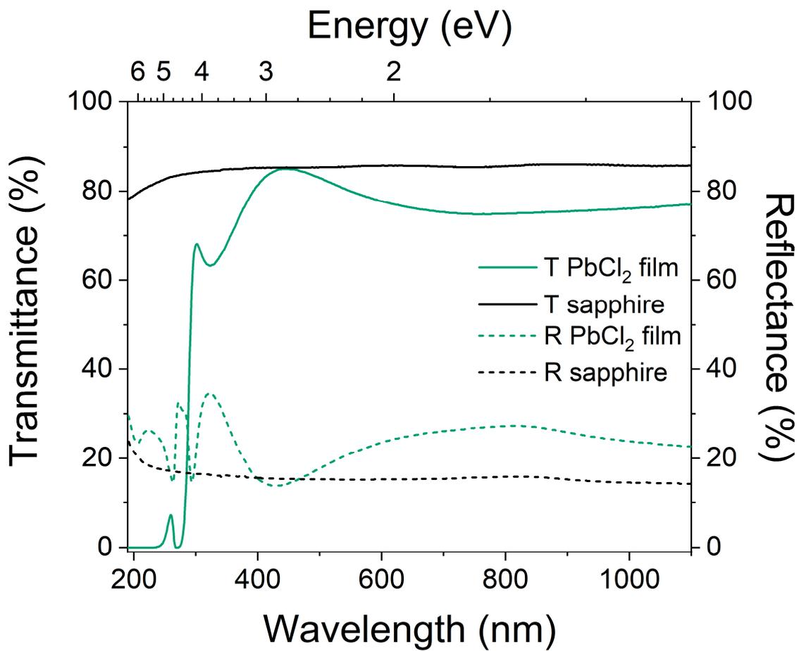
**Figure S12.** Transmittance and reflectance of a PbCl<sub>2</sub> film deposited at 85 °C, with 600 cycles of 1.5 s Pb(btsa)<sub>2</sub>, 0.8 s GaCl<sub>3</sub> pulse and 3.0 s purge durations. An evaporated aluminium mirror served as a reference for reflectance measurements.
