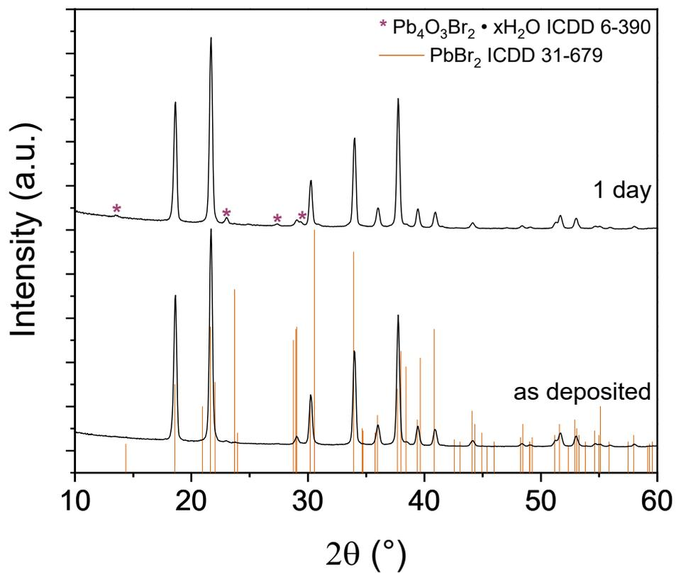
**Figure S18.** XRD pattern of a  $\text{PbBr}_2$  film as deposited and after storage in ambient air for 1 day. The film was deposited at 75 °C with 1000 cycles of 1.0 s  $\text{Pb}(\text{btsa})_2$  pulse, 1.5 s  $\text{TiBr}_4$  pulse and 1.0 s purge durations. The as deposited sample is still exposed to air during the transfer between the ALD reactor and diffractometer.
