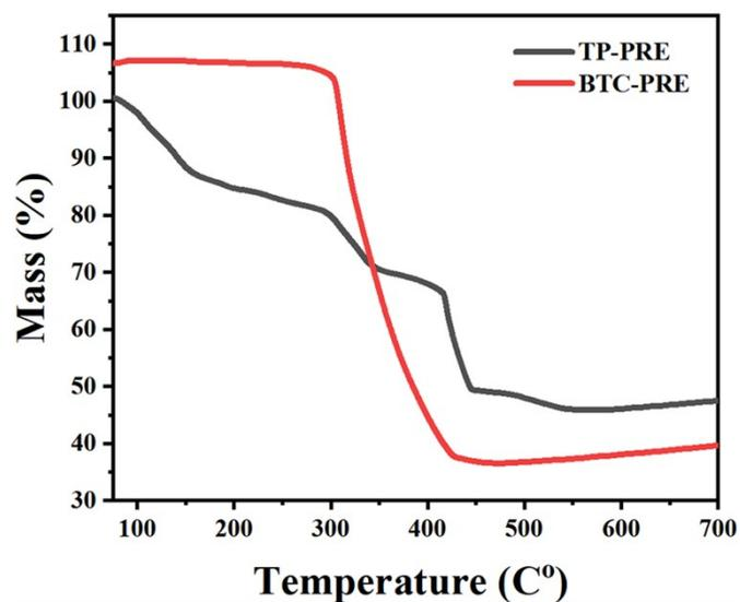
Figure S2 The TGA curves of TP-PRE and BTC-PRE.
