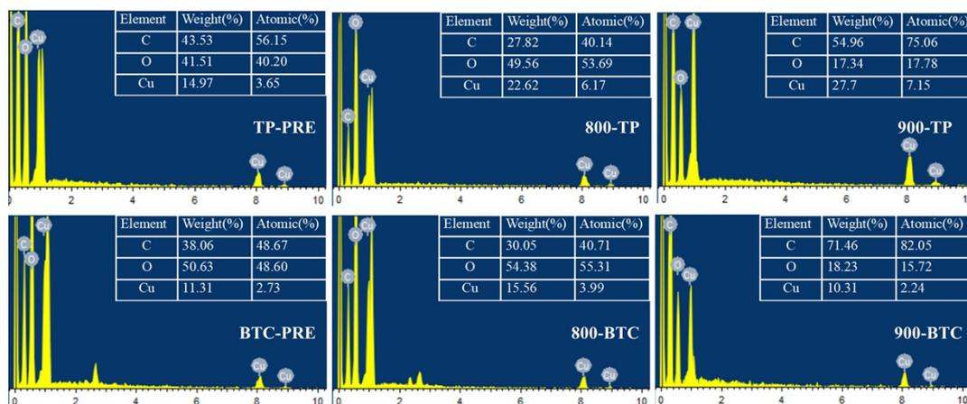
Figure S3 EDS analysis of TP-PRE, 800-TP, 900-TP, BTC-PRE, 800-BTC, 900-BTC
