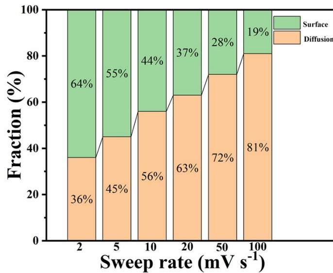
**Figure S14** Normalized contribution ratio of surface/diffusion-controlled currents at various scan rates for 900-BTC
