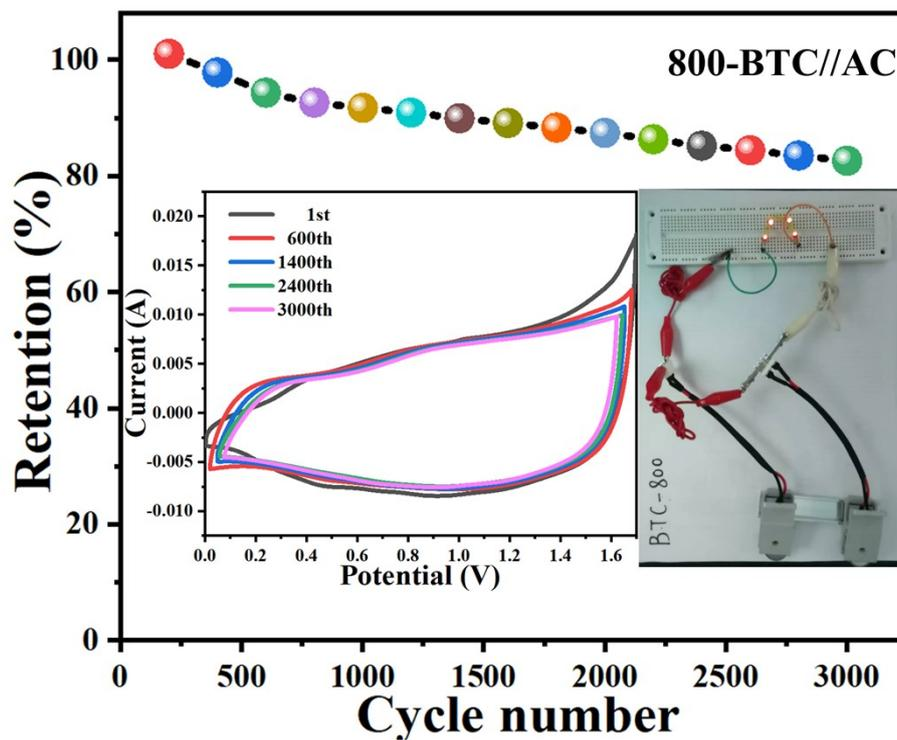
Figure S19 The endurance tests of the 800-BTC//AC device for 3000 cycles at  $30 \text{ mV s}^{-1}$ . Inset: CV curves at different cycles.
