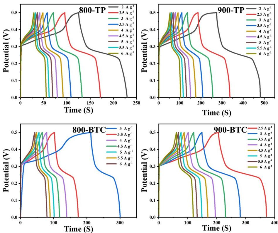
Figure S12 CP curves of 800-TP, 900-TP, 800-BTC and 900-BTC electrodes at different scan rates
