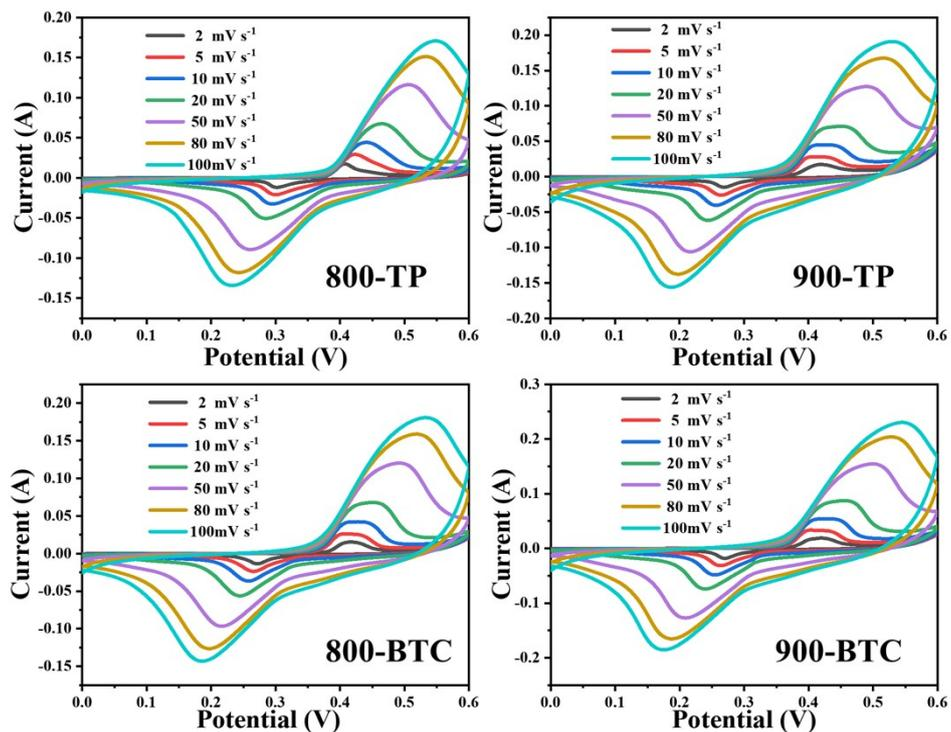
Figure S11 CV curves of 800-TP, 900-TP, 800-BTC and 900-BTC electrodes at different scan rates
