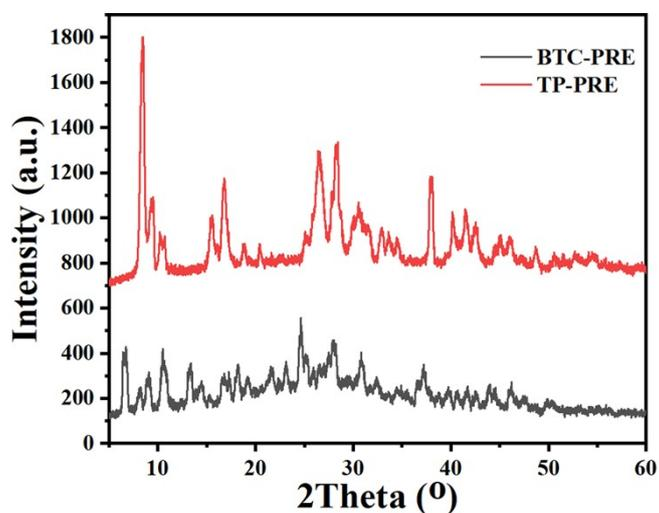
**Figure S1** Comparison of XRD patterns of BTC-PRE and TP-PRE
