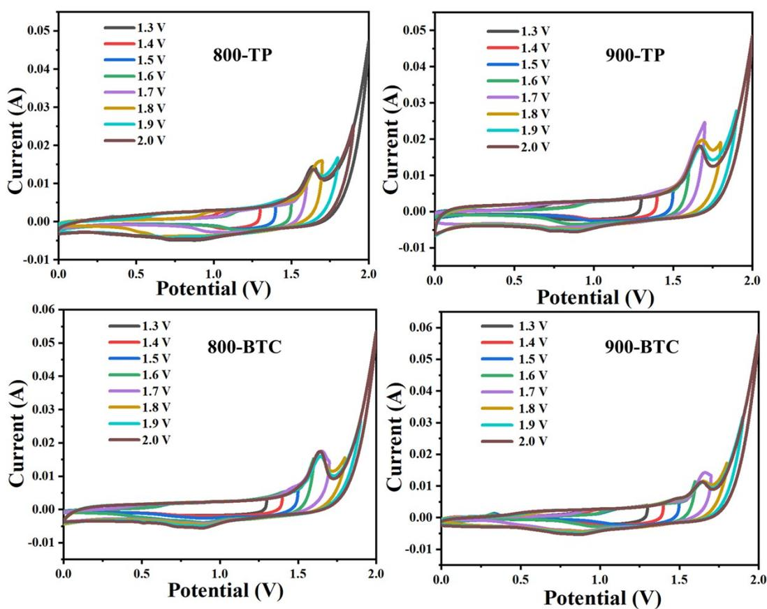
**Figure S16** Polarization curves of 800-TP//AC, 900-TP//AC, 800-BTC//AC and 900-BTC//AC, respectively.
