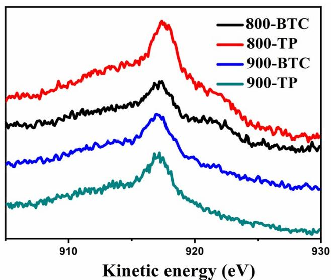
Figure S4 Auger energy spectra of 900-BTC, 900-TP, 800-BTC and 800-TP, respectively.
