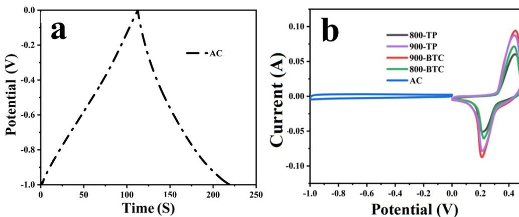
**Figure S15** (a) CP curves of AC at a current density of  $1 \text{ A g}^{-1}$  in  $6 \text{ mol L}^{-1} \text{ KOH}$
