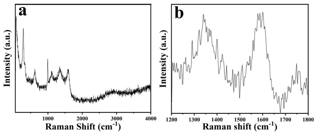
**Figure S10** (a) The Raman curve of BTC-900 from 50  $\text{cm}^{-1}$  to 4000  $\text{cm}^{-1}$  Raman shift
