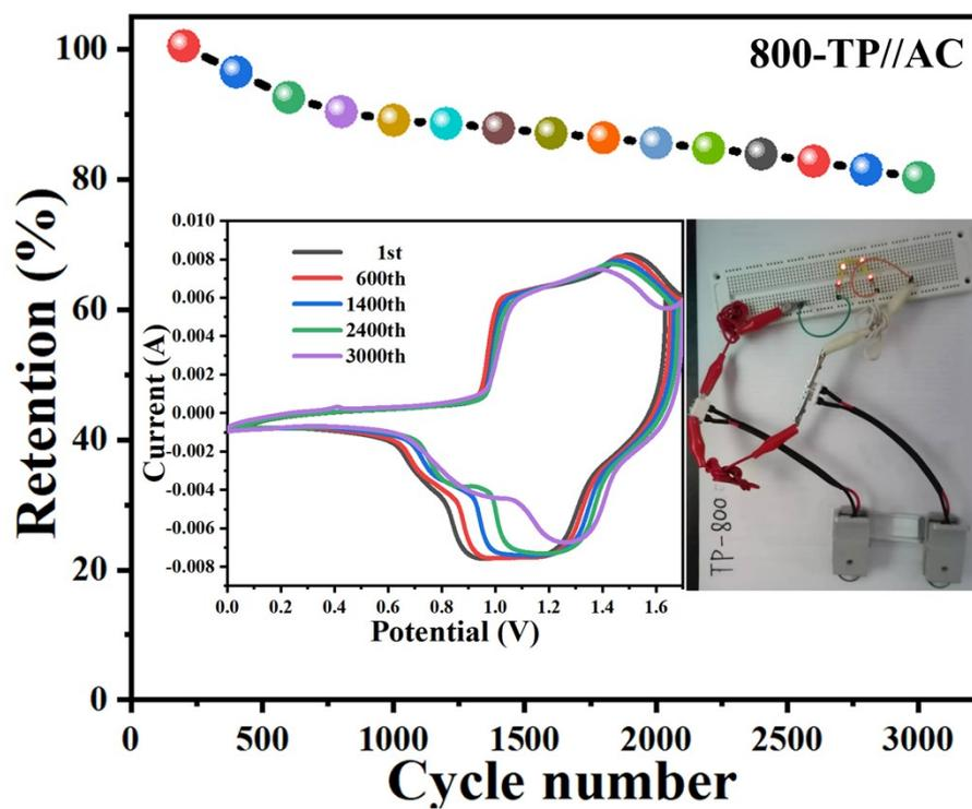
**Figure S21** The endurance tests of the 800-TP//AC device for 3000 cycles at  $30 \text{ mV s}^{-1}$ . Inset: CV curves at different cycles.
