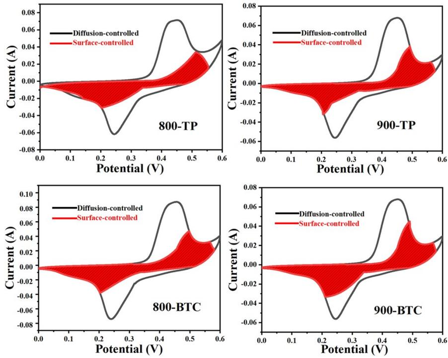
**Figure S13** Voltammetric response for the as-prepared calcined sample electrodes at a sweep rate of  $20 \text{ mV s}^{-1}$
