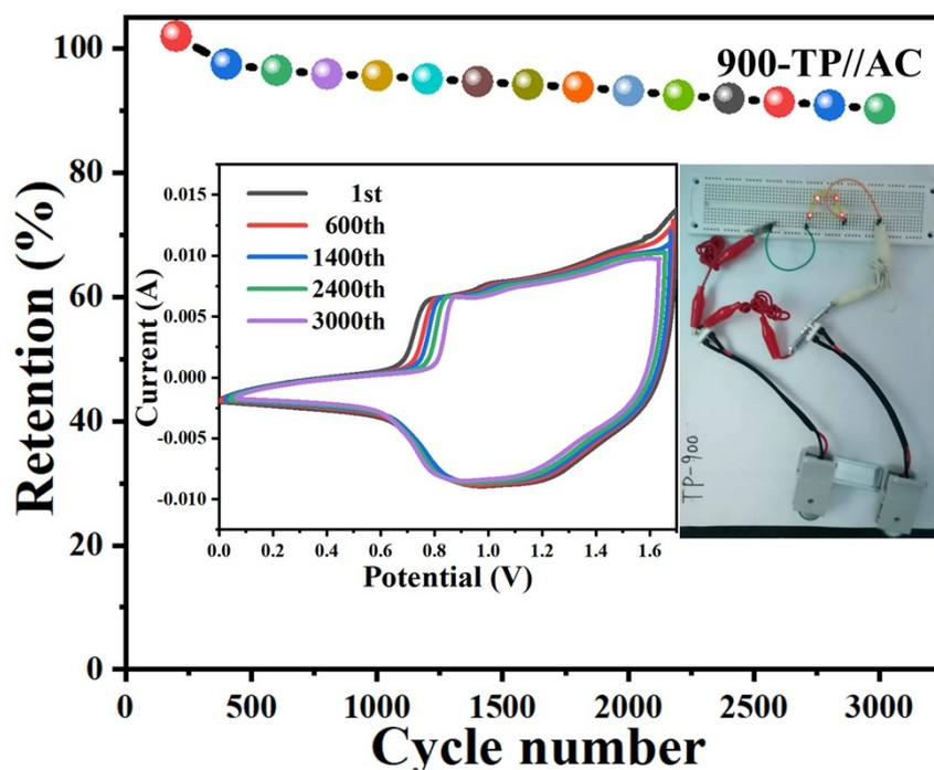
Figure S20 The endurance tests of the 900-TP//AC device for 3000 cycles at  $30 \text{ mV s}^{-1}$ . Inset: CV curves at different cycles.
