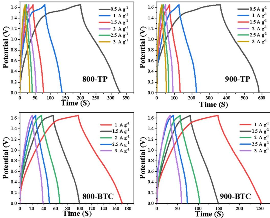
Figure S18 CP curves of 800-TP//AC, 900-TP//AC, 800-BTC//AC and 900-BTC//AC
