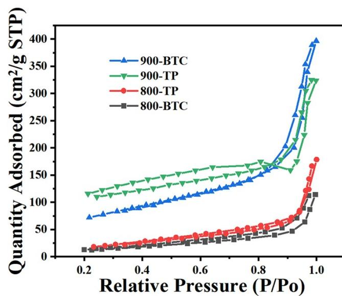
**Figure S5** Nitrogen adsorption-desorption isotherm and pore-size distribution of calcined samples
