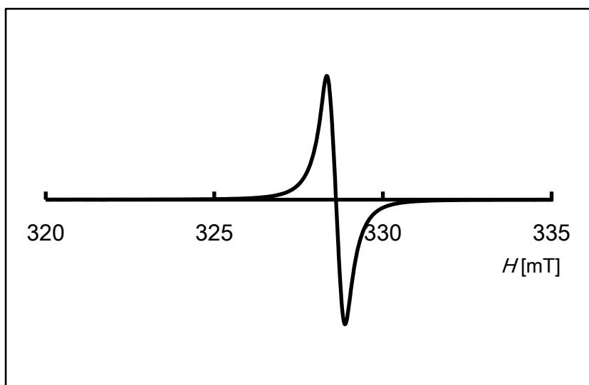
**Fig. S8** ESR spectrum of **[5b]**SbCl<sub>6</sub> in the solid state at -150 °C.
