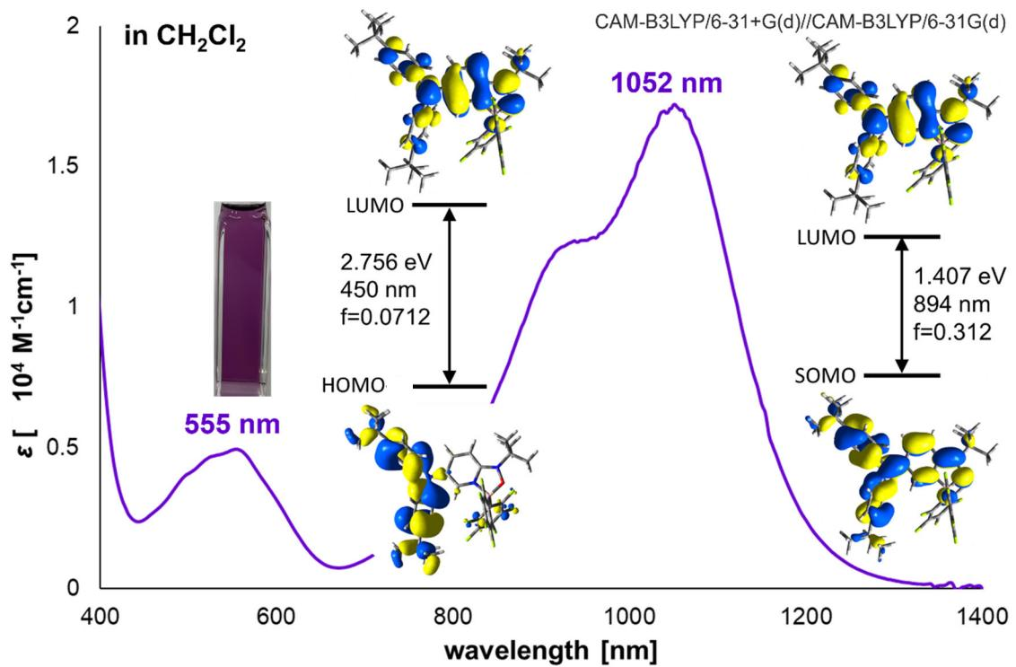
**Fig. S20** UV-vis-NIR spectrum of **[5a]SbCl<sub>6</sub>** in  $\text{CH}_2\text{Cl}_2$  and TD-DFT assignments for the longest and second longest absorption bands.
