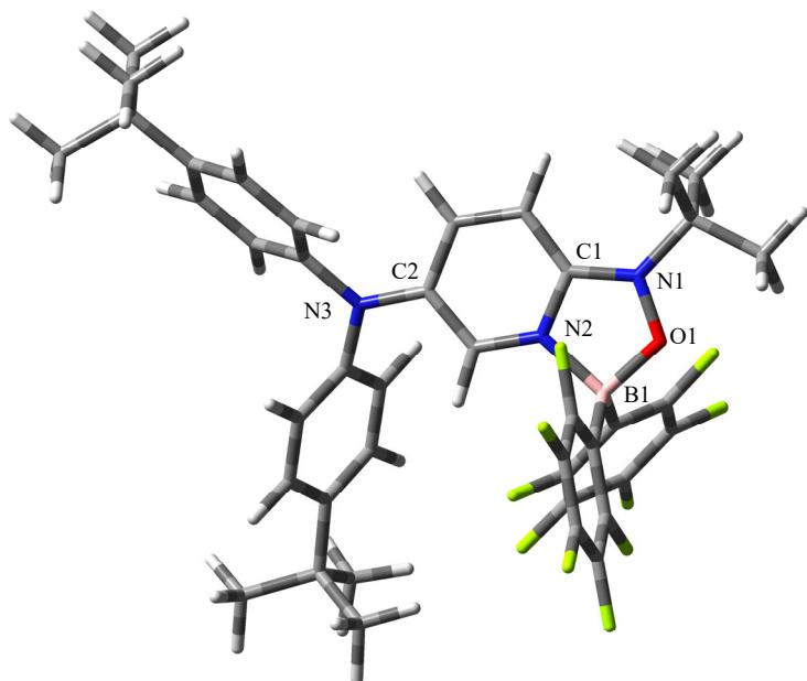
**Fig. S11** DFT-optimized structure of **5a**. Selected bond lengths (Å): N1-O1 1.338, C1-N1 1.341, O1-B1 1.514, N2-B1 1.605, C2-N3 1.363.
