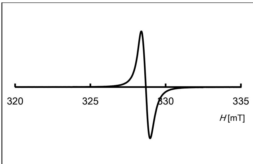
**Fig. S5** ESR spectrum of **[5a]**SbCl<sub>6</sub> in the solid state at 25 °C.
